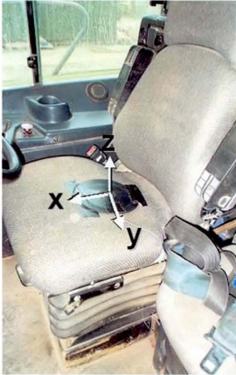
Figure 3.8 Typical location of mounting for the seat surface accelerometer, highlighting the vibration axes measured.
