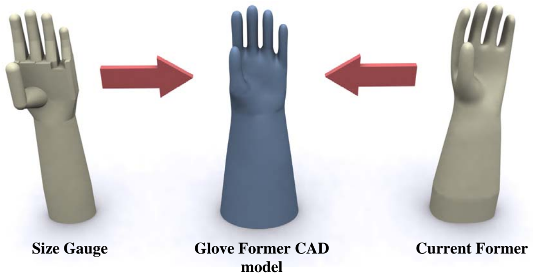
Figure 6.15 – Integrating current glove former detail and size gauge 3D shape into the glove former CAD model.
