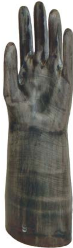
Figure 6.19 – Size 4 resin cast of a prototype former
