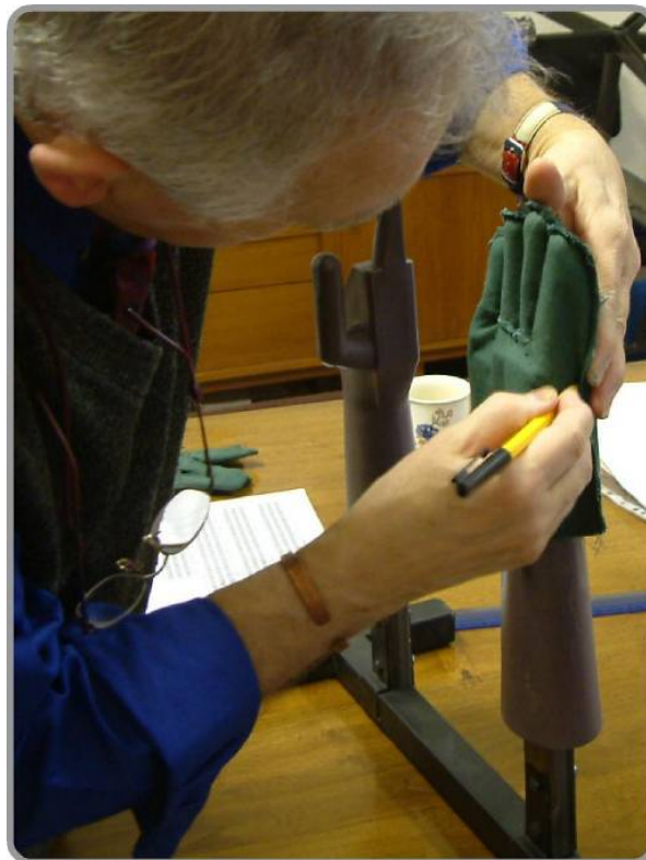
Figure 5.46 – Pattern designer using size gauge for fit analysis
