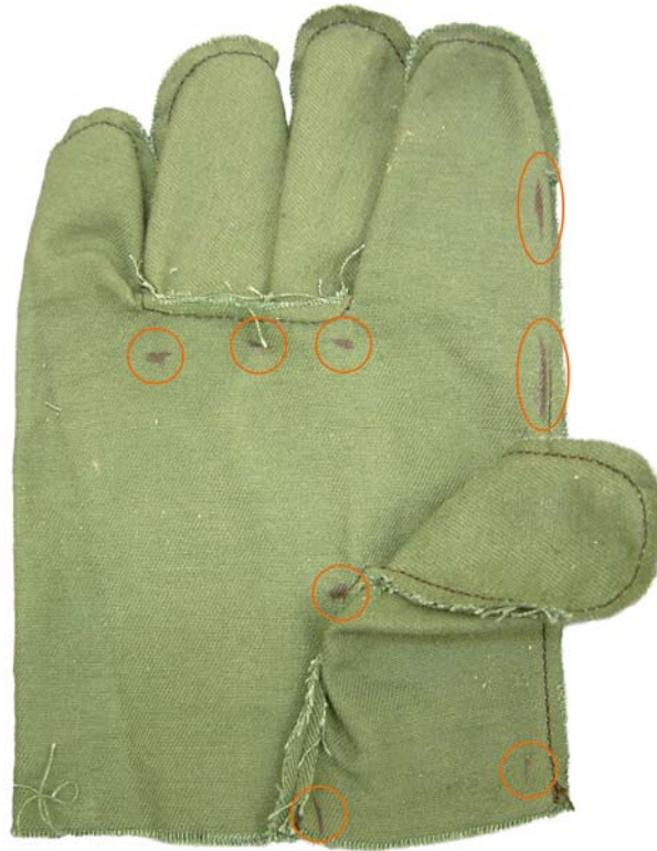
Figure 5.64 – Fit errors identified on glove following analysis with size gauge
