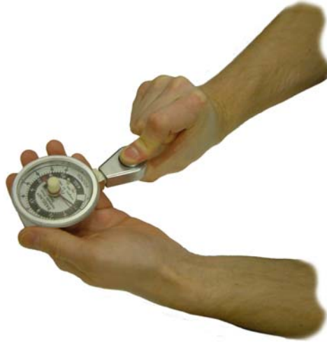
Figure 5.52 – Pinch strength being recorded
