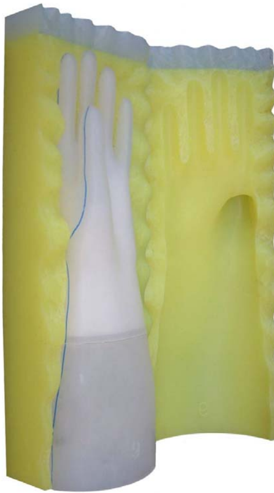
Figure 6.18 – The RP model in the silicon tooling
