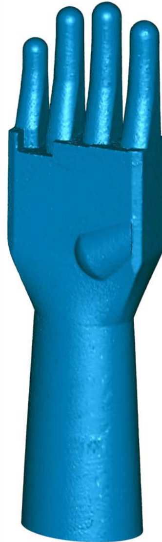
Figure 7.8 – Completed surface model from point cloud data
