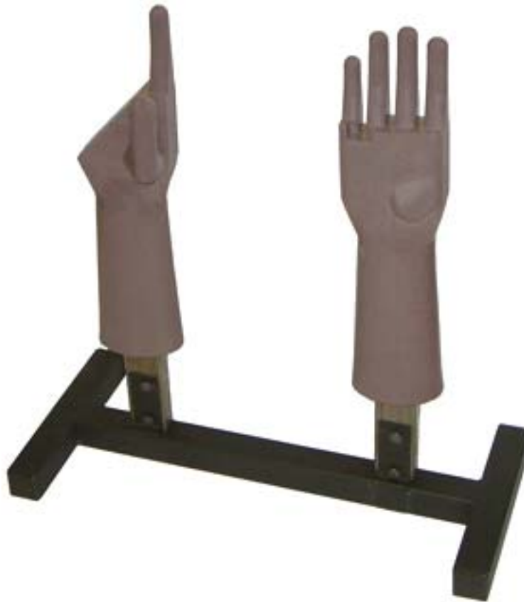
Figure 5.26 – A size 3 right- handed size gauge (manikin)
