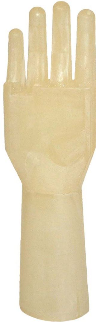
Figure 5.21 – RP model of size 3 hand model
