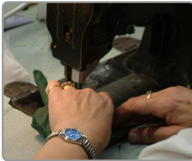
Figure 5.35 – Seamstress stitching glove pieces together to form glove
