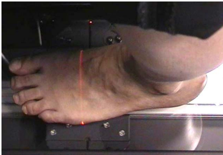
Figure 2.4 – A foot being scanned using the INFOOT 3D foot scanner from Shoemaster (Shoemaster, 2003).
