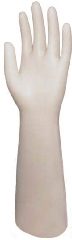
Figure 6.1 – Ceramic former used in glove dip moulding
