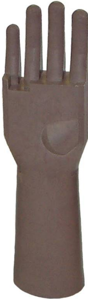
Figure 5.23 – Resin cast from silicon tool
