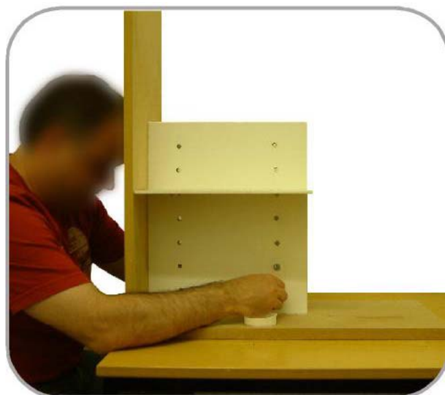
Figure 5.56 – Subject performing nut and bolt assembly test
