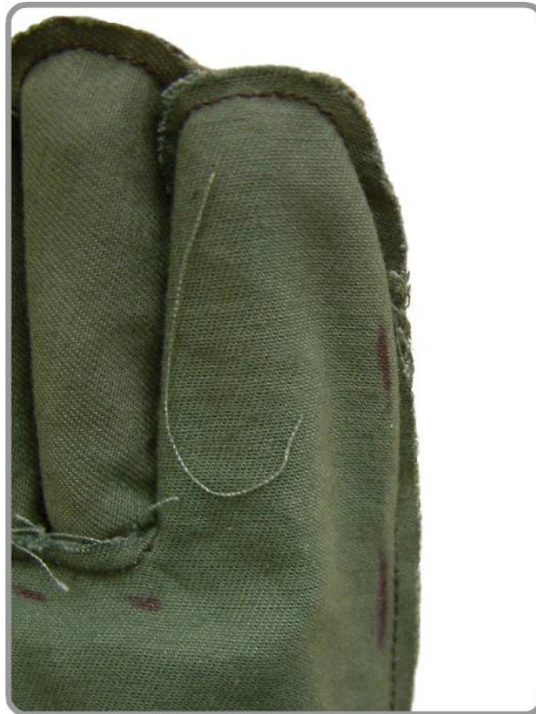
Figure 5.47 – Markings on glove to identify fit errors
