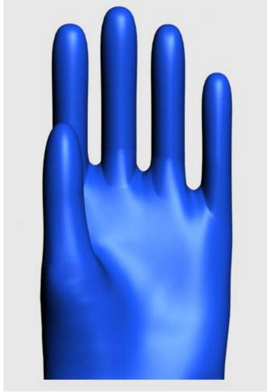
Figure 6.13 – Digits and palm surfaces blended together to create the completed hand shape.
