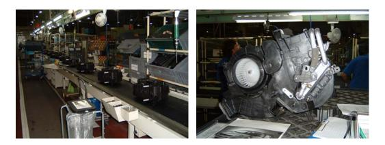
Figure 7.8: (a) Heater Assembly Line 3 and (b) Heater Unit
