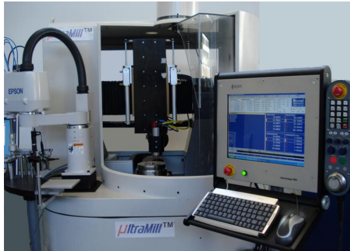
Fig. 7.5 5-axis micro milling machine tool
