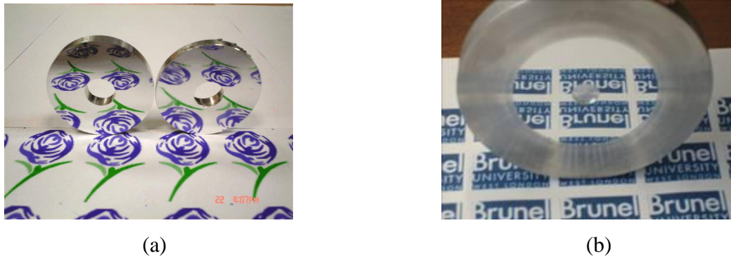
Fig. 7.2 Machined mirror surfaces: (a) the mirror surface machined on Machine A, (b) the mirror surface machined on Machine B.
