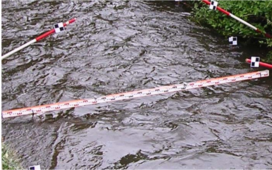
Figure 5.15: Survey staff positioned close to the water surface
