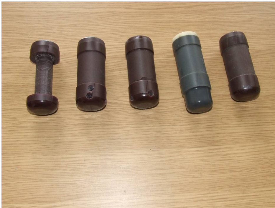
Figure 21: The different projectiles used to investigate impact characteristics with the instrument simulated skull
