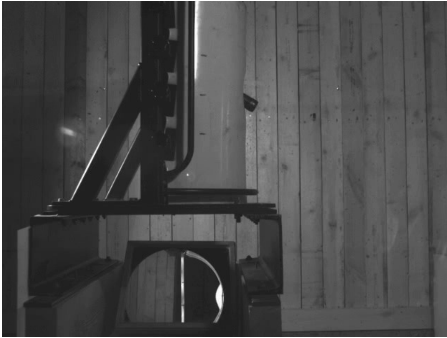
Figure 213: 4 Hole 2 Row L21A1 against BABT rig (3) Time = 4.9ms
