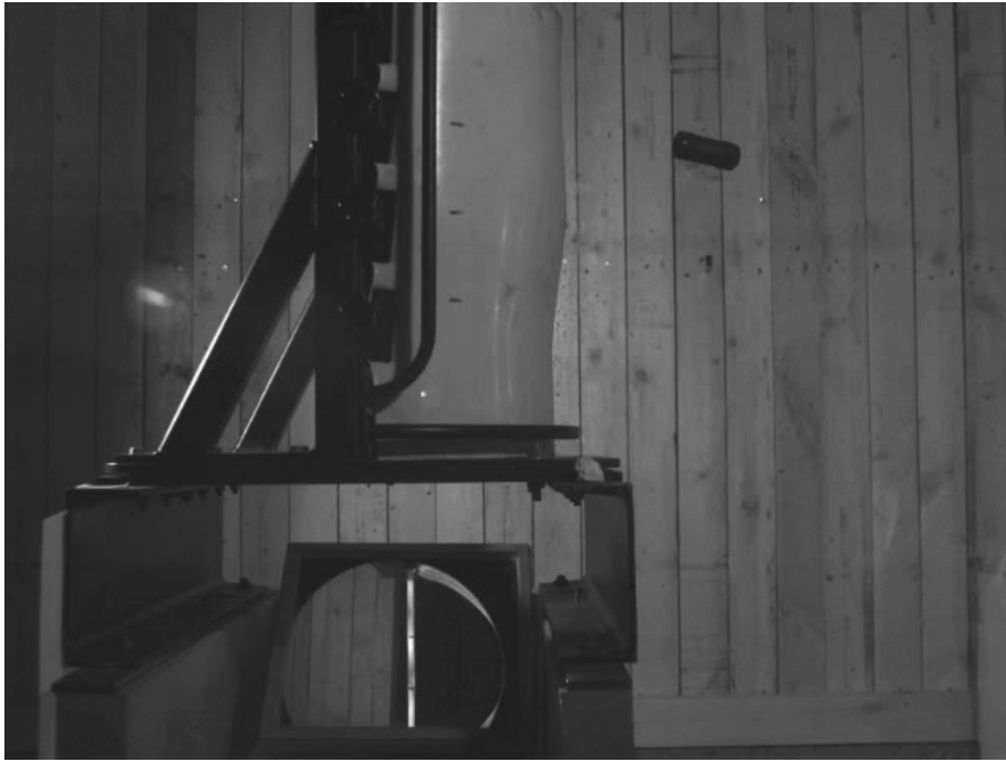
Figure 210: 4 Hole L21A1 against BABT rig (3) Time = 45.9ms
