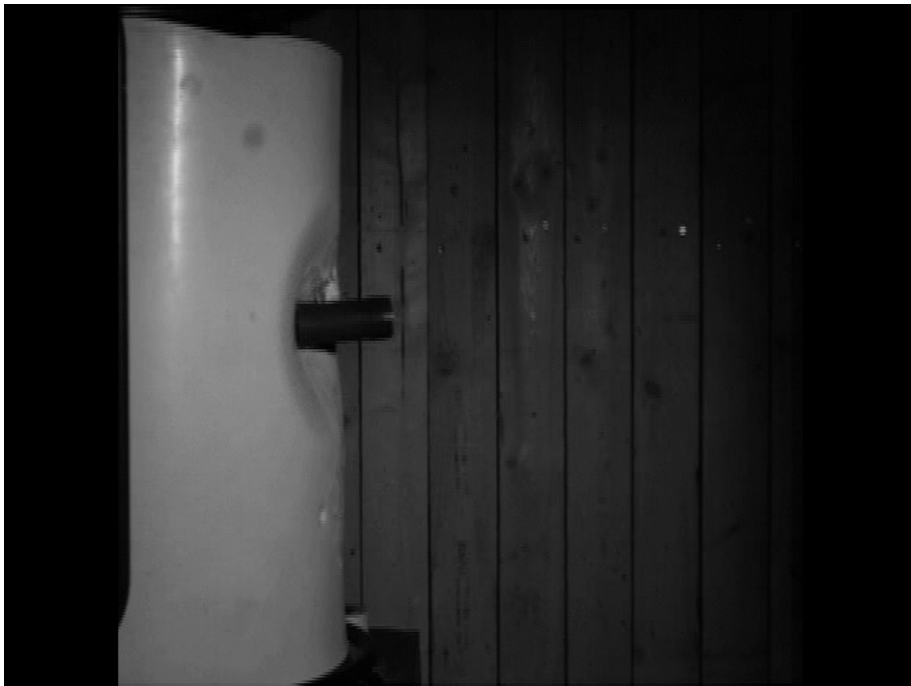
Figure 89: Sharp edged projectile T = 5\text{ms}
