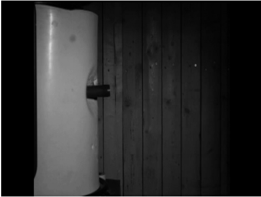
Figure 88: Sharp edged projectile T = 3\text{ms}
