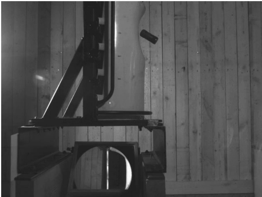
Figure 204: Standard L21A1 against BABT rig (3) Time = 10.9ms
