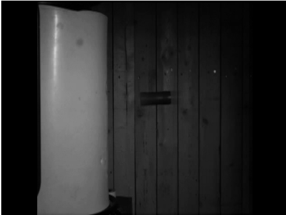
Figure 85: Sharp edged projectile in stable flight
