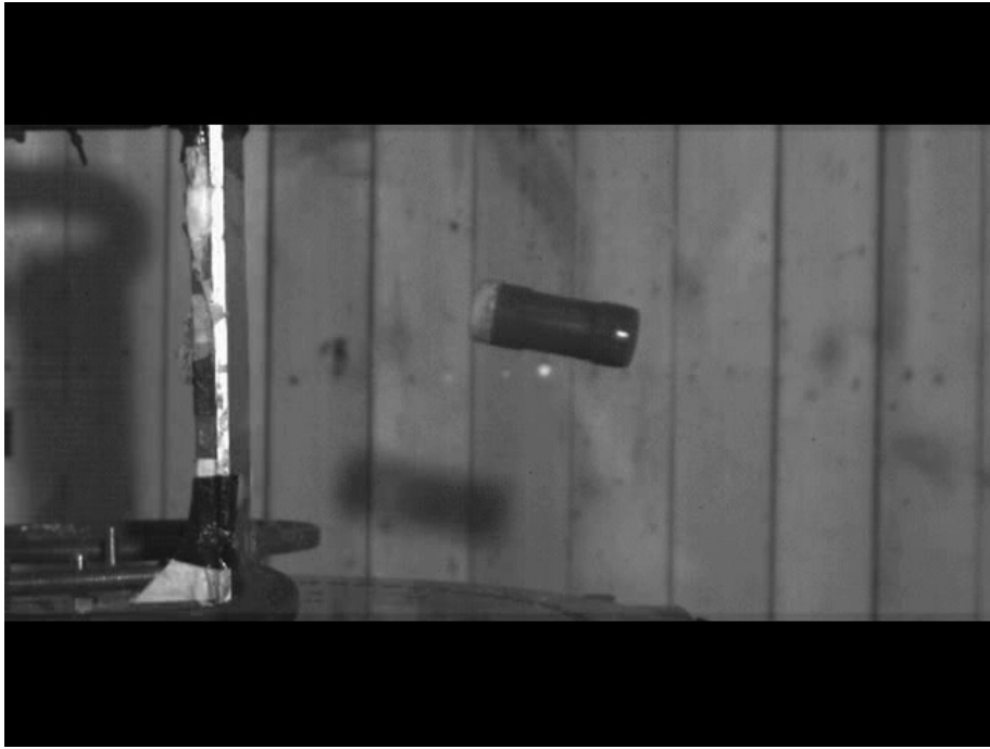
Figure 148: Foam fronted L21A1 against plate Time = 9.4ms
