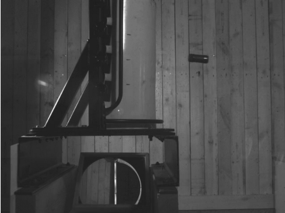
Figure 211: 4 Hole 2 Row L21A1 against BABT rig (3) Time = 0ms
