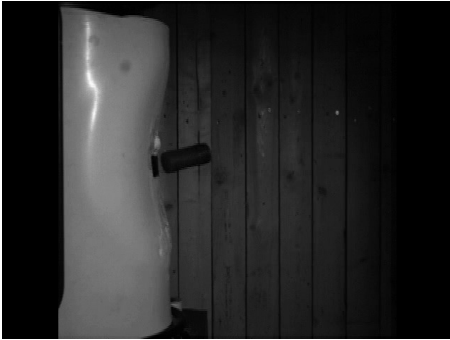
Figure 92: Sharp edged projectile T = 10\text{ms}
