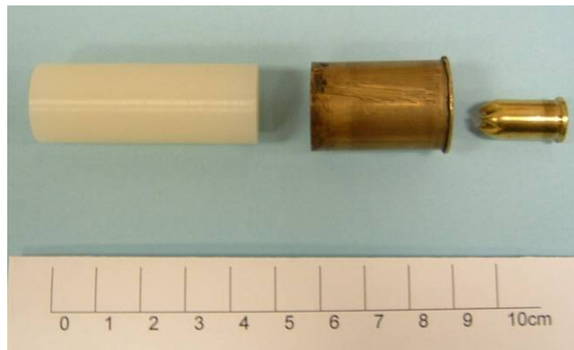
Figure 255: Projectile, Breech Adaptor and .357'' blank cartridge
