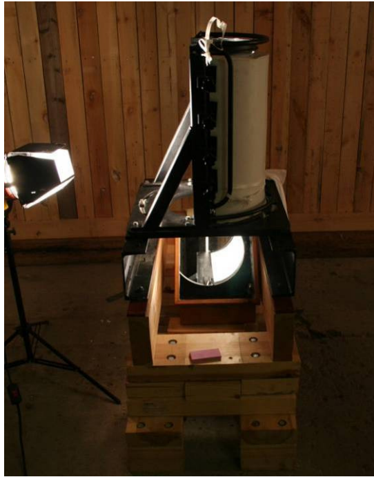
Figure 34: Behind Armour Blunt Trauma (BABT) rig with mirror and back lighting
