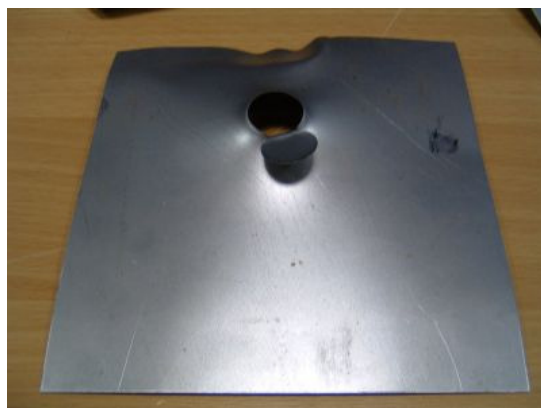
Figure 257: 170\text{ms}^{-1} impact against 1mm thick plate
