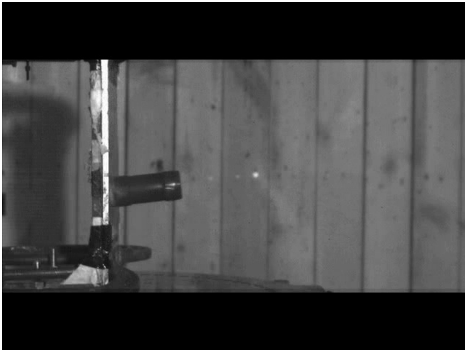
Figure 152: Felt fronted L21A1 against plate Time = 3.6ms
