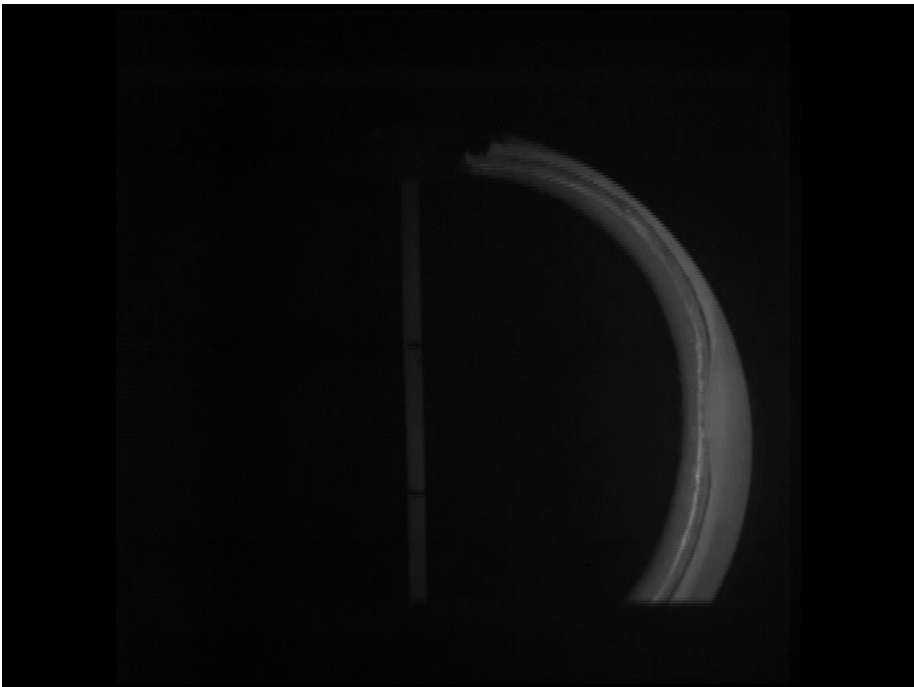
Figure 56: BABT rear face against standard L21A1 at T = 3ms
