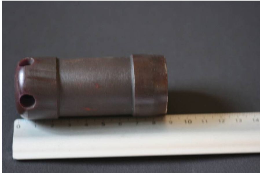
Figure 40: The standard L21A1 baton with two 8mm diameter perpendicular holes running through the nose.
