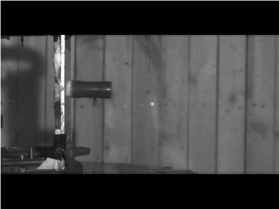
Figure 145: Foam fronted L21A1 against plate Time = 2.1ms
