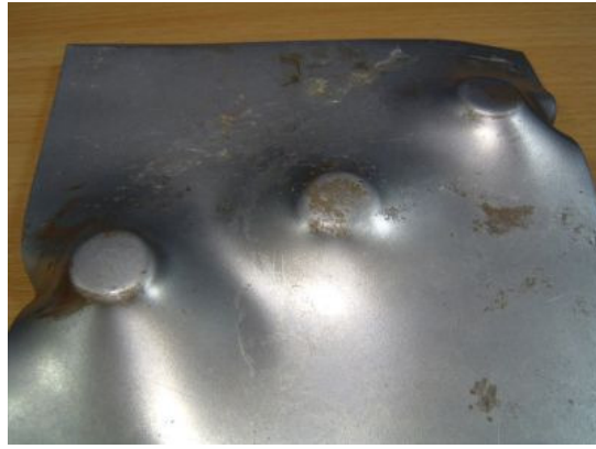
Figure 258: 160ms -1 impacts against 1mm thick plate
