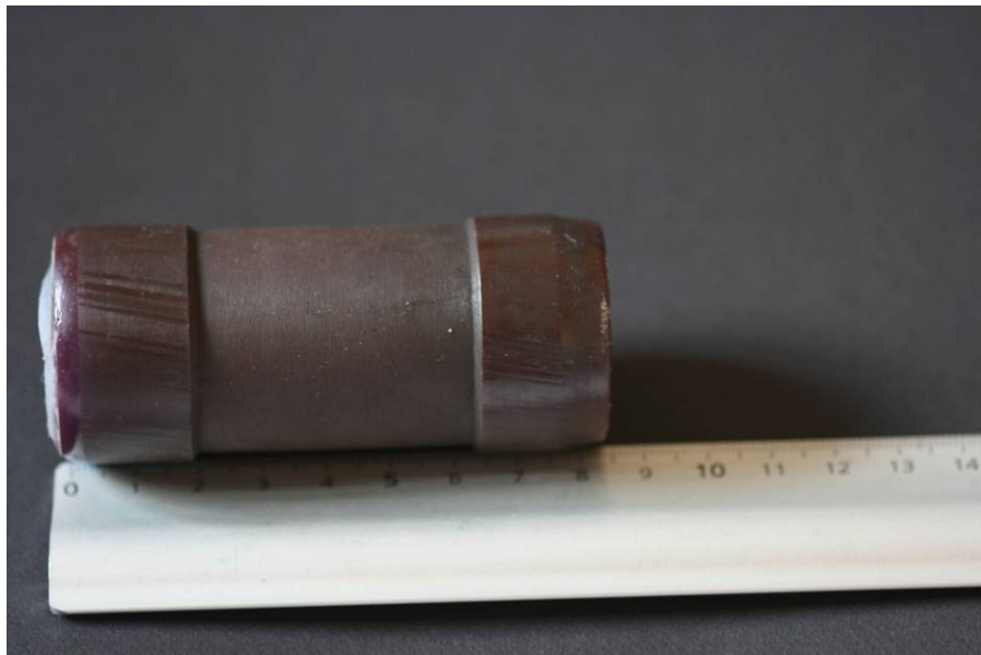
Figure 46: The side profile of the projectile remains largely unchanged with the exception of the slightly visible silicone insert
