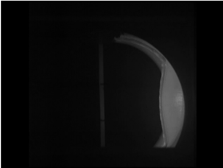
Figure 57: BABT rear face against standard L21A1 at T = 6\text{ms}
