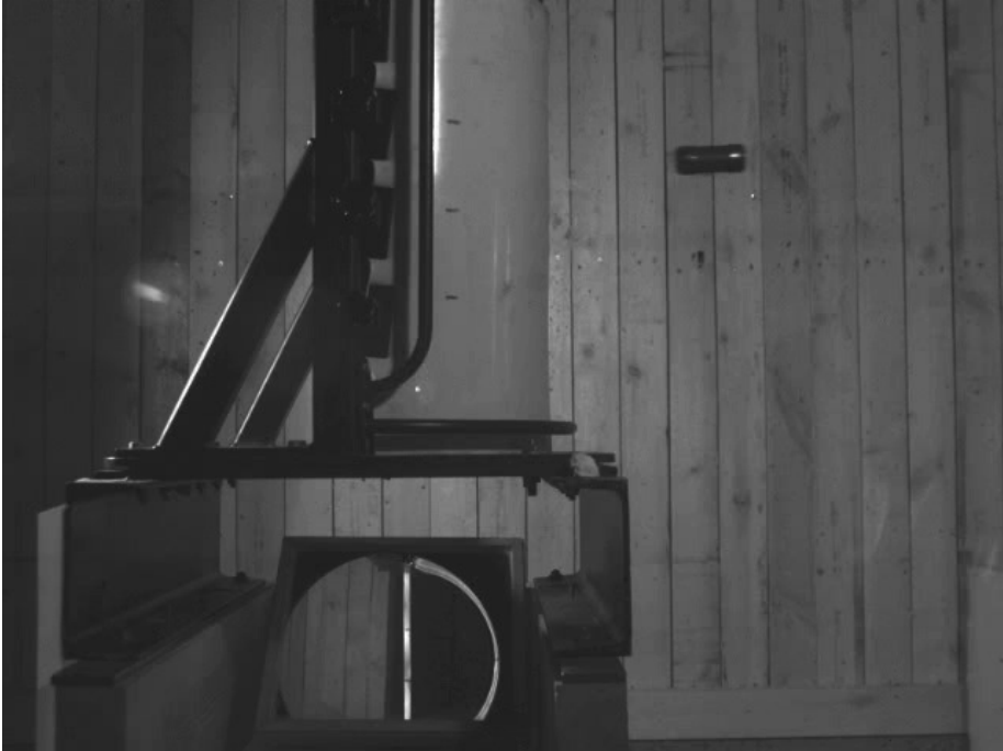
Figure 206: 4 Hole L21A1 against BABT rig (3) Time = 0ms
