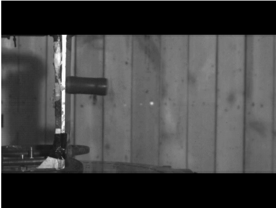
Figure 140: Standard L21A1 against plate Time = 2.1ms
