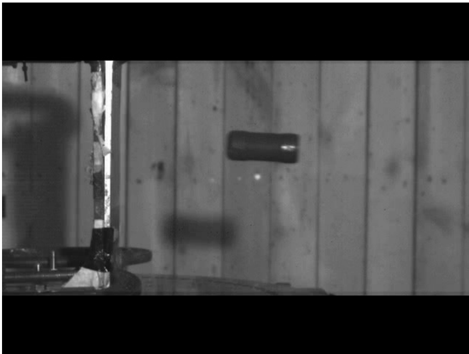
Figure 139: Standard L21A1 against plate Time = 0ms
