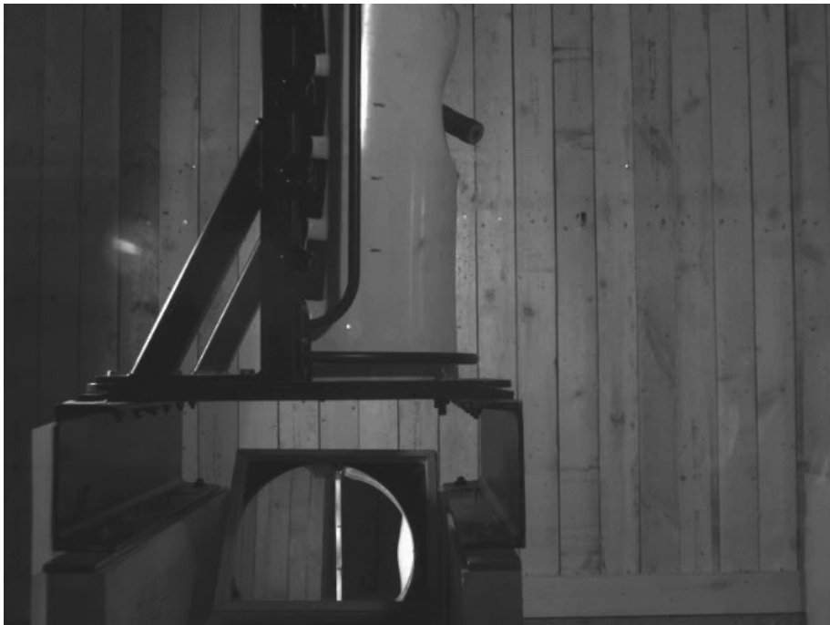
Figure 219: 2 Hole L21A1 against BABT rig (3) Time = 7.3ms
