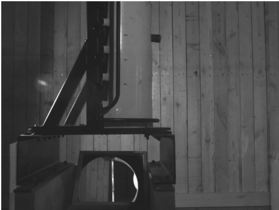
Figure 234: Hollow L21A1 against BABT rig (3) Time = 7.3ms
