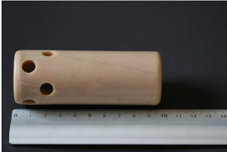
Figure 38: Modified L5A5 baton with four equispaced holes in two rows
