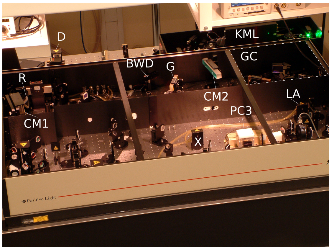
FIGURE 2.4: Annotated photograph of the Spitfire CPA system. The regen cavity runs along the front of the box and cannot be seen in this picture. D is the Dazzler. In the stretcher: R is the vertical retroreflector, G is the grating, CM1 and CM2 are the curved mirrors and BWD is the bandwidth protection device. X is the crystal for the X path amplifier. PC3 is the third Pockels cell and LA is the crystal for the linear amplifier. GC is the compressor for the 1 kHz line.
