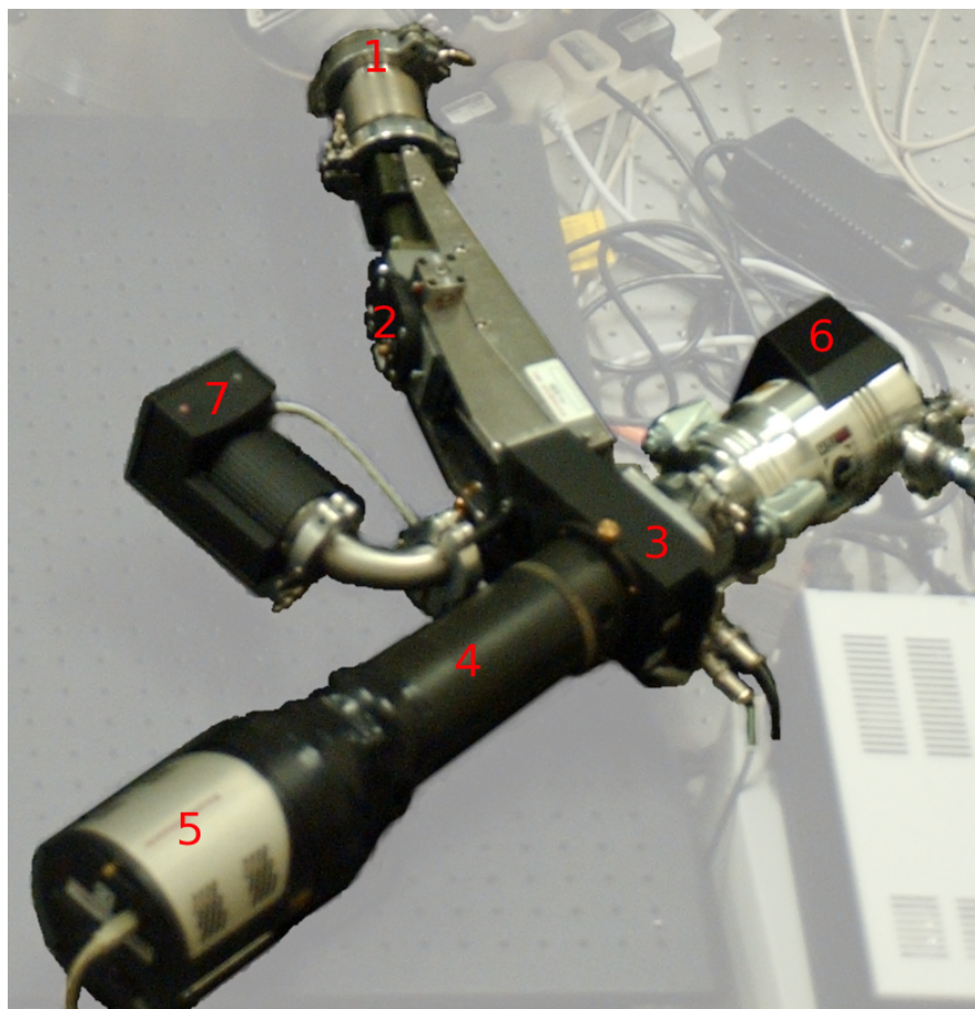
FIGURE 2.41: Grazing incidence spectrometer: 1, Entrance slit. 2, Grating. 3, MCP. 4, Lens system. 5, CCD camera. 6, Turbo pump. 7, Vacuum gauge.
