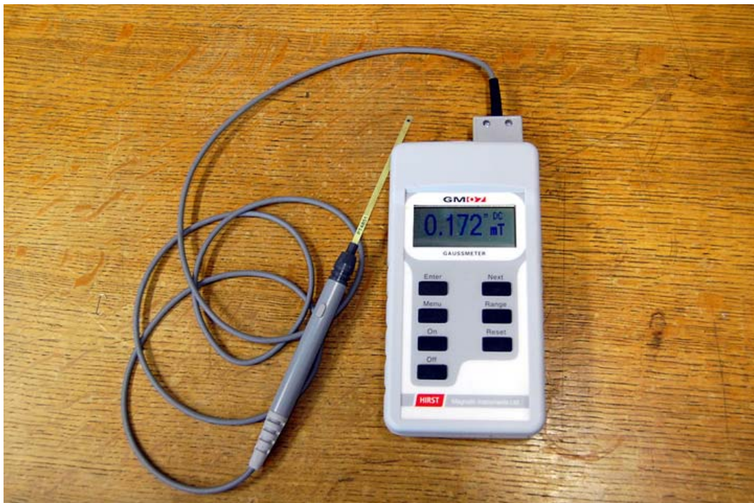
Figure 5-16 Portable Gauss meter GM07
