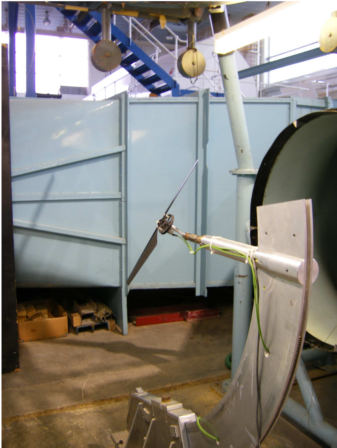
Figure B.3: Wind Tunnel testing of the Draganflyer X Pro
