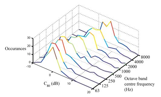
Figure B-3. Distribution of  $C_{80}$  values for database of 100 simulated room impulse responses for the octave bands from 63Hz to 8000Hz.
