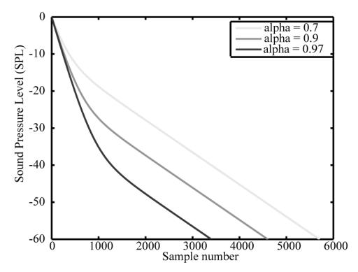
Figure 7-7. A dual exponential decay model can give non-uniform decay, where the faster decaying exponential dominates the early part of the decay curve, and the slower decaying exponential controls the late part of the decay. The decay envelopes for three different weighting factors as shown in the legend are illustrated.
