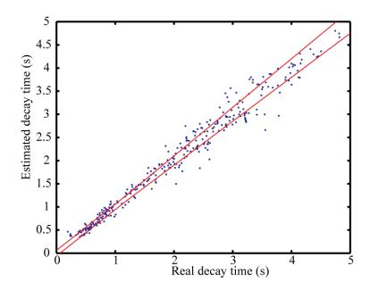
Figure 6-5. ANN estimation results on test data set for Rt using speech as test signal. Red lines indicate the subjective difference limens.
