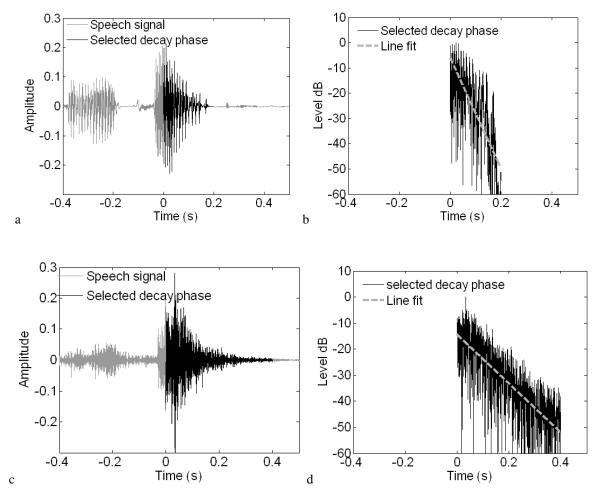
Figure 7-1. (a) and (b) the energy decay of an anechoic speech utterance saying: (dec)'imal point'. The utterance itself has a decay time equivalent to a "reverberation time" of 0.3s. (c) and (d) depict the same section of speech but recorded in a space with a reverberation time of 0.63s, the resultant decay rate of the reverberant section is equivalent to a T<sub>30</sub> of 0.64s.After Kendrick et al.[9].
