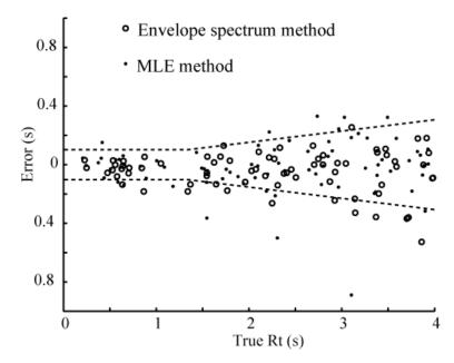
Figure 10-1. Error in parameter estimation versus the true value for reverberation time.
