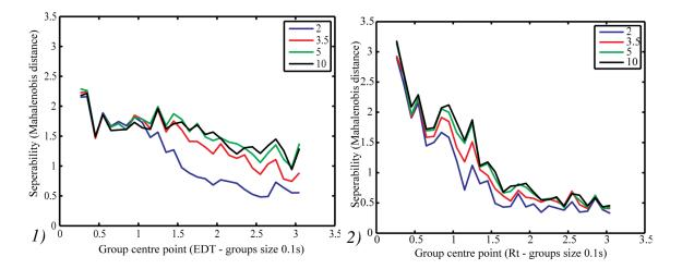
Figure 6-7. Mahalanobis distance as a function of Rt(1) and EDT(2). These plots indicate the separability of the data and how it changes with respect to decay rate. The legend indicates the window width (in seconds) used to compute the envelope spectrum.
