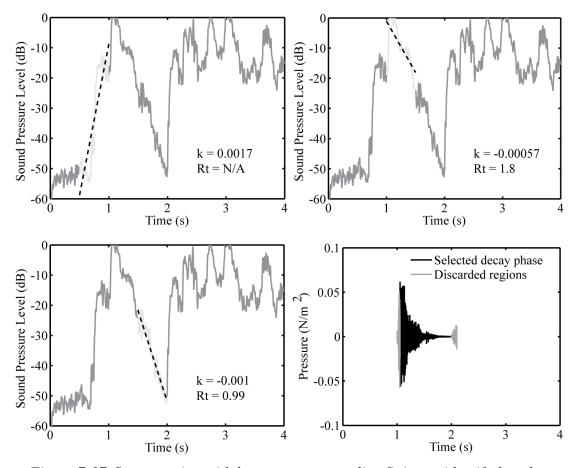
Figure 7-17. Segmentation with least mean square line fitting to identify free decay phases for further MLE. (a) Frame with positive k indicating rise edge is discarded; (b)
