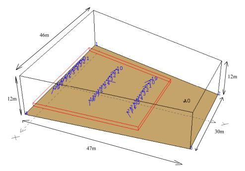
Figure 4-4. View from CATT acoustic showing one of the randomly generated room geometries. The sound source is labelled as A0, the grid of receivers is numbered from 1 to 27.
