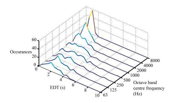
Figure B-2. Distribution of EDT values for database of 100 simulated room impulse responses for the octave bands from 63Hz to 8000Hz.
