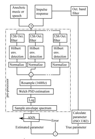
*Figure 6-18. Schematic of 12<sup>th</sup> octave envelope spectrum method for estimating room acoustic parameters from music, after Kendrick et al. [73].*
