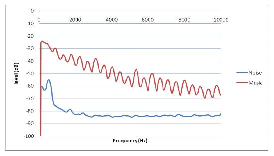
Figure 8-15. Noise vs. signal level for anechoic recordings
