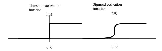
*Figure 5-2. Examples of two types of activation function: 1) threshold activation functions can take one of two values, 2) sigmoid activation functions are continuous.*
