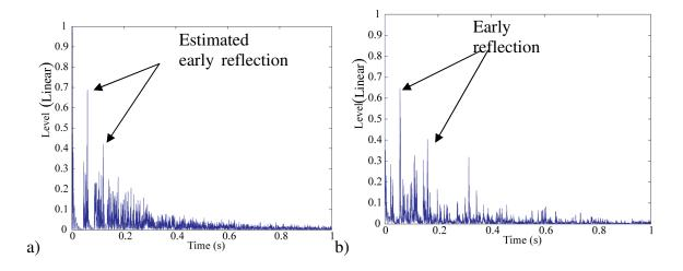
Figure 9-11. Magnitude of the impulse response estimated using combined cepstrum/ML method (a) and true impulse response (b)
