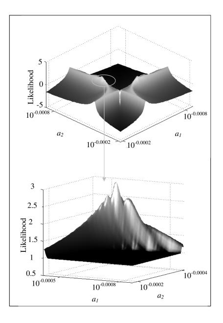
Figure 7-8. The likelihood function over a grid of exponential parameters  $a_2$  and  $a_1$ . At each location the solution has been optimised with respect to the parameter;  $\alpha$ . The maxima represent the local and global solutions. The bottom plot is a magnification of a section of the top plot as indicated.
