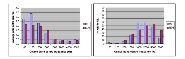
Figure 8-14. The average error for Rt and EDT as a function of octave band (left hand side) and the percentage of Rt and EDT predicted parameters within the subjective DL (right hand side). The analysis is based on the application of the ML method to simulated impulse responses convolved with 40 mins of anechoic music segmented into eight, five min segments for Rt and four, ten minute segment for EDT.
