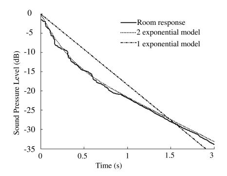
Figure 7-13. Comparison of the estimated decay curves for an artificial room response using the new dual exponential model and the single exponential model.
