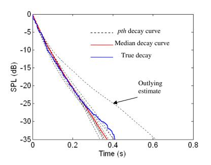
Figure 7-28. Optimal Schroeder curve estimation using eight, 60s segments of anechoic speech convolved with a real RIR. Each decay curve estimate has been backwards integrated to produce a Schroeder curve.[10]
