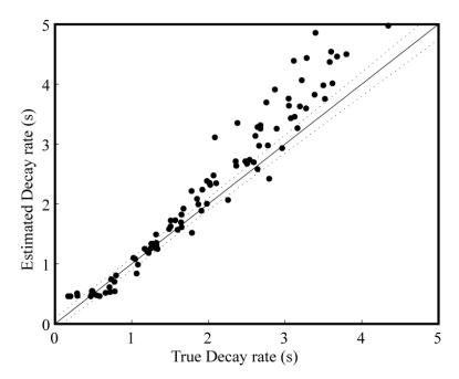
Figure 8-2. EDT estimated using ML method plotted against the true EDT for 100 simulated impulse responses and speech.
