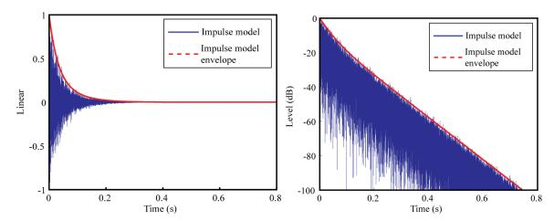
Figure 7-5. This figure shows an example of the RIR model generated from the above parameters. The plots show both the estimated envelope of the RIR (in red) and the RIR estimate (in blue)
