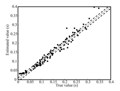
Figure 8-6. t<sub>s</sub> estimated using ML method plotted against the true t<sub>s</sub>. 100 impulse responses were chosen at random from a database. Each impulse response was convolved with 9 minutes of speech. For the ML estimation, the reverberated signal was windowed into three, 3 minute segments.
