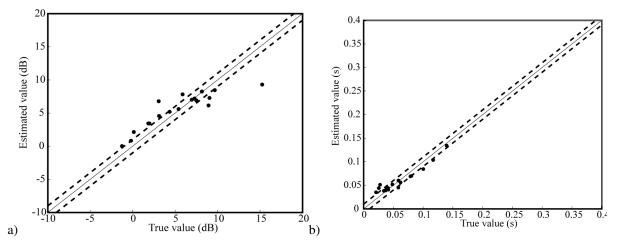
Figure F-17. Real impulse responses, 9 mins of speech windowed into 1  $\frac{1}{2}$  minute segments, results presented are for  $C_{80}(a)$  and  $t_s(b)$ .
