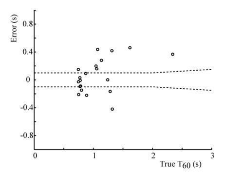
Figure 6-20. Error in Reverberation time estimation, using set of real room impulse response as test set, dotted lines indicate subjective difference limens.
