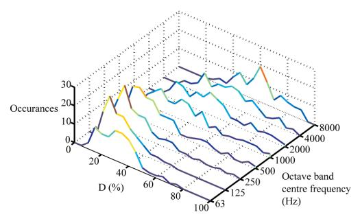
Figure B-5. Distribution of D values for database of 100 simulated room impulse responses for the octave bands from 63Hz to 8000Hz.
