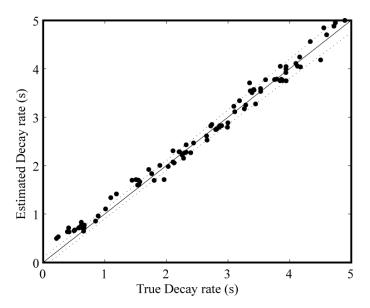
Figure 8-9. Comparison of estimated and true reverberation time. Estimates were obtained from the application of the ML method to simulated impulse responses convolved with 40 mins of anechoic music windowed into 20, two minute segments, results presented.
