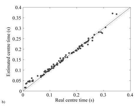
Figure 7-15. Comparison of the centre time estimated directly from impulse responses using MLE (2s length) vs. the true value
