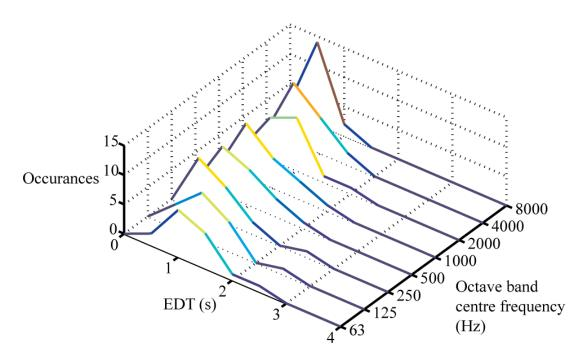
Figure C-7. Distribution of EDT values for database of 18 real room impulse responses for the octave bands from 63Hz to 8000Hz.
