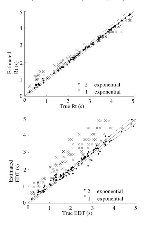
Figure 7-12. Comparison of dual and single exponential model estimations of Rt (a) and EDT (b). Maximum likelihood estimation performed directly on simulated room impulse responses. Dotted lines show perception difference limens.
