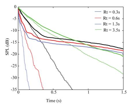
Figure E-13. Backwards integrated decay curve estimates calculated from MTFs estimated by the ANN method, dotted lines shows the estimates while bold lines show the true MTF.
