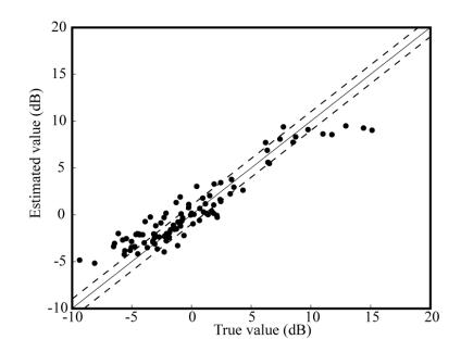
Figure 8-12. Comparison of estimated and true  $C_{80}$ . Estimates were obtained from the application of the ML method to simulated impulse responses convolved with 40 mins of anechoic music windowed into 10 minute segments.
