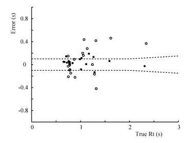
Figure 10-7. Error in reverberation time estimation versus the true value •MLE and o envelope spectrum method. Validation set using real room measurements. Music excitation. After Kendrick et al. [9].
