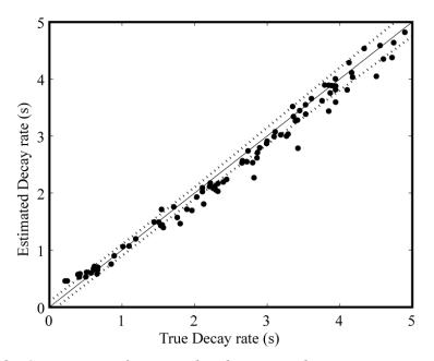
Figure 8-8. Comparison of estimated and true reverberation time. Estimates were obtained from the application of the ML method to simulated impulse responses convolved with 40 mins of anechoic music windowed into eight, five minute segments.
