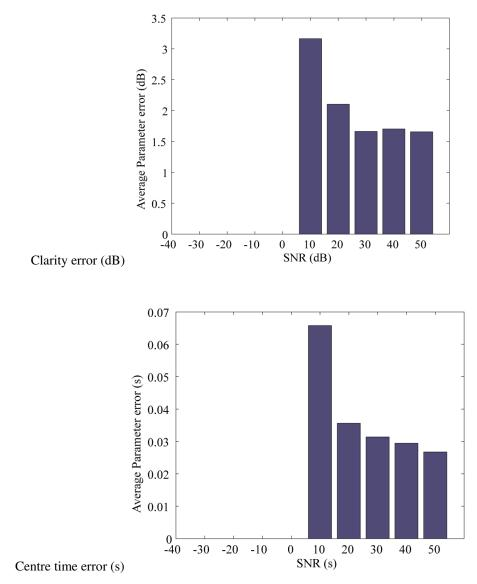
Figure 8-27. Effect of change of signal to noise ratio on parameter estimation accuracy using speech as excitation signal 1)  $C_{80}$  2)  $t_s$
