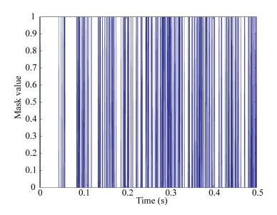
Figure 9-7. Masking function showing the temporal pattern of the early reflections
