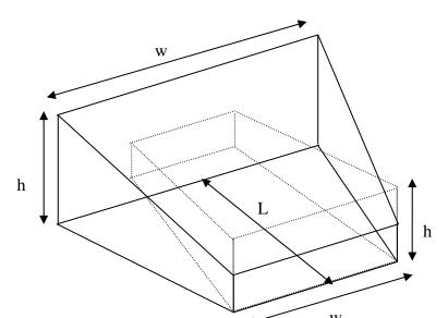
Figure 4-2. Model 2, Fan shaped room model. The dotted shape tries to demonstrate how the geometry may vary, and demonstrates how a sloping floor could occur.
