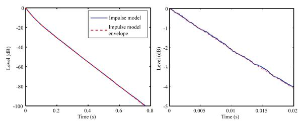
Figure 7-6. Schroeder curve of room impulse response models, the backwards integrated impulse response model and the backwards integrated RIR envelope are shown to be similar. a) shows the full dynamic range of the decay while b) shows a small section highlighting the random fluctuations in the impulse response model.
