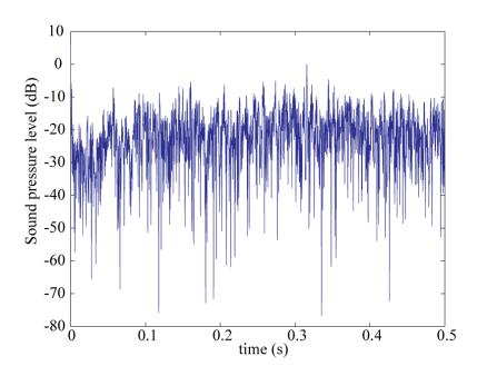
Figure 9-6. Estimated impulse response using the cepstral method with overall decaying trend removed, normalised to strongest reflection
