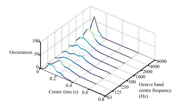
Figure B-4. Distribution of  $t_s$  values for database of 100 simulated room impulse responses for the octave bands from 63Hz to 8000Hz.
