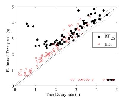
Figure 7-25. Comparison of reverberation time and EDT, estimated using all decay phases with >25dB dynamic range in a single maximum likelihood estimation and the true value. Speech received in artificial rooms.
