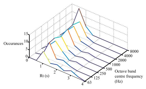
Figure C-6. Distribution of Rt values for database of 18 real room impulse responses for the octave bands from 63Hz to 8000Hz.
