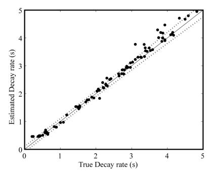
Figure 8-1. Rt estimated using ML method plotted against the true Rt for 100 simulated impulse responses and speech.
