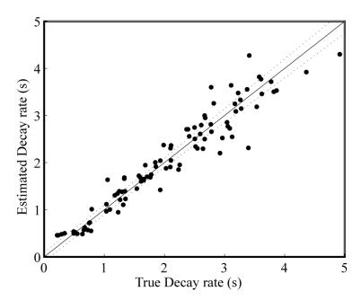
Figure 8-11. Comparison of estimated and true EDT. Estimates were obtained from the application of the MP method to simulated impulse responses convolved with 40 minutes of anechoic music windowed into four, ten minute segments.
