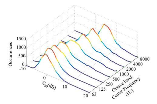
Figure 4-10. Distribution of clarity  $C_{80}$  values in the database of 8400 simulated room impulse responses for the octave bands from 63 Hz to 8000 Hz.
