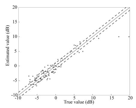
Figure 2-4. Example of plot showing accuracy of  $C_{80}$  estimations. Each dot represents an estimation and the difference limens are represented by dashed lines. This gives an indication of the accuracy of the method
