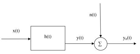
Figure 2-3. Room response to a signal including measurement noise
