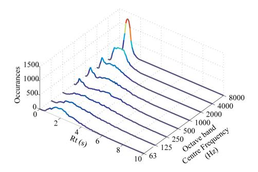
Figure 4-7. Distribution of Rt values in the database of 8400 simulated room impulse responses for the octave bands from 63 Hz to 8000 Hz.
