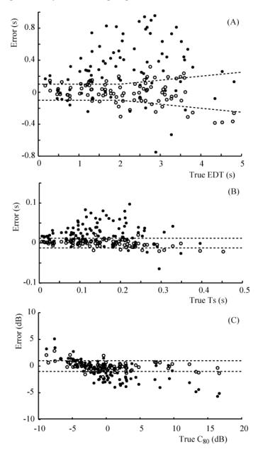
Figure 10-6. Error in parameter estimation versus the true value: (A) EDT, (B) centre time and (C) clarity • MLE and o envelope spectrum method. Validation set using simulated impulse responses. Music excitation. After Kendrick et al. [9].
