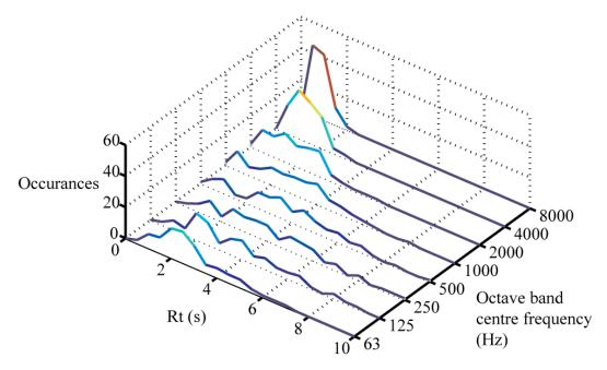
Figure A.1. Distribution of Rt values for database of 100 simulated room impulse responses for the octave bands from 63Hz to 8000Hz.
