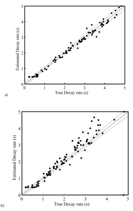
Figure 7-21. Comparison of (a) reverberation time and (b) EDT, estimated using multidecay maximum likelihood estimation and the true values. Artificially reverberated speech using simulated impulse responses (1 kHz octave band).
