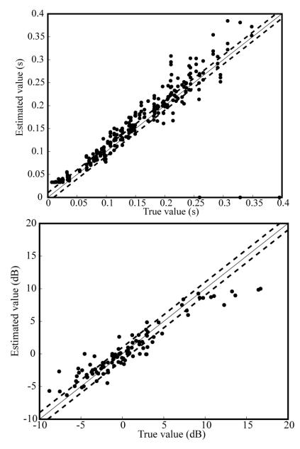
Figure 7-23. Comparison of (a) Centre time and (b)  $C_{80}$ , estimated using multi-decay maximum likelihood estimation and the true value. Speech received in simulated rooms.
