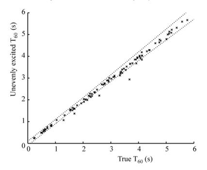
Figure 6-16. Unevenly excited reverberation time compared to the true, evenly excited value. The unevenly excited reverberation time has the same octave band frequency response as a typical piece of music. The dashed lines indicate limits derived from the perceptual difference limens after Kendrick et al. [73].
