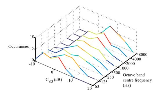
Figure C-8. Distribution of  $C_{80}$  values for database of 18 real room impulse responses for the octave bands from 63Hz to 8000Hz.
