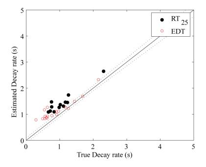
Figure 7-24. Comparison of reverberation time and EDT, estimated using all decay phases with >25dB dynamic range in a single maximum likelihood estimation and the true value. Speech received in real rooms.
