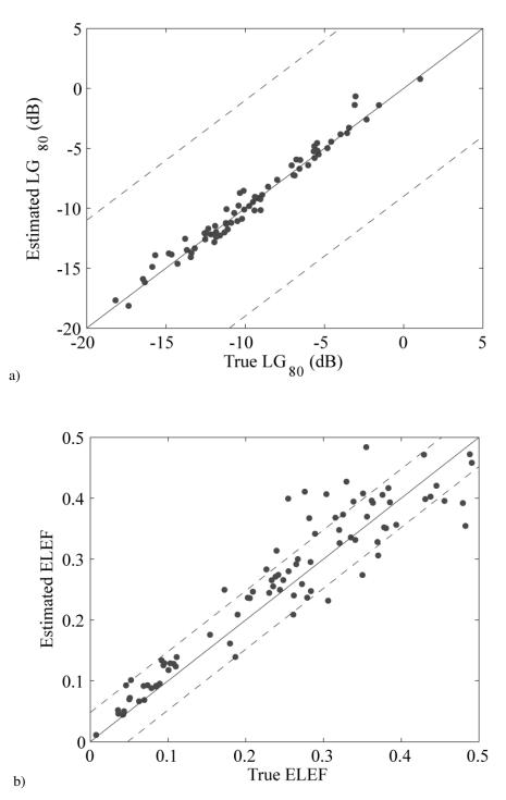
Figure 7-16. Comparison of the estimated parameters a) Late lateral strength and b) early lateral energy fraction. (estimated directly on 2s length of artificial RIRs using omni and figure-of-8 microphones)
