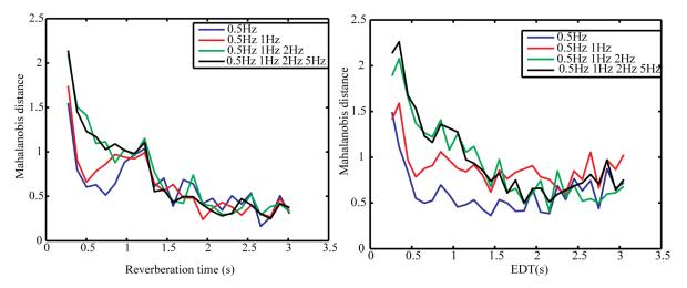
Figure 6-14. Data separability as described by the Mahalnobis distance for a sum of sine waves modulating white noise convolved with the RIR database for 1) Rt and 2) EDT. The Mahalnobis distance group step size was 0.1s.
