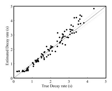
Figure 8-4. EDT estimated using ML method plotted against the true EDT. 100 RIRs were chosen at random from a database. Each impulse response was convolved with 9 minutes of speech. For the ML estimation, the reverberated signal was windowed into three, three minute segments.
