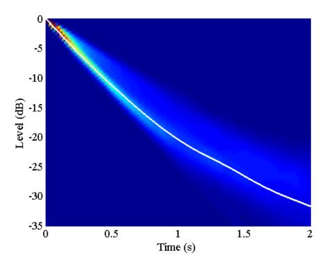
Figure 8-23. Approximate distribution of decay curve estimates, the white line is the median decay curve
