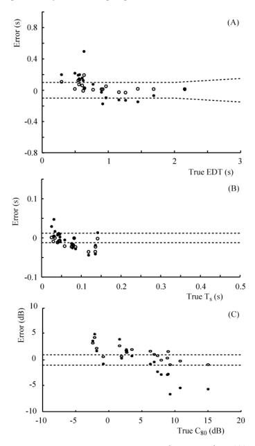
Figure 10-8. Error in parameter estimation versus the true value: (A) EDT, (B) centre time and (C) clarity.
