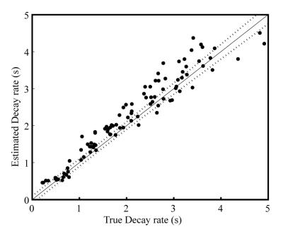
Figure 8-10. Comparison of estimated and true EDT. Estimates were obtained from the application of the MP method to simulated impulse responses convolved with 40 mins of anechoic music windowed into eight, five minute segments.
