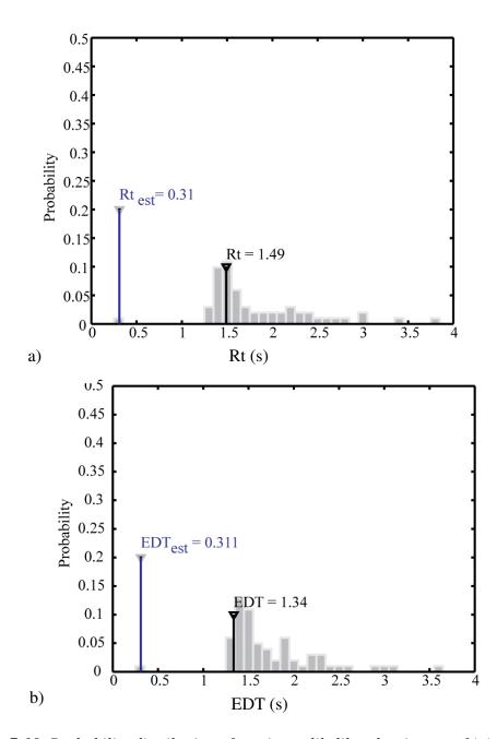
Figure 7-19. Probability distribution of maximum likelihood estimates of (a) Rt and (b) EDT, compared with actual Rt and EDT values. Minimum ML estimates  $RT_{EST}$  and  $EDT_{EST}$  are show on the plots. 90s speech stimulus for a single artificial room response.
