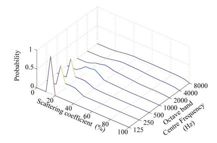
Figure 4-3. Distribution of possible scattering coefficients used in defining the material properties of the room, each line represents the distribution of possible scattering coefficients used in the room model for each octave band.
