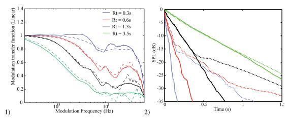
Figure E-14. Backwards integrated decay curve estimates(2) calculated from MTFs(1) estimated by the ANN method using PCA pre-processing, dotted lines shows the estimates while bold lines show the true MTF.
