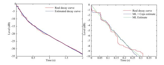
Figure 9-12. Impulse response estimated from reverberant speech using combined cepstrum and ML method.
