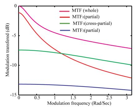
Figure 6-10. MTF evaluated for a model of non-uniform sound decay using a sum of exponentials. The partial MTFs are shown for each exponential as well as the cross term and the whole MTF
