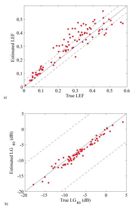
Figure 8-22. Maximum likelihood estimates for a) Early Lateral Energy Fraction (ELEF) and b)Late Lateral Reflection Strength LG.
