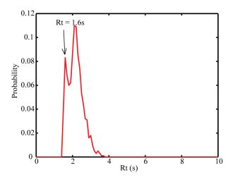
Figure 7-3. Histogram of ML decay rate estimates, showing how the first peak is selected as the best estimate.
