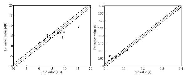
Figure F-19. Real impulse responses, 40 mins of speech windowed into 4 minute segments, results presented are for  $C_{80}$  (a) and  $t_s$  (b).
