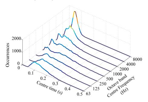
*Figure 4-9. Distribution of centre time t<sub>s</sub> values in the database of 8400 simulated room impulse responses for the octave bands from 63 Hz to 8000 Hz.*
