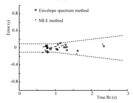
*Figure 10-3. Error in parameter estimation versus the true value for Rt.* • *MLE and o envelope spectrum method. Validation set using real RIR. After Kendrick et al. [9].*
