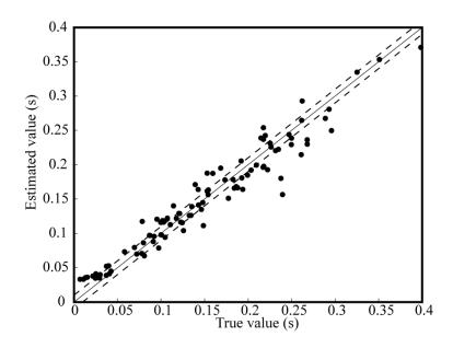
Figure 8-13. Comparison of estimated and true t<sub>s</sub>. Estimates were obtained from the application of the ML method to simulated impulse responses convolved with 40 mins of anechoic music windowed into 10 minute segments
