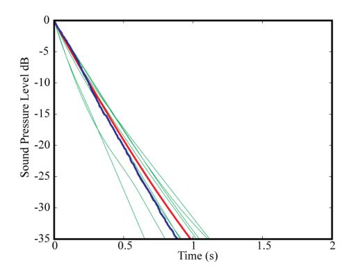
Figure 8-21. Decay curve estimates for the Haden Freeman Concert Hall. Green lines are individual segment estimates, red is the optimal decay curve estimate and blue is the averaged true decay curve from 4 snare hits. 8, 10 minute segments were used.
