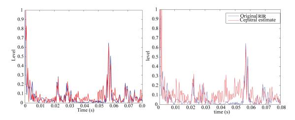
Figure 9-5. Estimated early sound field using averaged cepstra from 500ms windows whose starting point is automatically detected as the initial onsets of speech utterances (a) and averaged cepstra from all 90s of speech using 95% overlapping 3sec windows (b). Plots have been scaled for comparison purpose.
