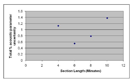
*Figure 8-25. The 90% confidence limits expressed as a fraction of the actual parameter and averaged over all parameters, as a function of the segment length.*
