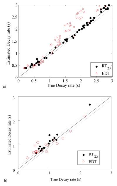
Figure 7-26. Comparison of reverberation time and EDT, estimated using 180s of speech, reverberated and segmented into 4 segments. Fastest decaying reponse with at least 25dB dynamic range selected and 4 decay phases used to estimate final decay curve. a) simulated rooms, b) real rooms
