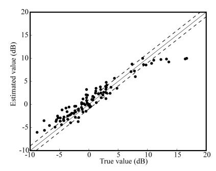
Figure 8-5.  $C_{80}$  estimated using ML method plotted against the true  $C_{80}$ . 100 impulse responses were chosen at random from a database. Each impulse response was convolved with 9 minutes of speech. For the ML estimation, the reverberated signal was windowed into three, 3 minute segments.
