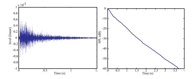
*Figure 4-5. a) Simulated room impulse response and b) decay curve produced from simulated impulse response for the example room model.*
