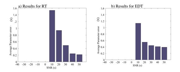
Figure 8-26. Effect of change of signal to noise ratio on parameter estimation accuracy using speech as excitation signal a) result for RT, b) result for EDT.
