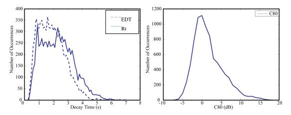
Figure 4-6. Distribution of Rt and EDT and  $C_{80}$  values in the database of 8400 simulated room impulse responses averaged over the octave bands from 63Hz to 8000Hz.
