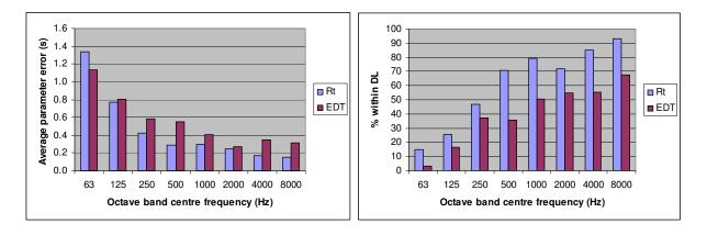
Figure 8-7. The average error for Rt and EDT as a function of octave band (left plot) and the percentage of Rt and EDT predicted parameters within the subjective DL (right plot) using simulated impulse responses convolved with 9 mins of anechoic speech windowed into three, 3 minute segments.
