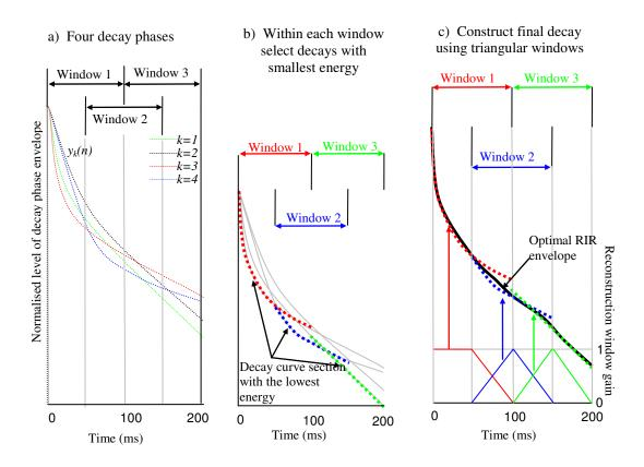
Figure 7-27. Optimal RIR envelope construction from a set of ML estimates. After Kendrick et al. [7].
