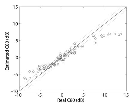
Figure 7-14. Comparison of the clarity estimated directly from impulse responses using MLE (2s length) vs. the true value.
