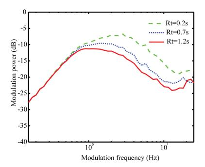
Figure 6-3. Example of speech envelope spectra received in different reverberant environments. Simple exponential impulse responses with reverberation times of 0.2s, 0.7s and 1.2s are generated and convolved with the speech signal. A 3.5s window is used in the spectrum estimation.
