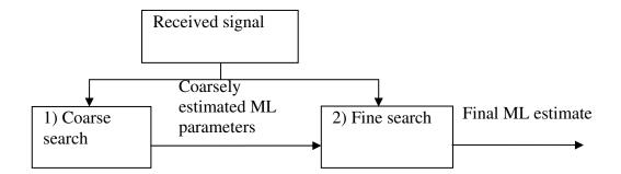
Figure 7-9. Minimisation overview. A two stage algorithm is employed. First a coarse search is applied to the likelihood function with the aim of finding the region where the global minimum is most likely to be present. Then these parameters are used as the starting point for a more detailed optimization.
