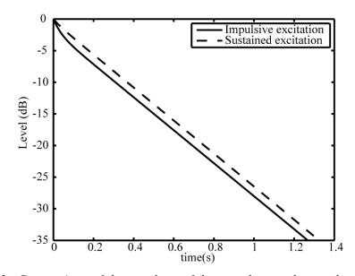
Figure 8-3. Comparison of the envelope of the reverberant decay when the RIR is excited using impulsive excitation and when the response is a sustained noise source switched off after a long period of time.
