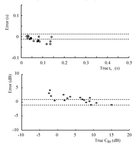
Figure 6-22. Error in  $t_s$  and  $C_{80}$  estimation, using set of real room impulse responses as test set, dotted lines indicate subjective difference limens.
