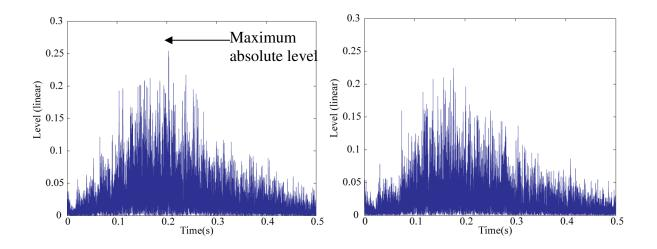
*Figure 8-17. Examples of the 'distributed source' impulse responses. Impulse responses recorded by orchestra members clapping simultaneously.*
