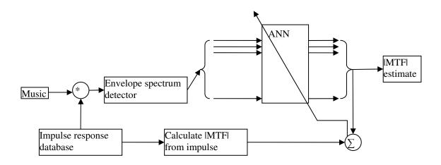
Figure E-11. Neural network method to estimate MTF directly from envelope spectra
