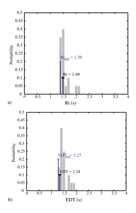
Figure 7-20. Probability distribution of maximum likelihood estimates with >25dB dynamic range of (a) Rt and (b) EDT, compared with actual Rt and EDT values . Minimum ML estimates  $RT_{EST}$  and  $EDT_{EST}$  are show on the plots. 90s speech stimulus for a single artificial room response.
