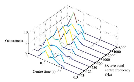
Figure C-9. Distribution of  $t_s$  values for database of 18 real room impulse responses for the octave bands from 63Hz to 8000Hz.
