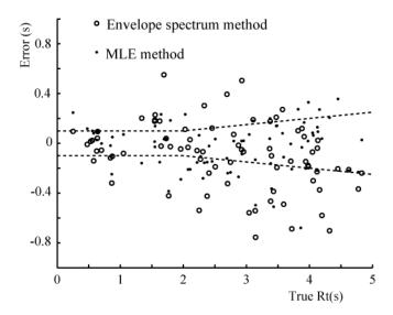
Figure 10-5. Error in reverberation time estimation versus the true value. The •MLE and **o** envelope spectrum method. Validation set using simulated impulse responses. Music excitation. After Kendrick et al. [9].
