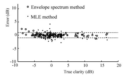
Figure 10-2. Error in parameter estimation versus the true value for clarity • MLE and • envelope spectrum method. Validation set using simulated impulse responses. Speech excitation. After Kendrick et al. [9].
