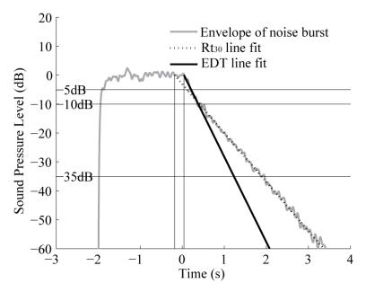
Figure 2-2. Decay curve of an enclosure, the straight lines demonstrate how the  $Rt_{30}$ and EDT are calculated. After Kendrick et al. [9]
