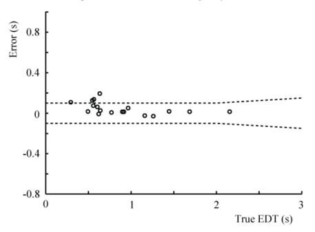
Figure 6-21. Error in EDT estimation, using set of real room impulse responses as test set.
