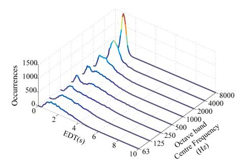
Figure 4-8. Distribution of EDT values in the database of 8400 simulated room impulse responses for the octave bands from 63 Hz to 8000 Hz.
