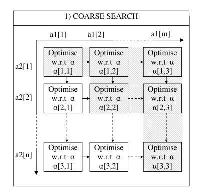
Figure 7-11. Coarse search method. Only the shaded cells are processed due to symmetry, the cost function is exhaustively computed at all highlighted grid points to reduce the chance of missing out on possible solutions in the coarse search. The sequential quadratic programming method [83] is used to minimize with respect to a at each grid position.
