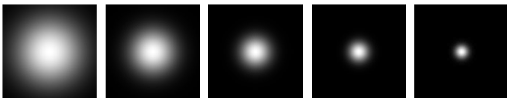
Figure 5.24: An example of flattened 3D texture for storing a Gaussian temporal kernel using r_t = 5 . From left to right slices for the current frame to the last forward/backward frame. Note that the kernel from backward and forward frames are symmetric, so there is the need to only store only one direction.
