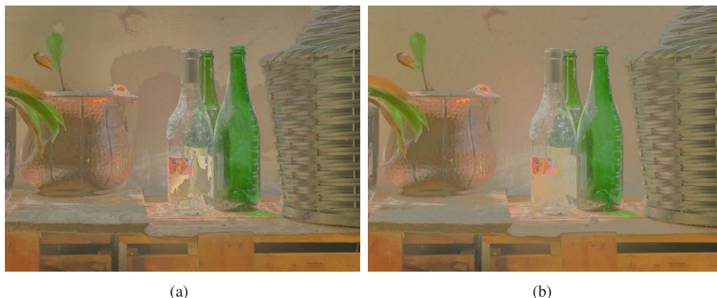
Figure 2.29: An example of Tumblin Rushmeier’s TMO [193] using adaptive luminance calculated by the segmentation method by Yee and Pattanaik [224] applied to the Bottles HDR image: a) The adaptation luminance is calculated with only 5 layers, in this case bands are visible creating artifacts. b) The adaptation luminance is calculated with 32 layers, in this case bands are not visible.
