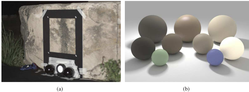
Figure 1.3: An example of capturing samples of a BRDF: a) A tone mapped HDR image showing a sample of the BRDF from a Parthenon's block [188]. b) The reconstructed materials in a) from many samples. Images are courtesy of Paul Debevec [188].
