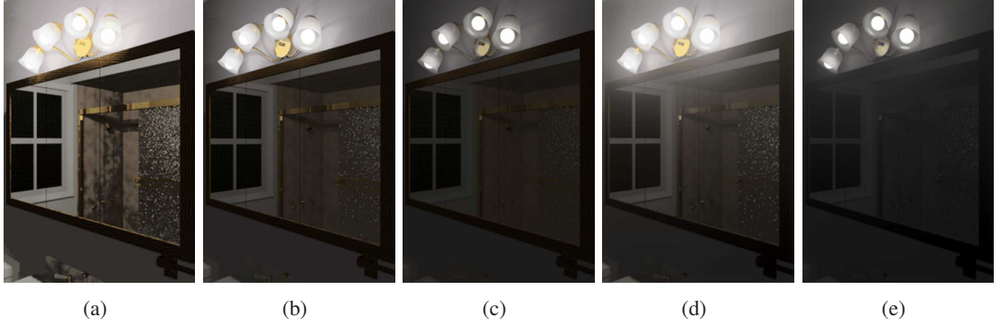
Figure 2.16: The various stage of Histogram adjustment by Ward et al. [107] applied to the Bathroom HDR image: a) The classic histogram equalisation. b) The histogram equalisation using truncation. c) Simulation of human contrast. d) Simulation of glare. e) The final image with all effects. Images are courtesy of Greg Ward [107].
