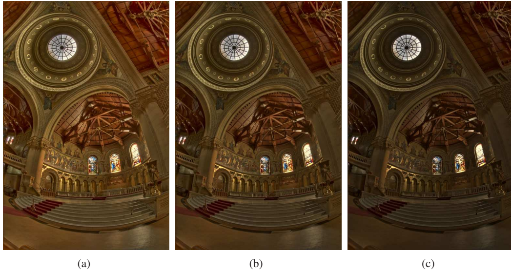
Figure 2.28: An example of tone mapping using the gradient domain operator by Fattal et al. [61] varying \beta parameter applied to Stanford Memorial Church HDR image: a) \beta = 0.7 . b) \beta = 0.8 c) \beta = 0.9 . Note that increasing \beta the overall look of the image gets darker. The original HDR image is courtesy of Paul Debevec [47].
