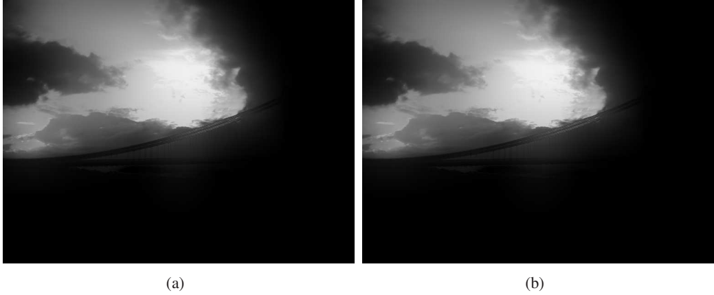
Figure 5.21: An example of expand map calculated at low resolution: a) An expand map calculated at full resolution. b) An expand map calculated at one 16th of the original resolution. Note that the differences are difficult to notice due to the smooth nature of \Lambda .
