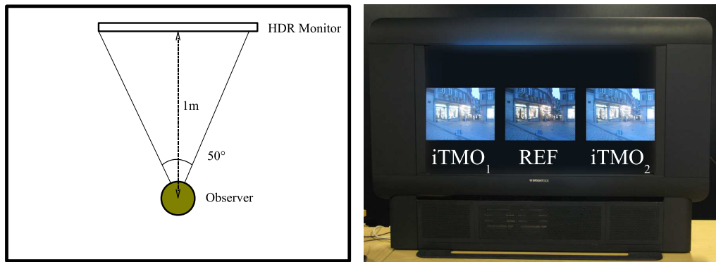
Figure 6.1: The setup of experiments. On the left side a diagram showing the setup of the experiment. On the right side an example of a paired comparison using the Dolby DR-37P HDR display. Subjects were required to determine which image (left or right) was most similar to the reference (middle).
