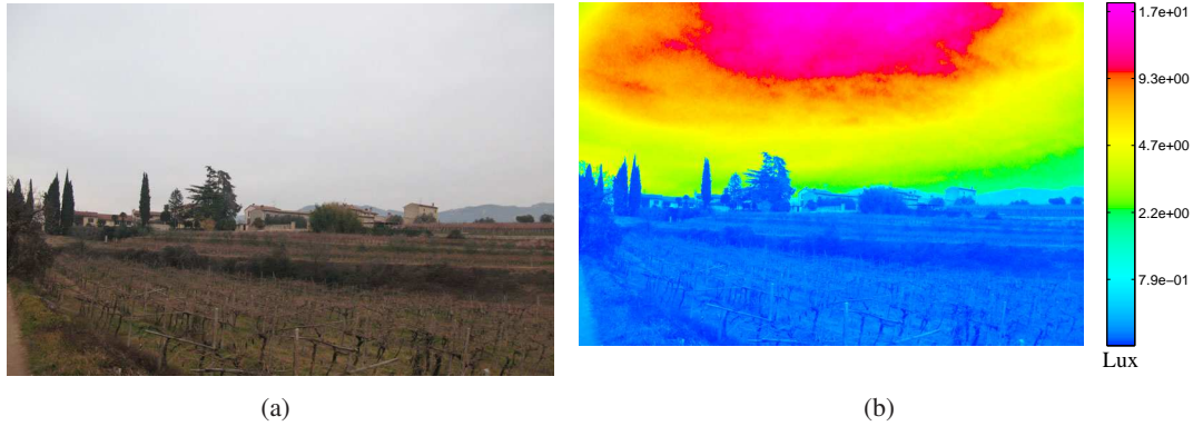
Figure 5.4: An example of expansion for well-exposed content for the Vineyard LDR image: a) The original LDR image. b) The false colour image of the expanded image in a) using Equation 5.7 with L_{w, \text{Max}} = 20 and L_{\text{white}} = 40 . Note that there are no over/under-exposed, so there are no missing areas with details and colours.
