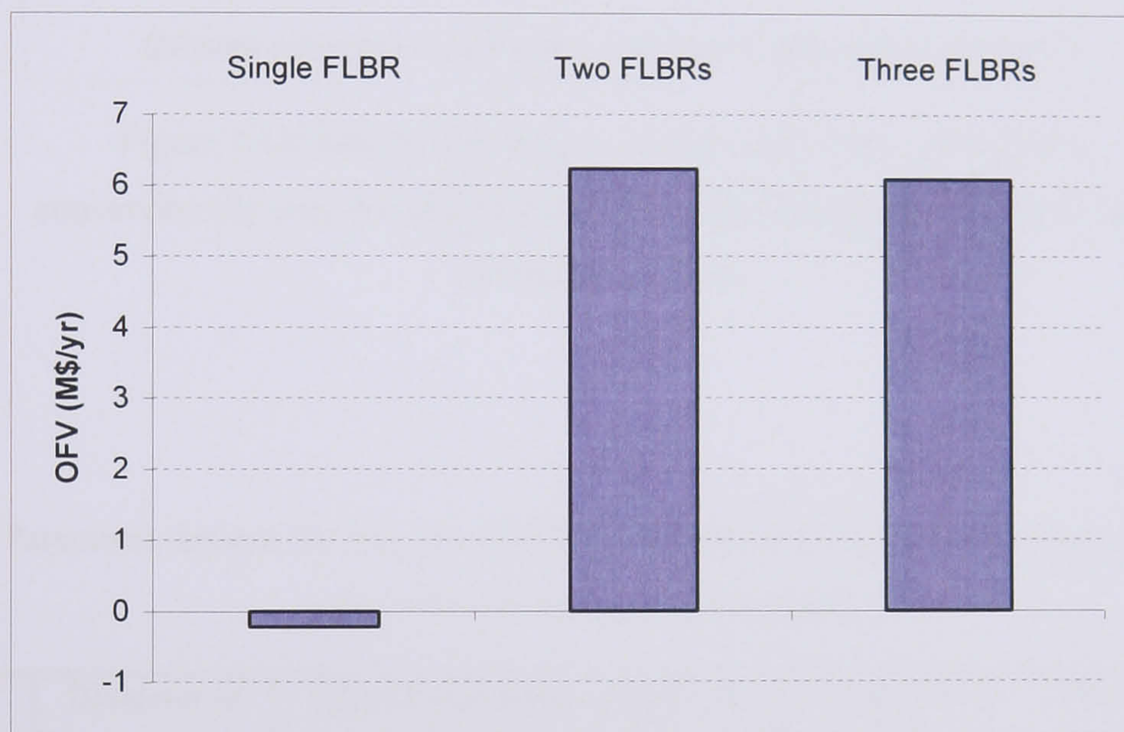
Figure 7.40: OFV for one, two and three FLBRs with 20 tubes in parallel for the acetic acid production process.
