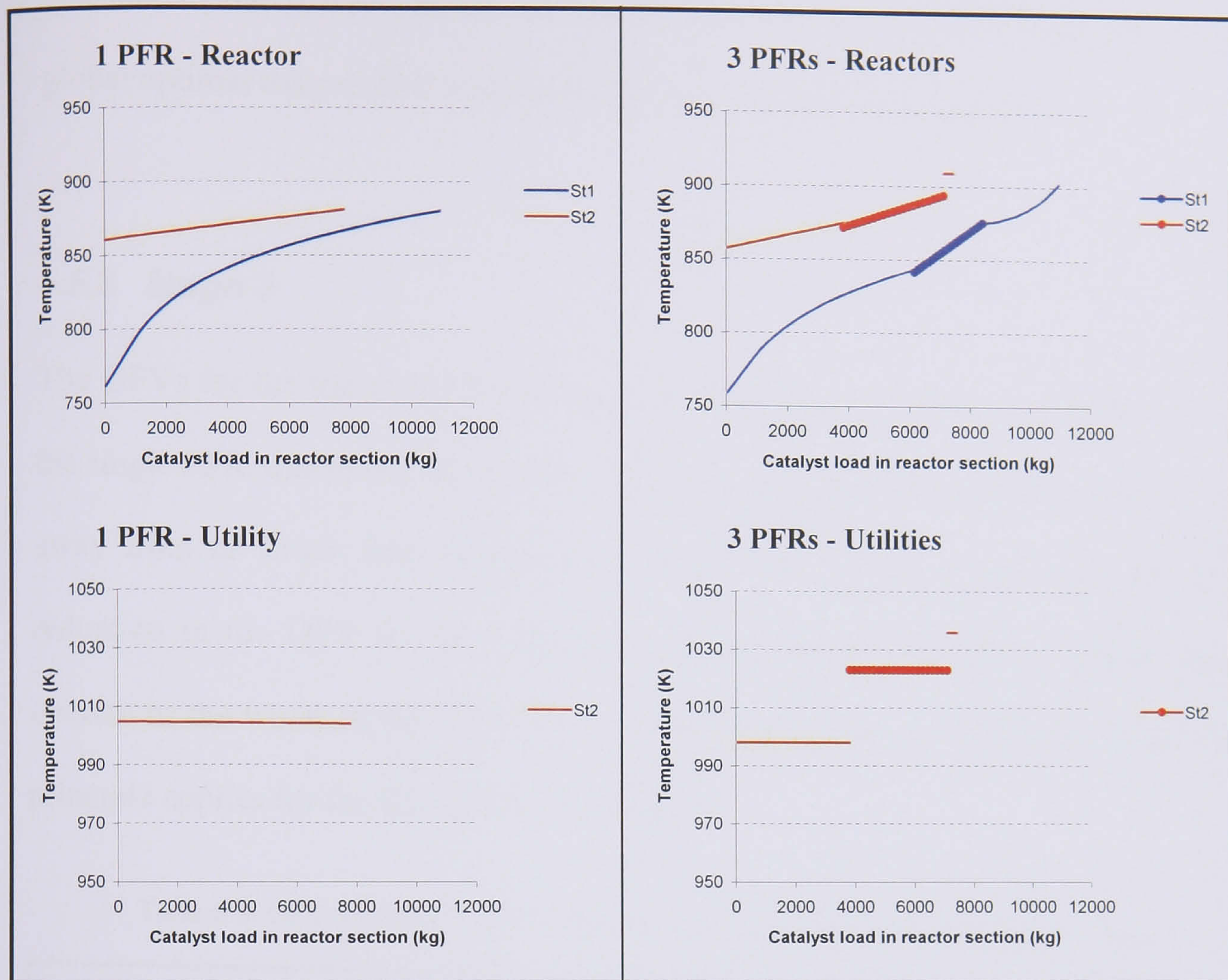
Figure 6.8: Temperature profiles for one and three PFRs in Stage 1 and 2 for the styrene production process: a) reactors, b) utilities.
