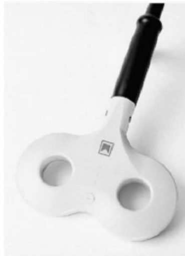
Figure 6.3. A 70 mm double circular coil used to deliver monophasic magnetic pulses.
