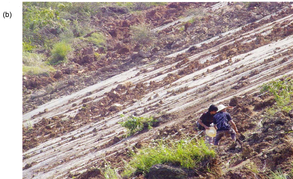
Figure 7. From Yueping (2008). Qiangjiangping landslide: (a) Sections of the slope before and after the slide and (b) photo of the slip surface.
