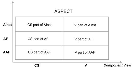
CS: Common Structure V: Variations AAF: Abstract Aspect Frame AF: Aspect Frame AInst: Aspect Instance Figure 4.1 A two dimensional view of an Aspect
