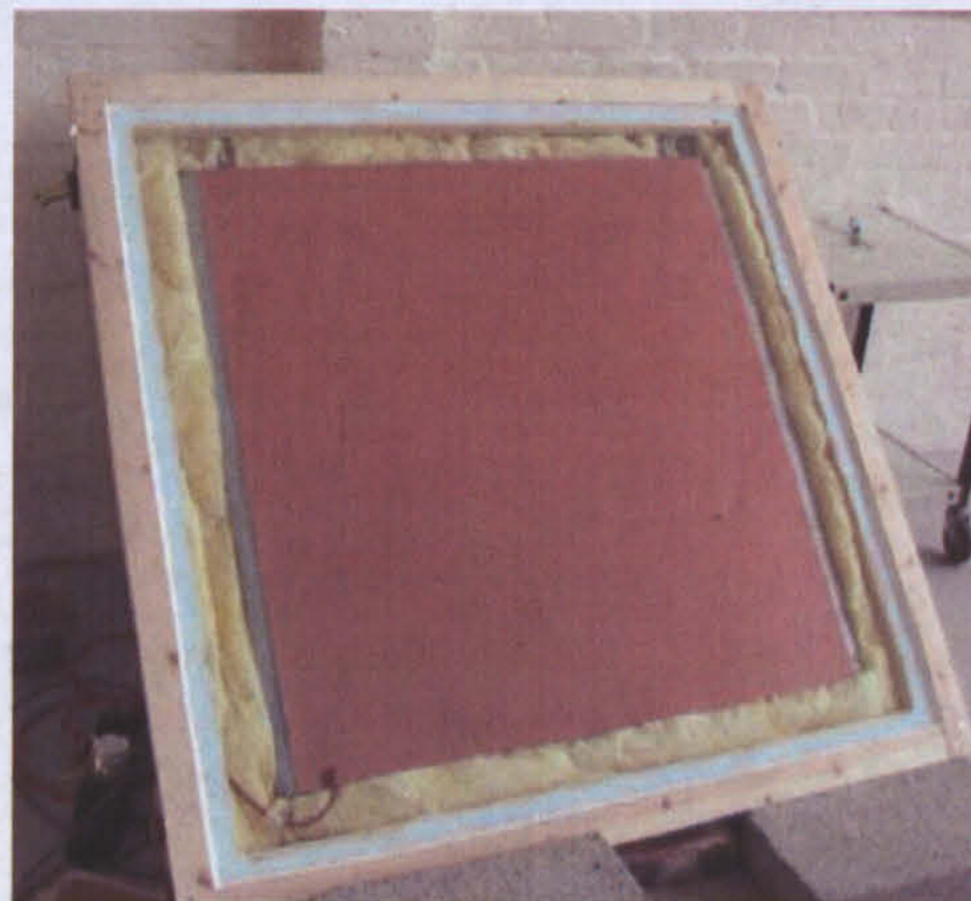
Figure 3.11: Silicone rubber resistance heating pad for applying the desired heat flux
