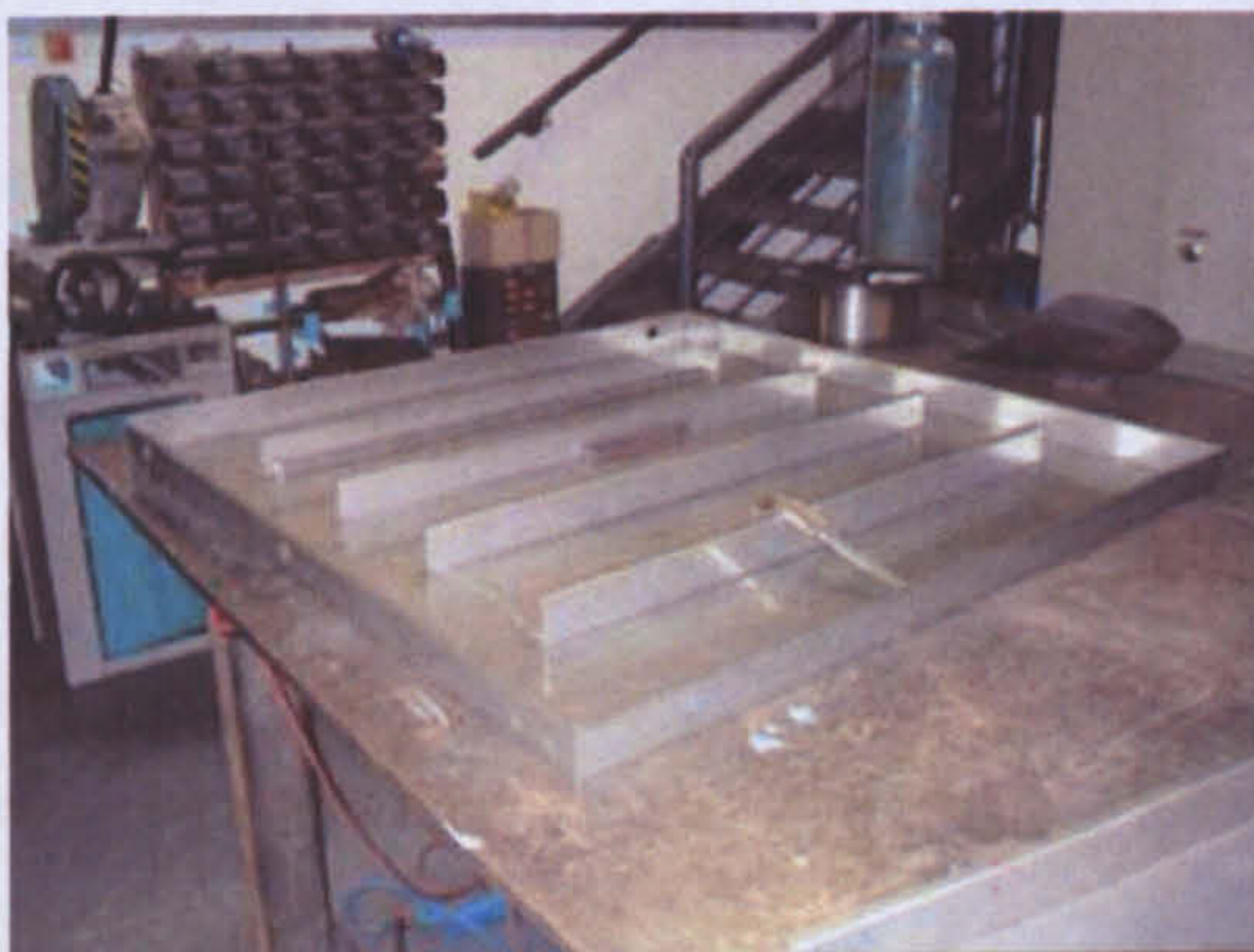
Figure 3.6: The finned heater after bending and before the welding process
