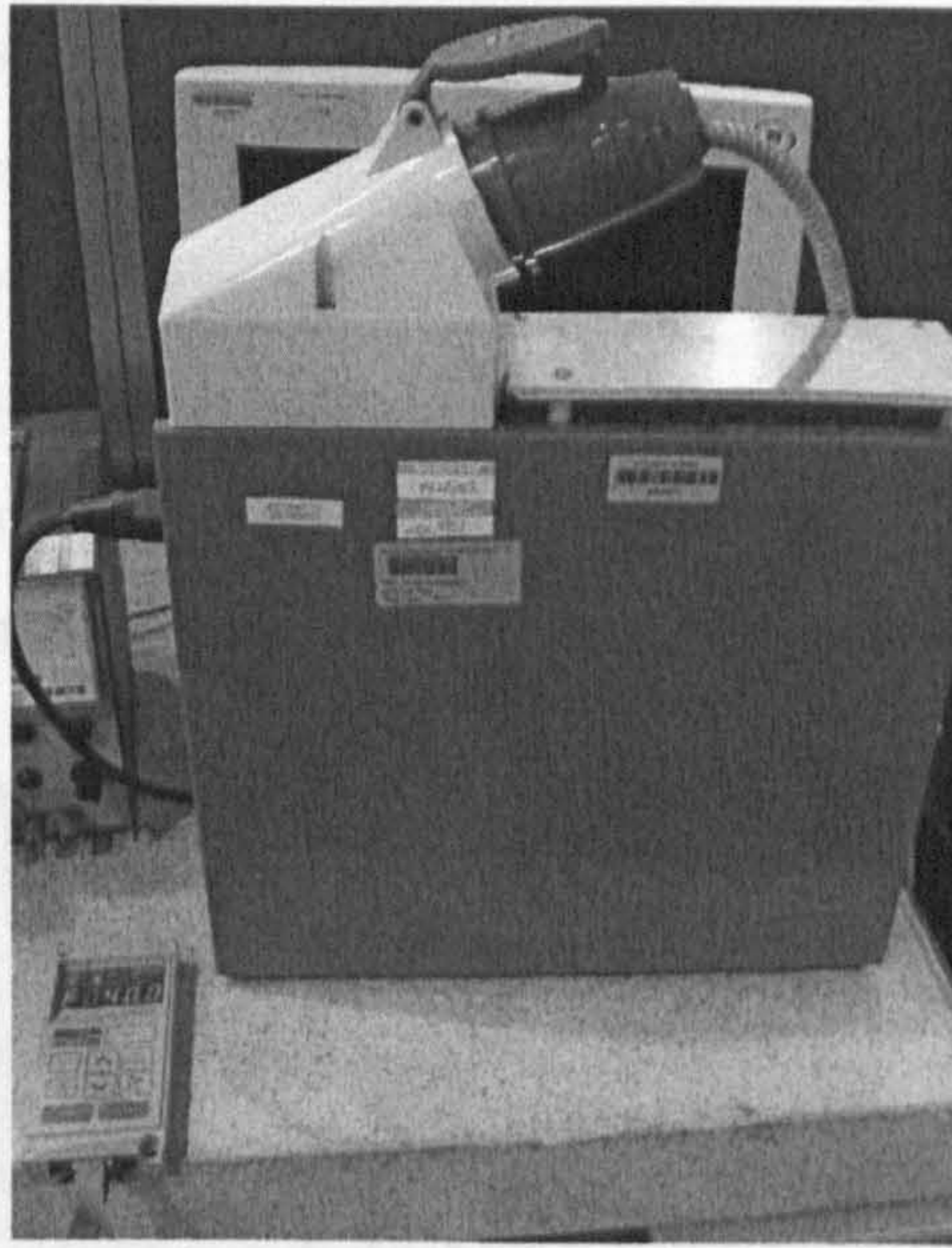
Fig. 5.14. Motor speed controller
