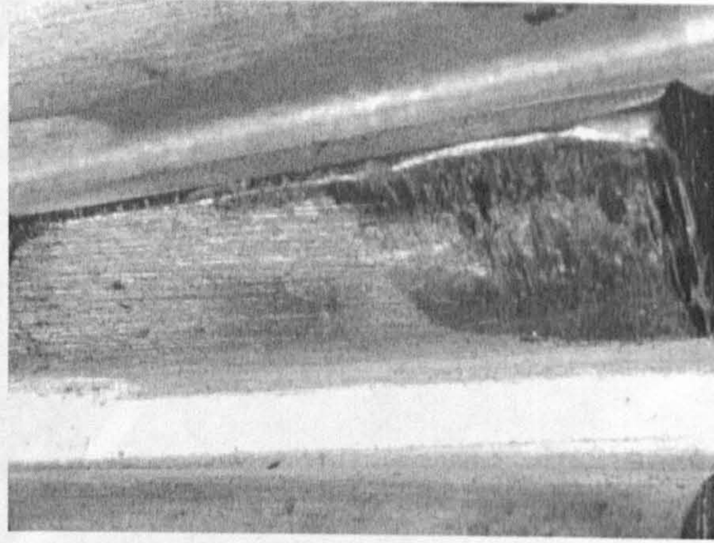
Fig.7.14. Damaged pinion (picture no.3)
