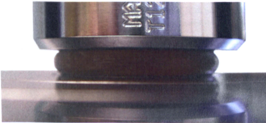
Figure 7.18: Barreling observed during uniaxial compression testing of UR1175.
