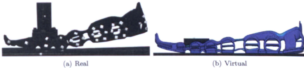
Figure 12.5: Real and virtual Gigaride dynamic forefoot cushion tests at point of maximum tip height (tip is at the posterior for forefoot tests).
