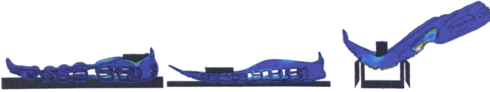
Figure 9.27: The three tests: heel cushion, forefoot cushion and forefoot bend, respectively (mid-sole assemblies shown).
