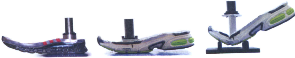
Figure 9.19: The three tests: heel cushion, forefoot cushion and forefoot bend, respectively (production shoes shown).
