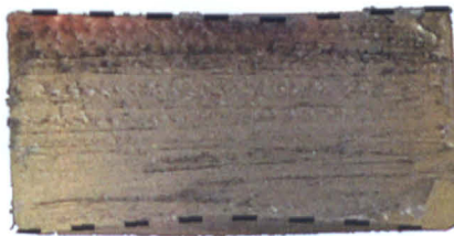
Figure 5.2: View of a compression button cut down the centre. Dashed lines indicate the height of the surface at the cut face.
