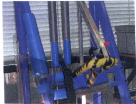
(f) Additional padding to reduce ringing in the frame caused by movement of the clamp on release
