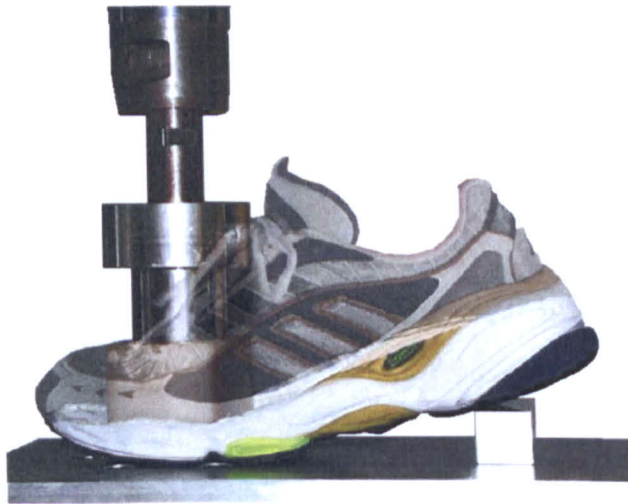
Figure 2.14: Forefoot cushioning test set-up (with optional heel lifting block).
