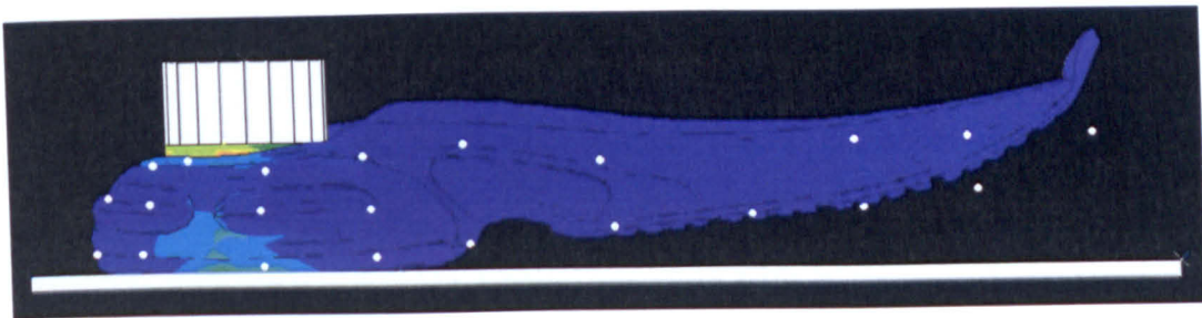
Figure 5.40: Still of a FE result animation, overlaid with pin positions (white) taken from high-speed video. Note that the FE model has rise further than the real, indicating that the front of the FE shoe is moving faster.
