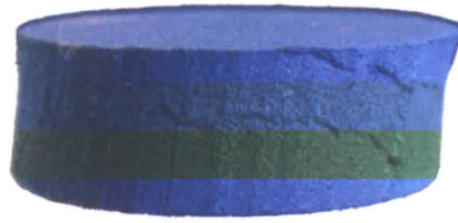
Figure 5.3: Foam compression sample cut with a stamp. Note the non-cylindrical result and rough edges.
