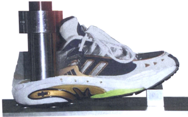
Figure 2.16: Rearfoot cushioning test set-up. The stamp used is 50 mm in diameter, which approximates the dimensions of the calcaneus (see Figure 2.2).
