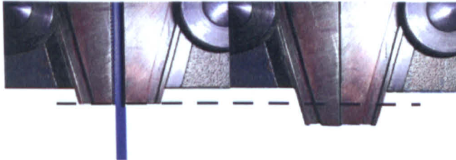
Figure 5.15: Effect of a change in sample thickness caused by contraction. Note the change in effective original length due to clamp movement.
