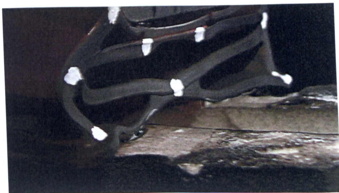
Figure 8.31: De-bonding of a Gigaride heel from its mounting during compression testing (Sample: GRS-3).
