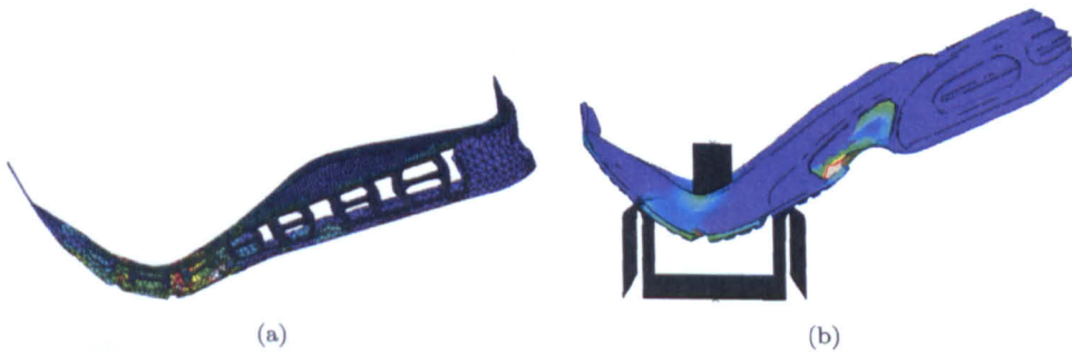
Figure 9.10: Forefoot bend models with: (a) specified boundary conditions with no contact, (b) modelled test equipment with full contact.
