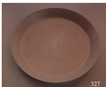
327. Ceramic prototype coated with paint, hand-shaped on pottery wheel.
