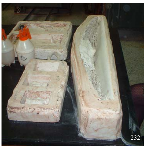
232. Students' work -- Empty refractory moulds after removing clay, ready for loading solid glass, glass workshop, Fine Arts College, Shanghai University. Photo by Xue Lu 2006.
