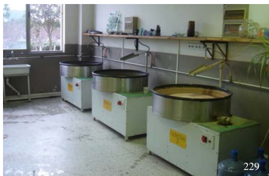
229/230. Cold-processing area: flat bed for grinding and polishing, Glass workshop, Fine Arts College, Shanghai University. Photo by Xue Lu 2006.
