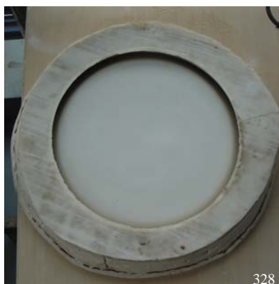
328-330. The gel-flex mould and wax cast from it.
