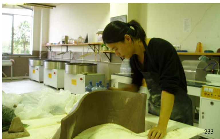
232. Students' work -- Empty refractory moulds after removing clay, ready for loading solid glass, glass workshop, Fine Arts College, Shanghai University. Photo by Xue Lu 2006.
