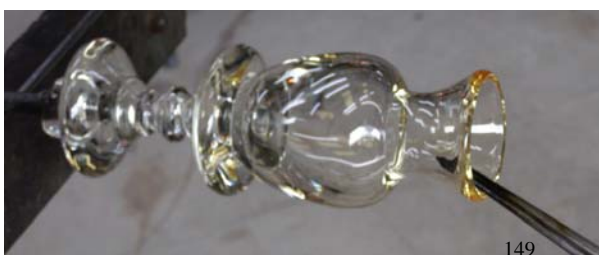
149. Opening up mouth to finish the hot work, then annealing.
