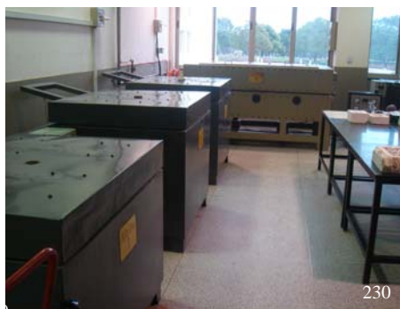
229/230. Cold-processing area: flat bed for grinding and polishing, Glass workshop, Fine Arts College, Shanghai University. Photo by Xue Lu 2006.
