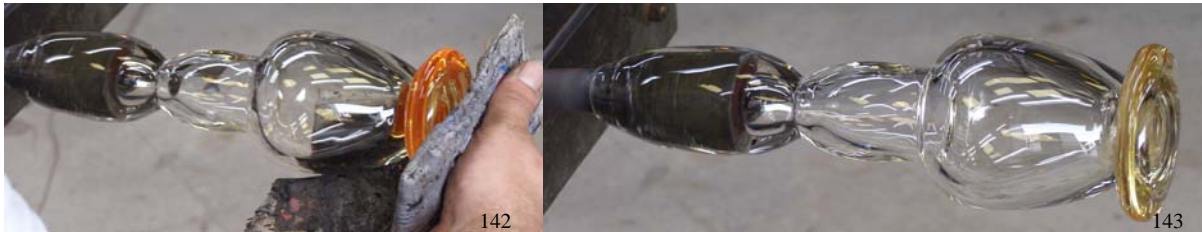
142/143. Adding the first component on the bottom of the cup and shaping by newspaper as a tool.
