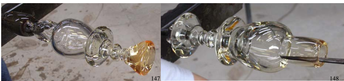
147/148. Adding the base, and shaping into the proper form, then pontiling.
