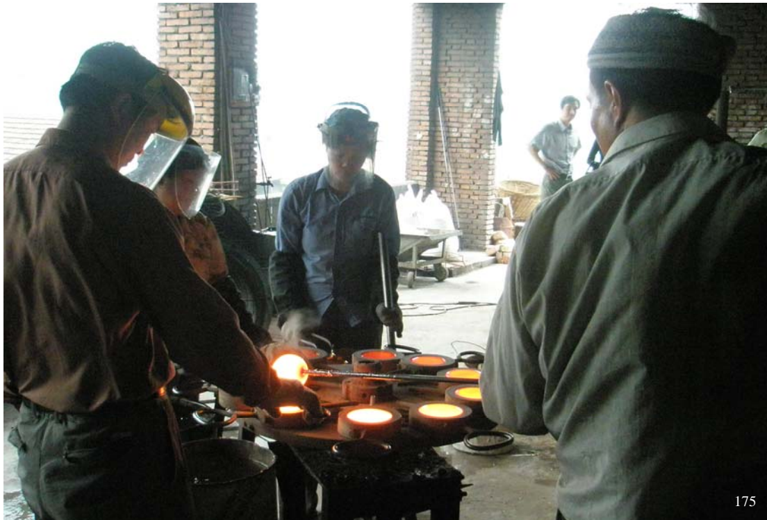
175. Making glass billet by local workers, Wan Li Glass Factory, Chang Shu, China.
