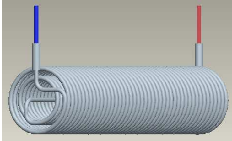
Appendix figure 64 The final design for the heat exchanger showing the coils
