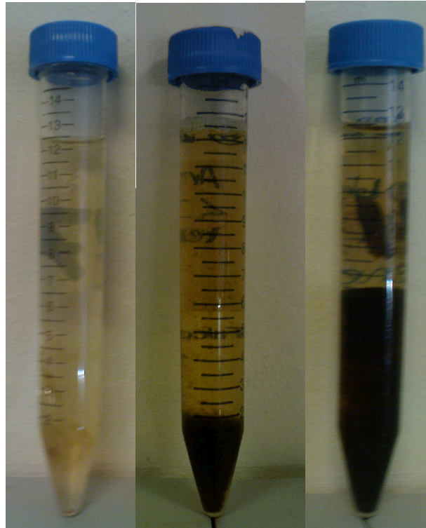
Figure 6.12. Precipitated humic acid fractions for (a) partially composted mixed fish, woodchip and green waste, (b) fully composted MSW (NES) and (c) stabilised green waste (<25 mm).
