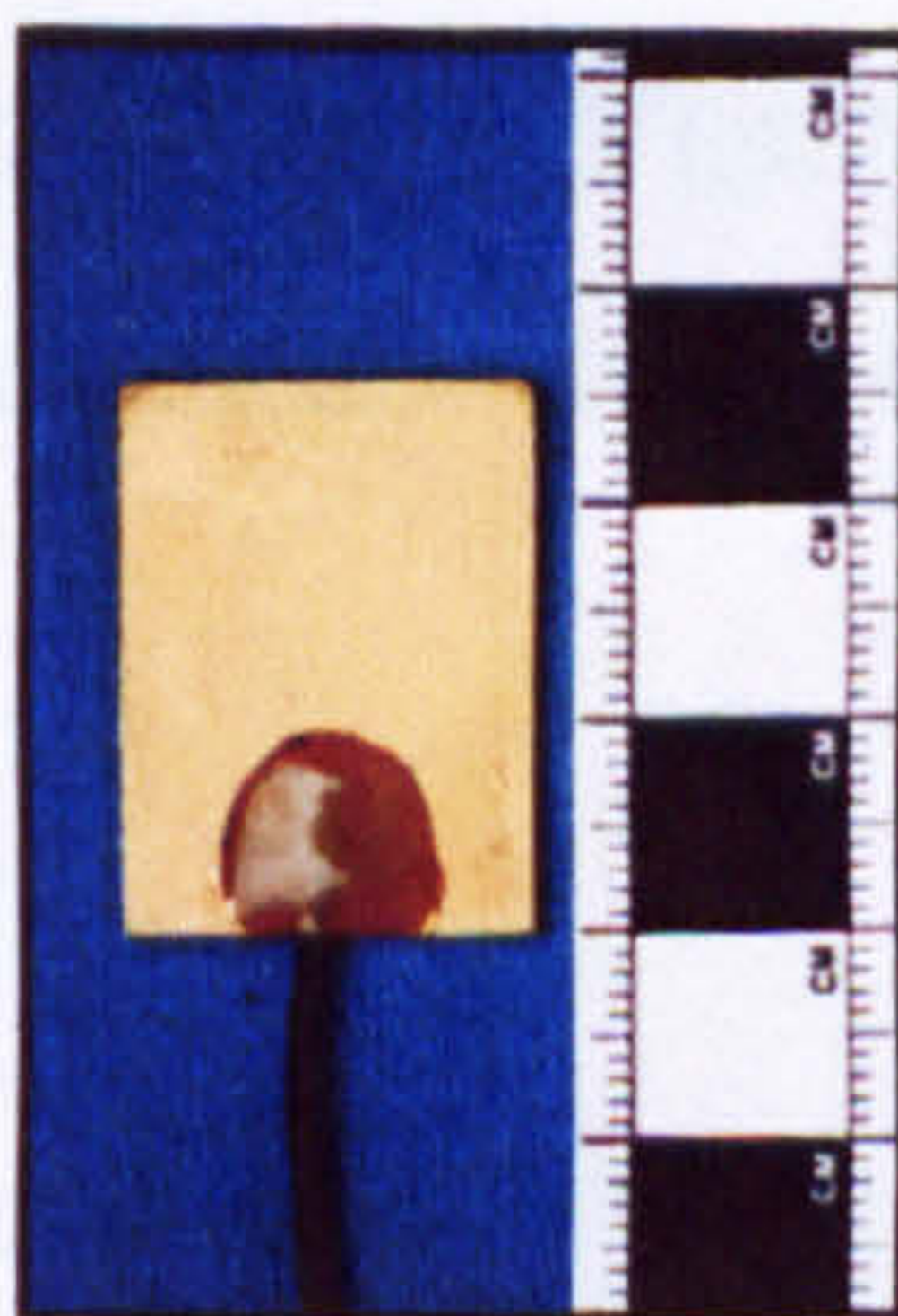
Figure 3.15: Gold sputter coated glass slide electrode
