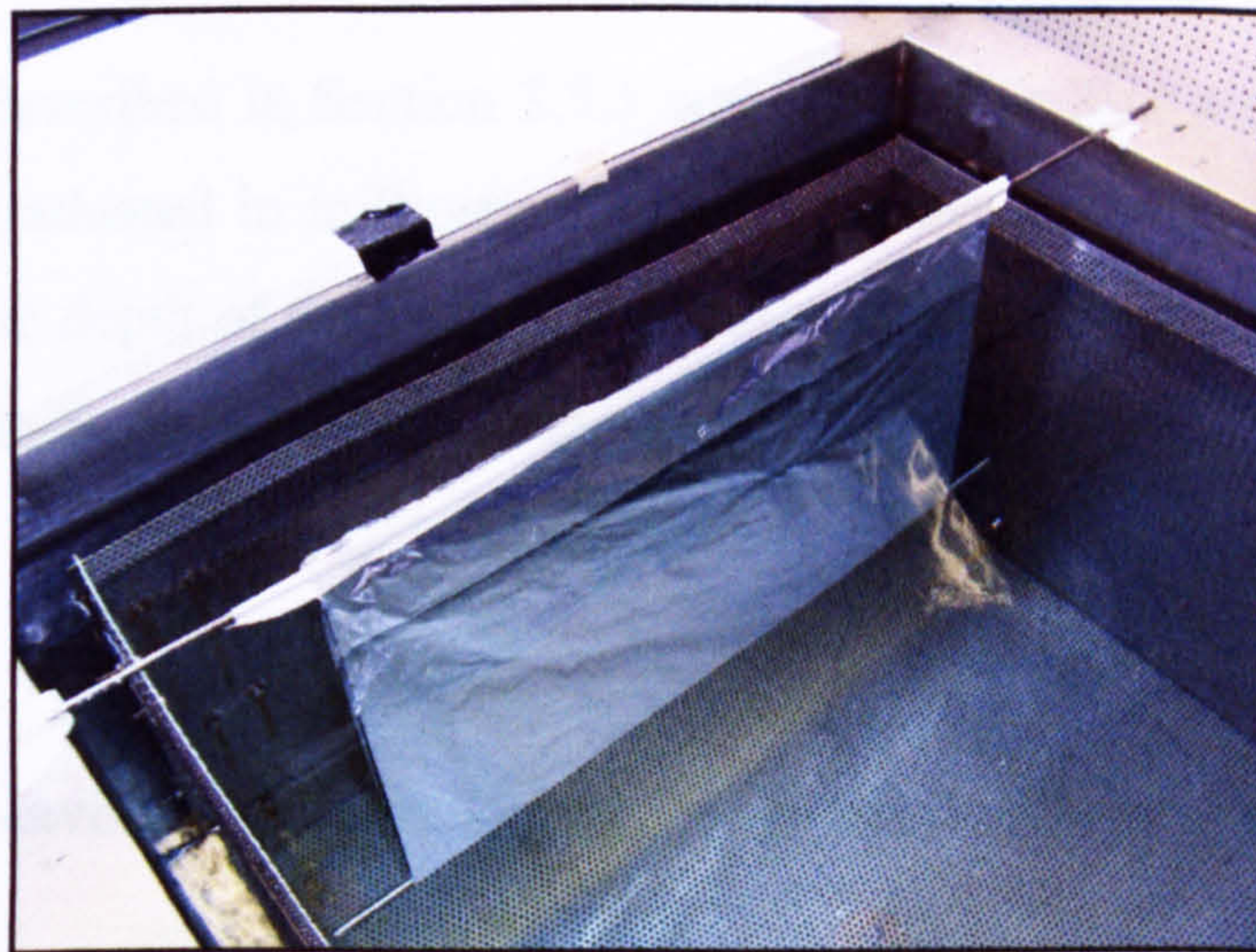
Figure 3.18: Vertical suspension of foil sheet for cavitation profiling
