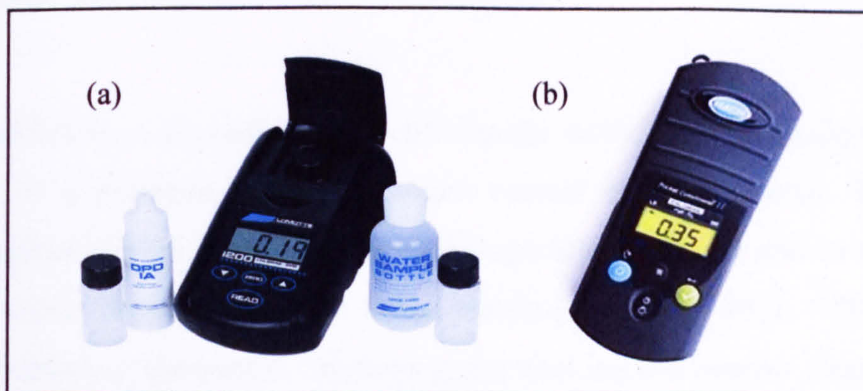
Figure 2.47: (a) the LaMotte™ and (b) Hach™ chlorine analyzer pocket colourimeter kits
