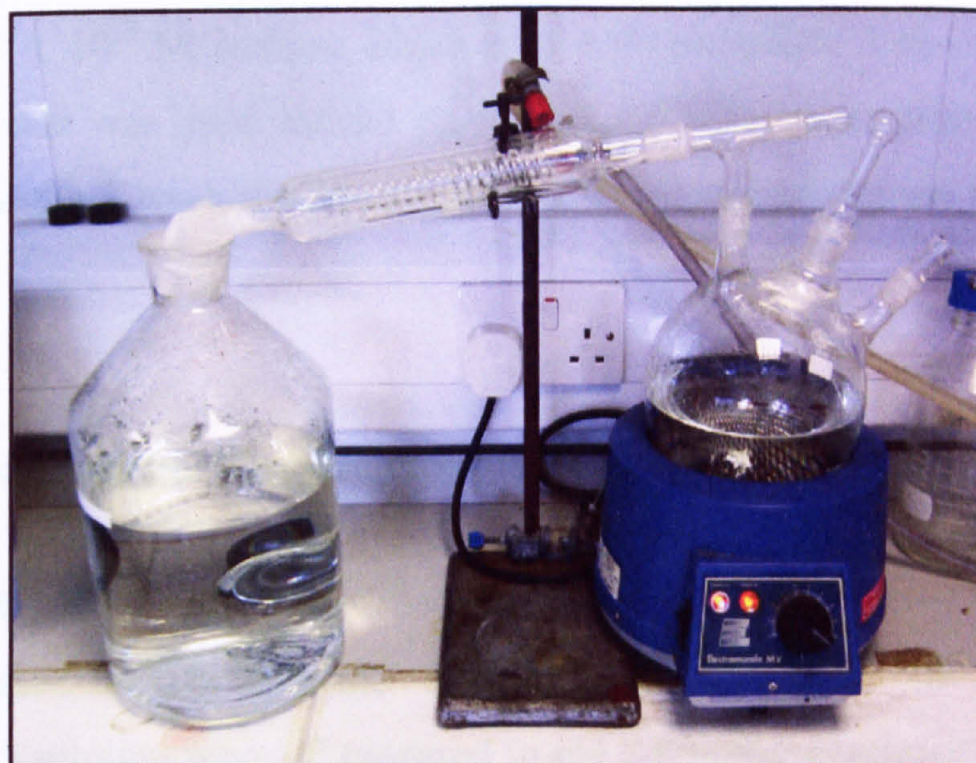
Figure 3.14: Water distillation set up
