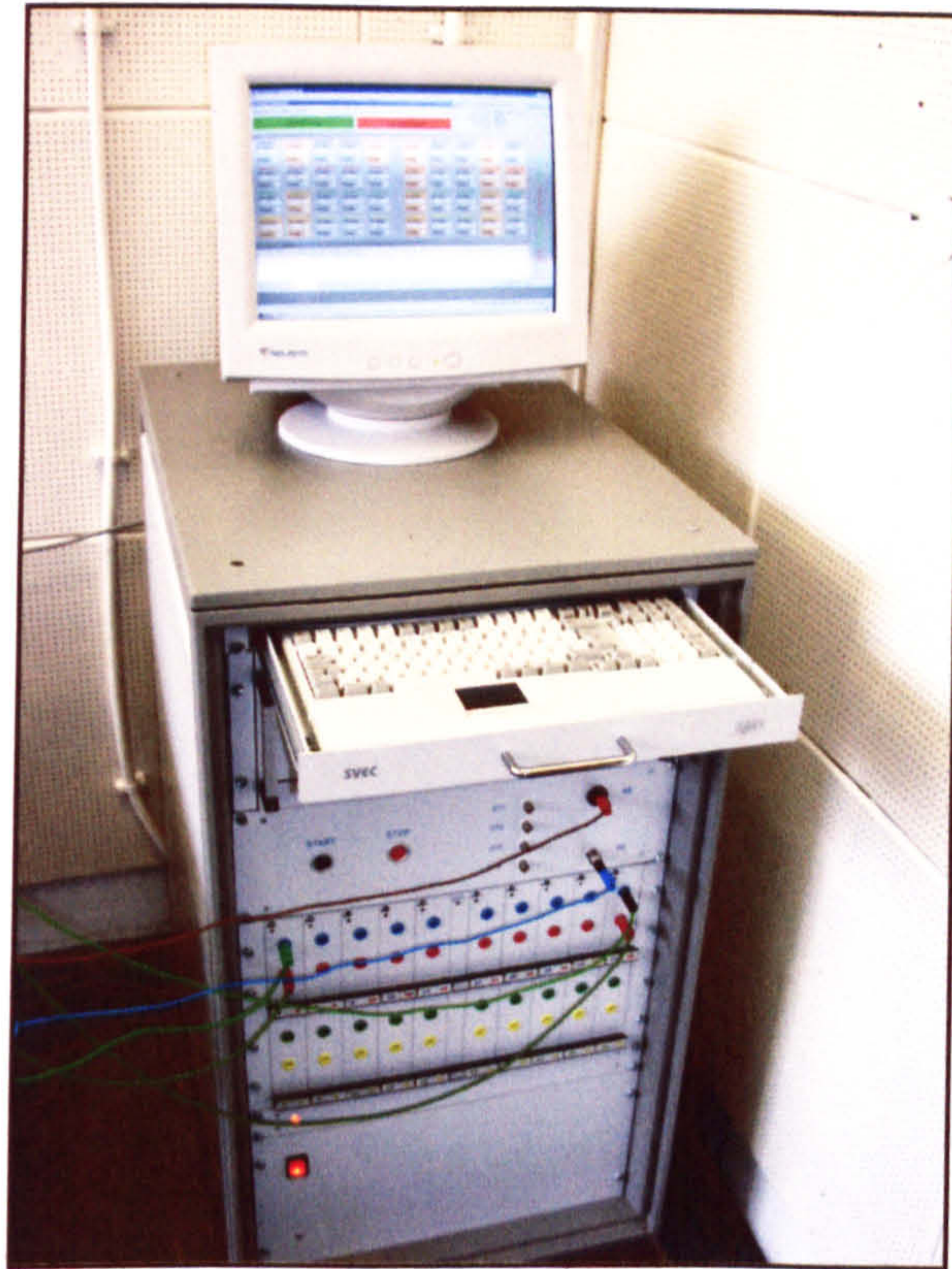
Figure 5.30: Microarray Limited custom built 40-channel industrial potentiostat
