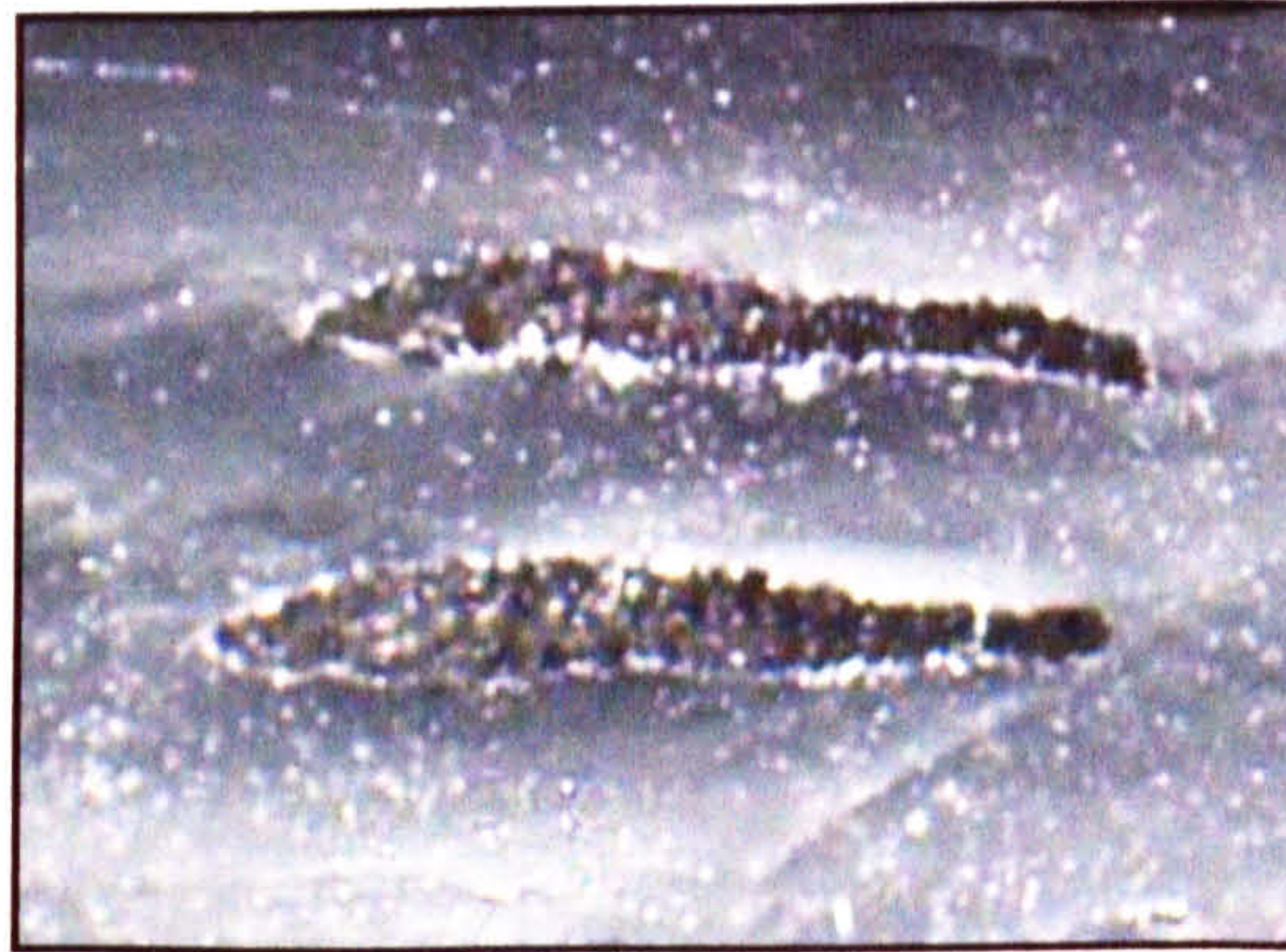
Figure 6.20: Coalescence of pin holes to form large voids in the foil sheet
