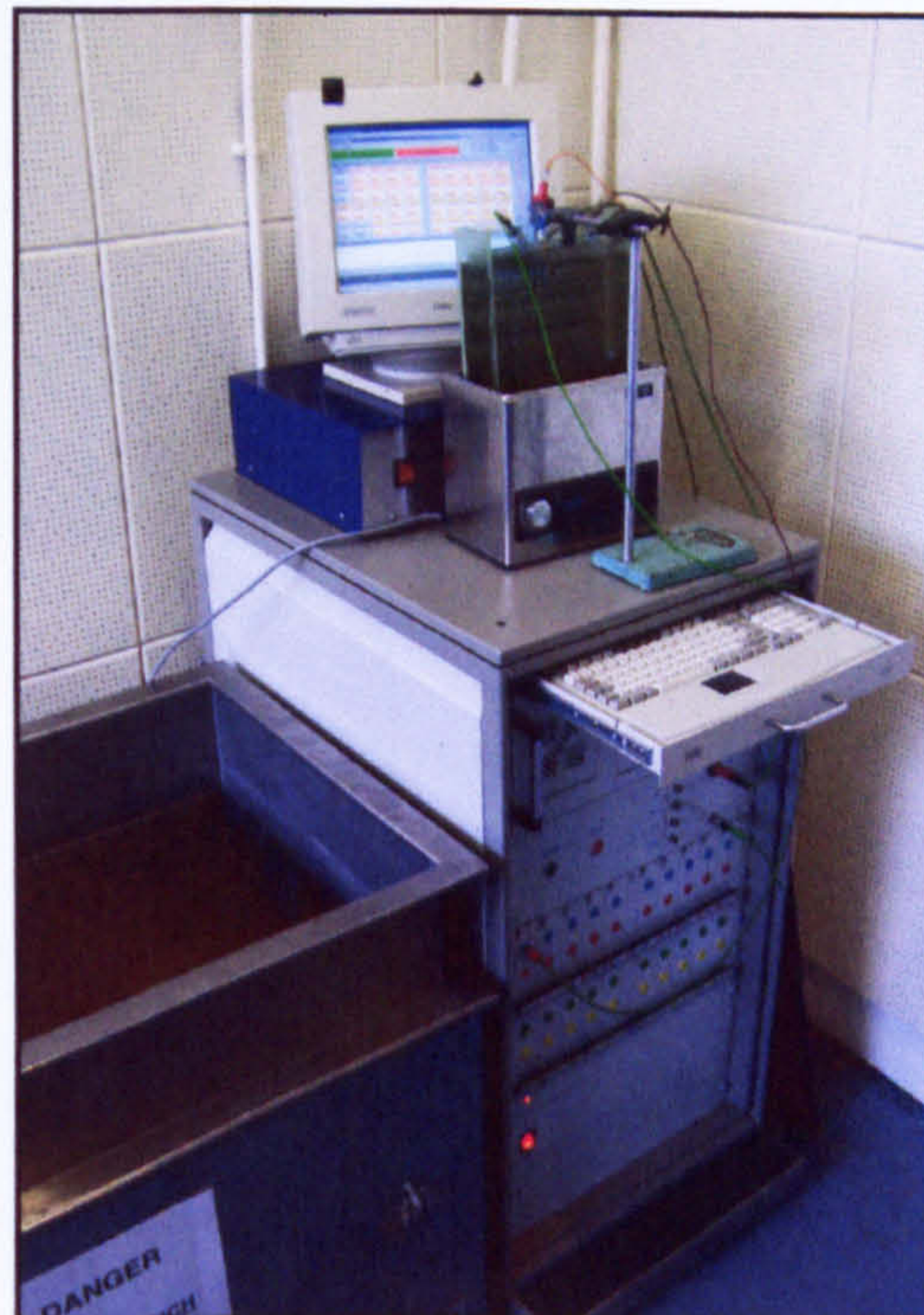
Figure 3.7: Sycopel multi-channel potentiostat
