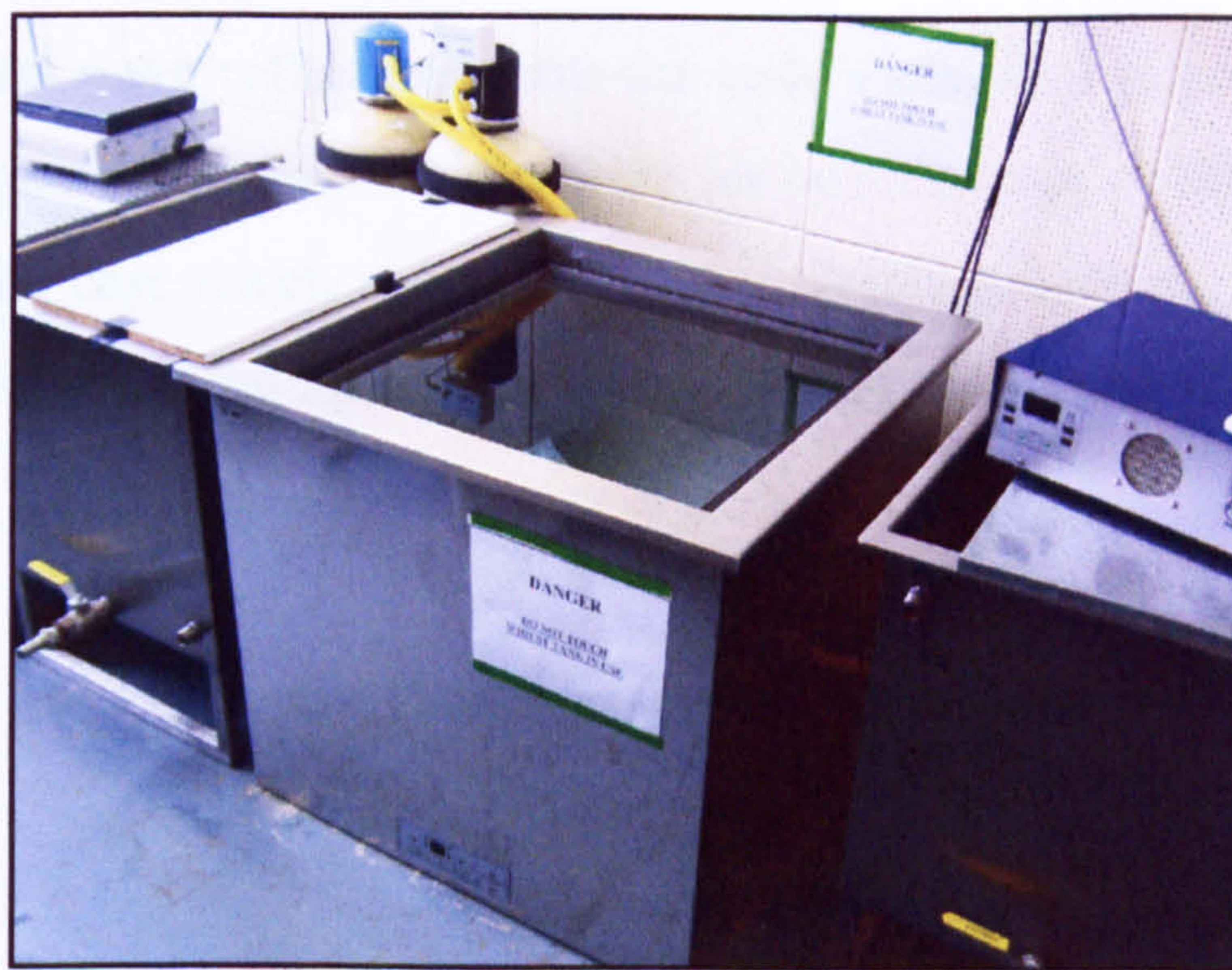
Figure 3.8: Custom built 2kW ultrasound tank
