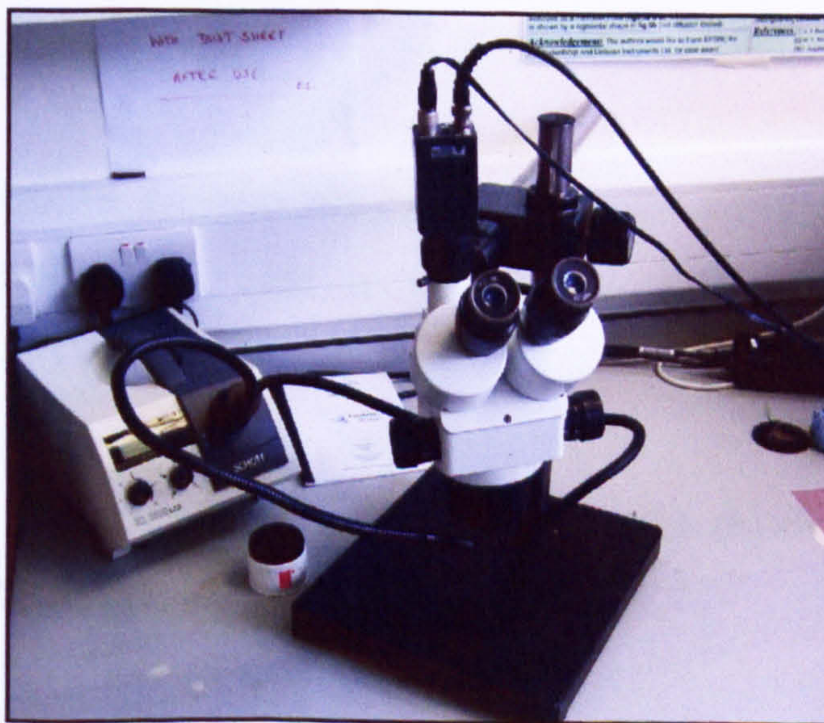
Figure 3.11: Olympus SZX12 microscope with Schott KL1500 light source
