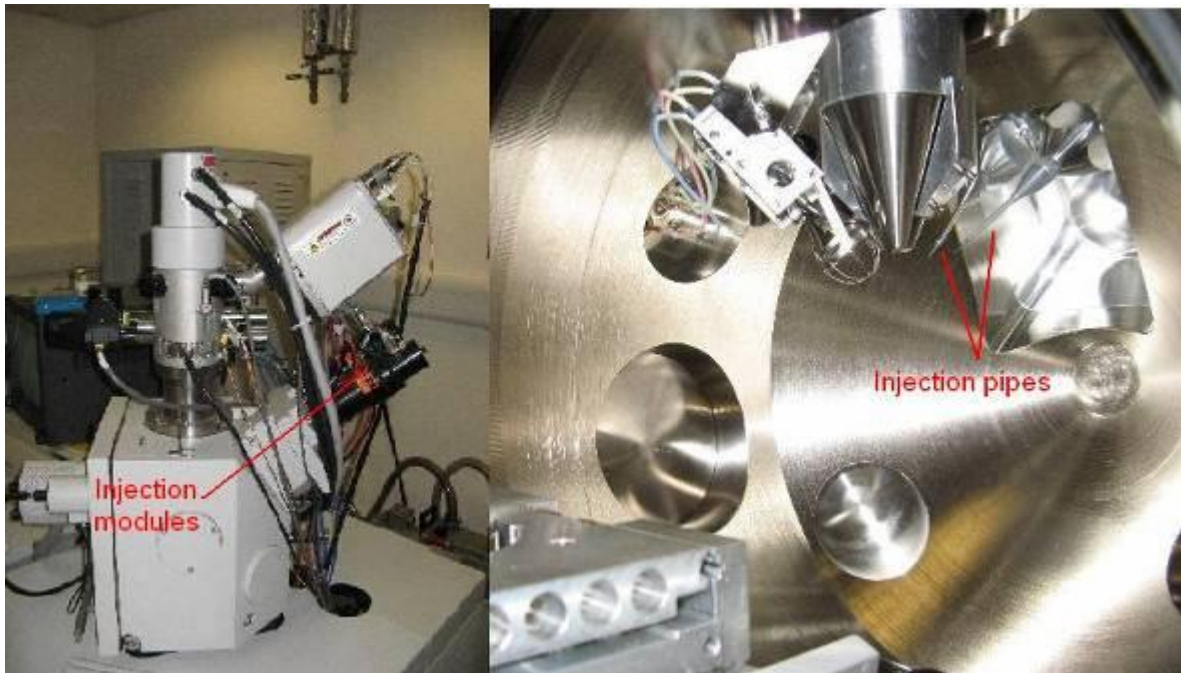
Figure 3.4 – FEI FIB 200 chamber gas injection system
