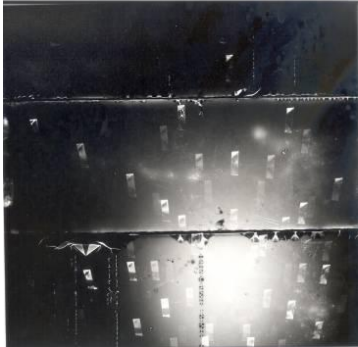
Figure 7.6 – Nuclear plate reflection image, 0.1x1.7mm beam through smaller side face of the diamond
