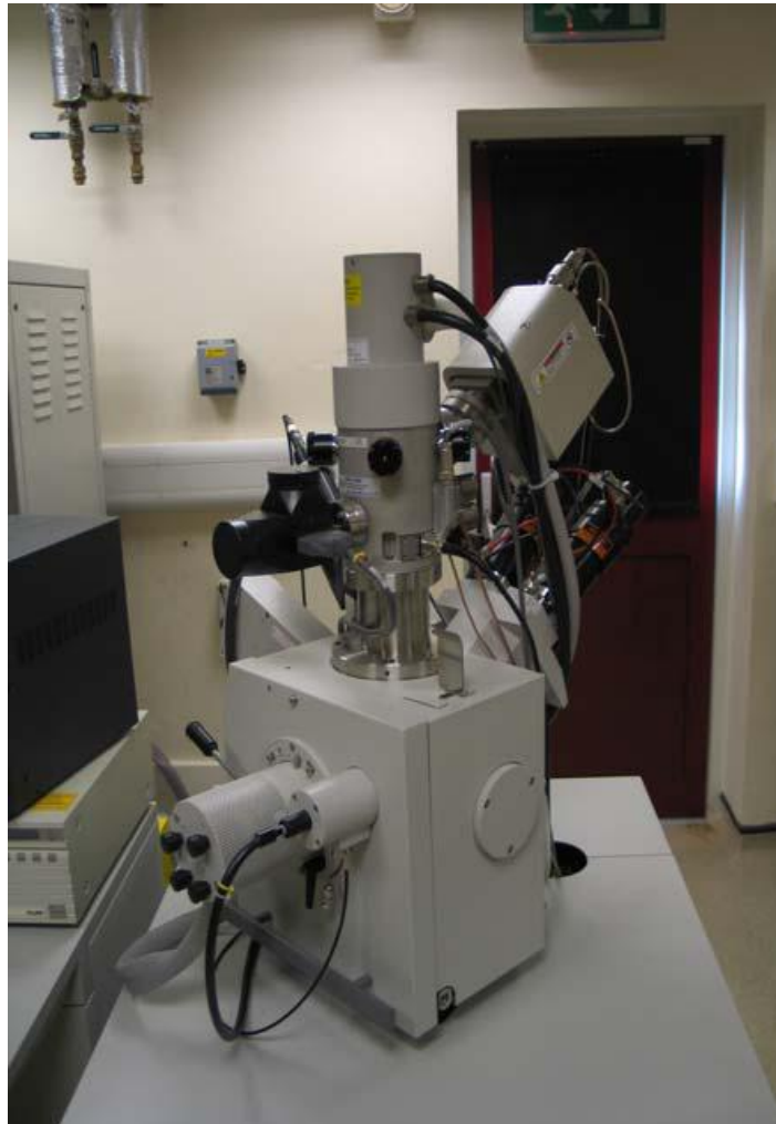
Figure 4.1 – A FEI 200 FIB system
