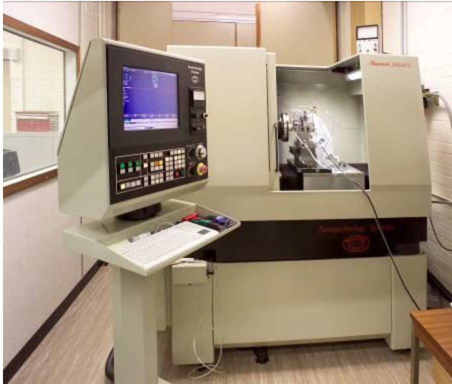
Figure 4.5 – A Moore Nanotech 350 UPL diamond turning machine
