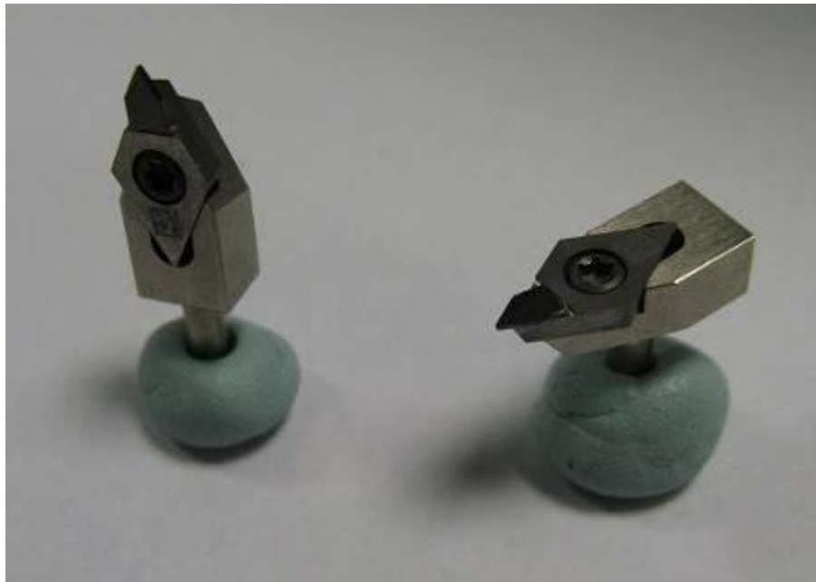
Figure 4.3 – CVD tool blanks in the horizontal and vertical holders
