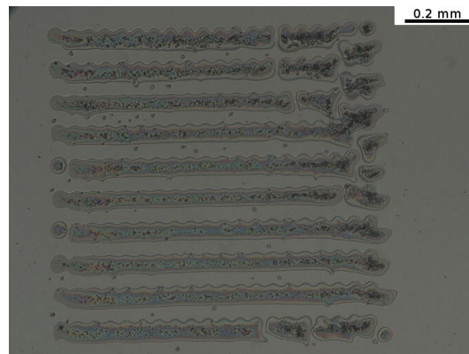
Figure 6.19: Optical micrograph of the 20x20 dots pattern printed with PZT ink MS1 under the following conditions: voltage 30 V, CPH 0.30 mm, 4 nozzles.
