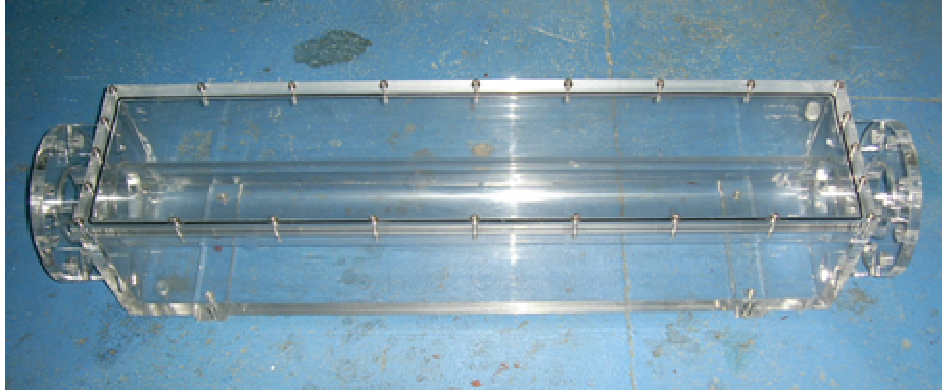
Figure 6-2: Perspex box used to reduce unwanted reflected light
