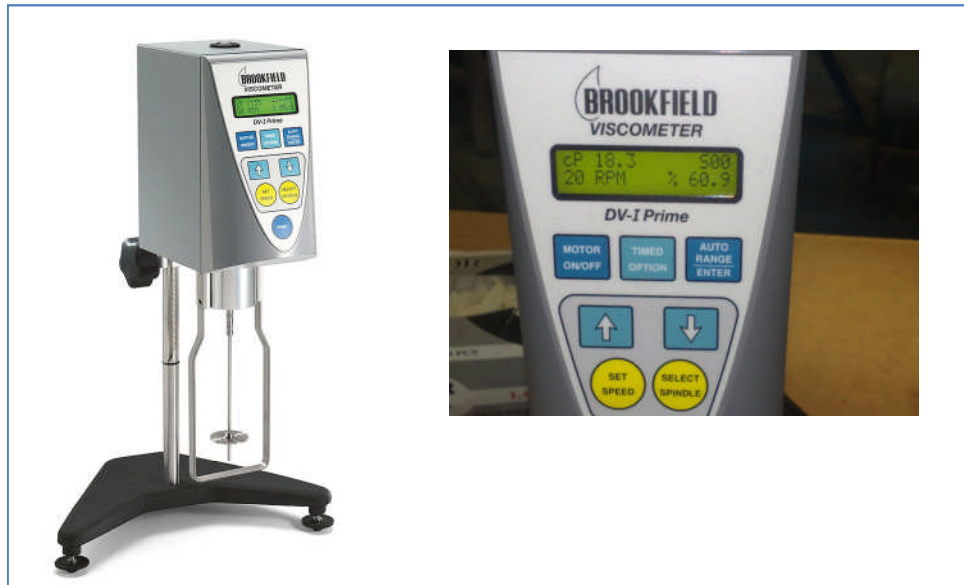
Figure 6-5: Rotational BROOKFIELD viscometer
