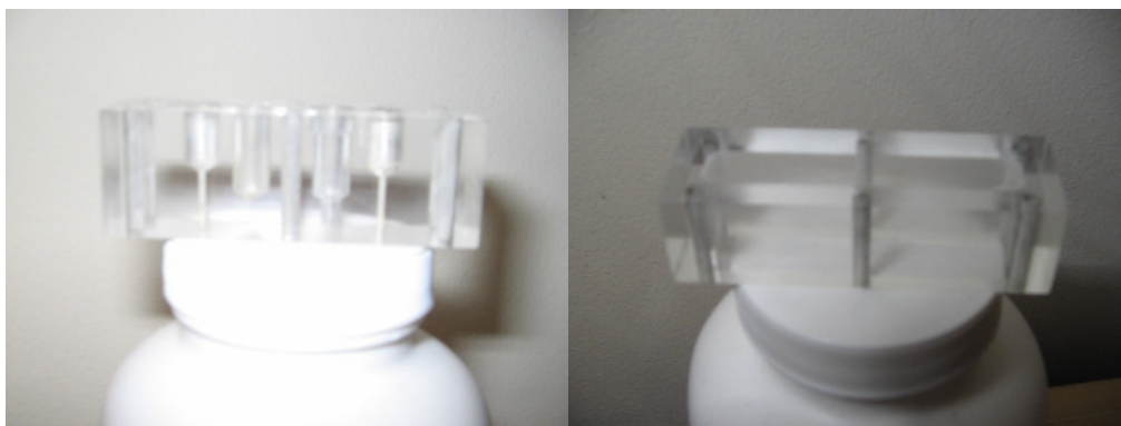
Figure 5.3 Photographs of the two machined Perspex blocks that will be sandwiching the fluidic channel.
