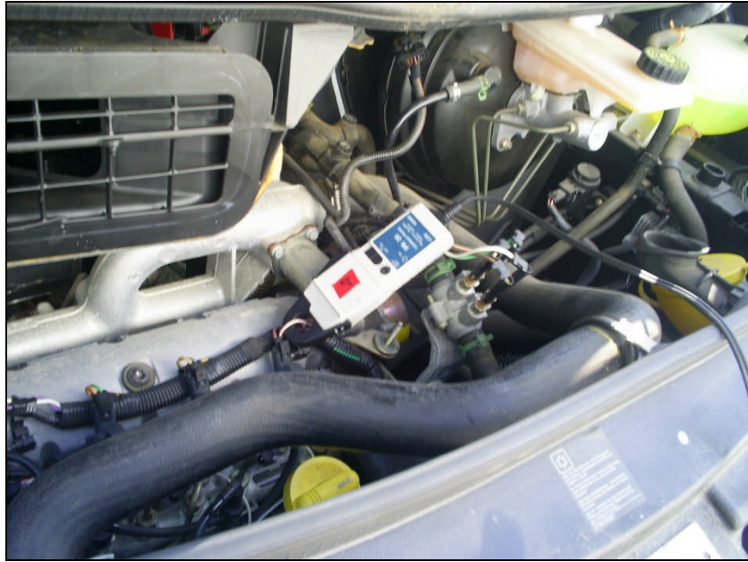
Figure 4.9 Vauxhall Vivaro injector currents measured with current probes
