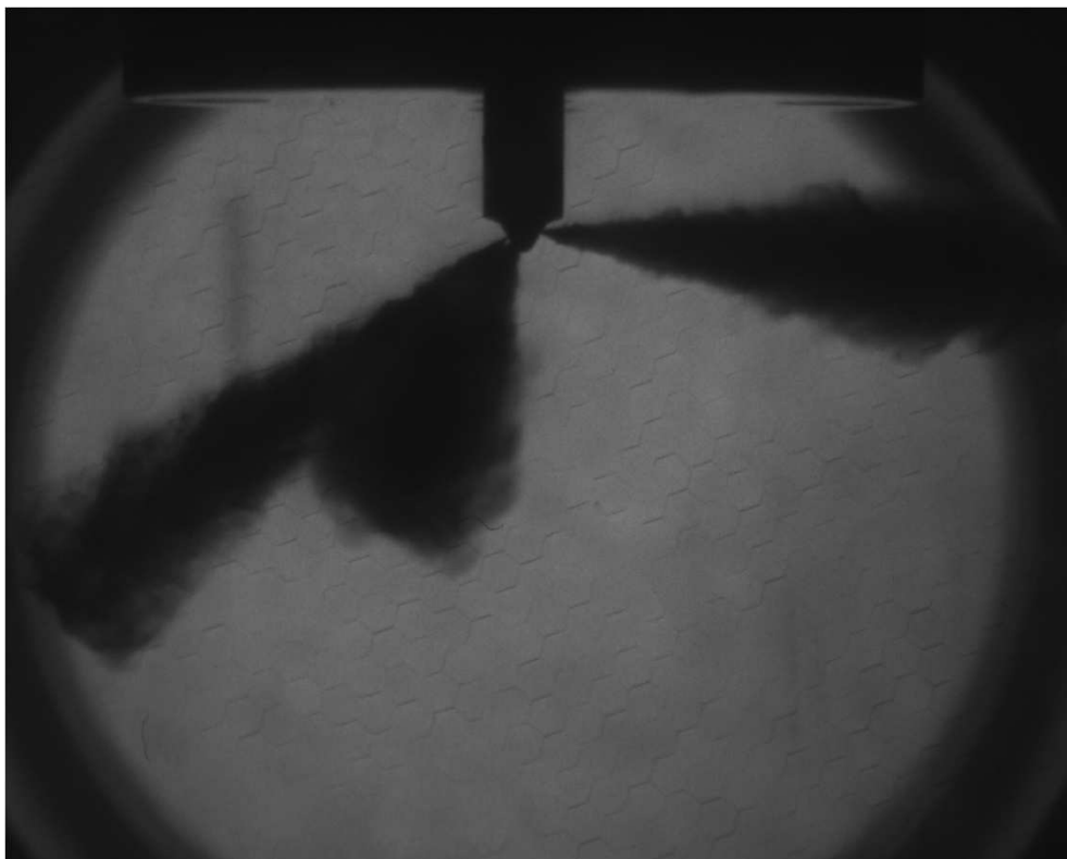
Figure 4.35 Injector plume 1, bomb pressure: 40bar, fuel pressure 1500bar, time: 1.5ms
