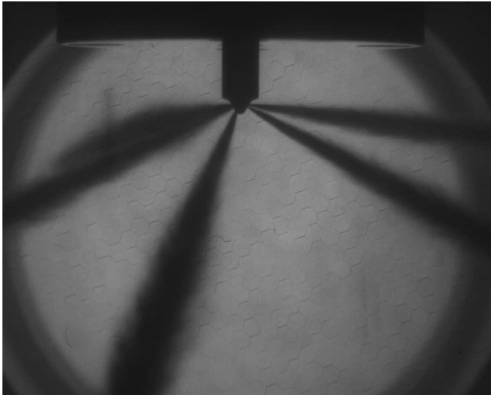
Figure 4.42 Injector plume 2, bomb pressure: atmospheric, fuel pressure 1500bar, time: 0.9ms
