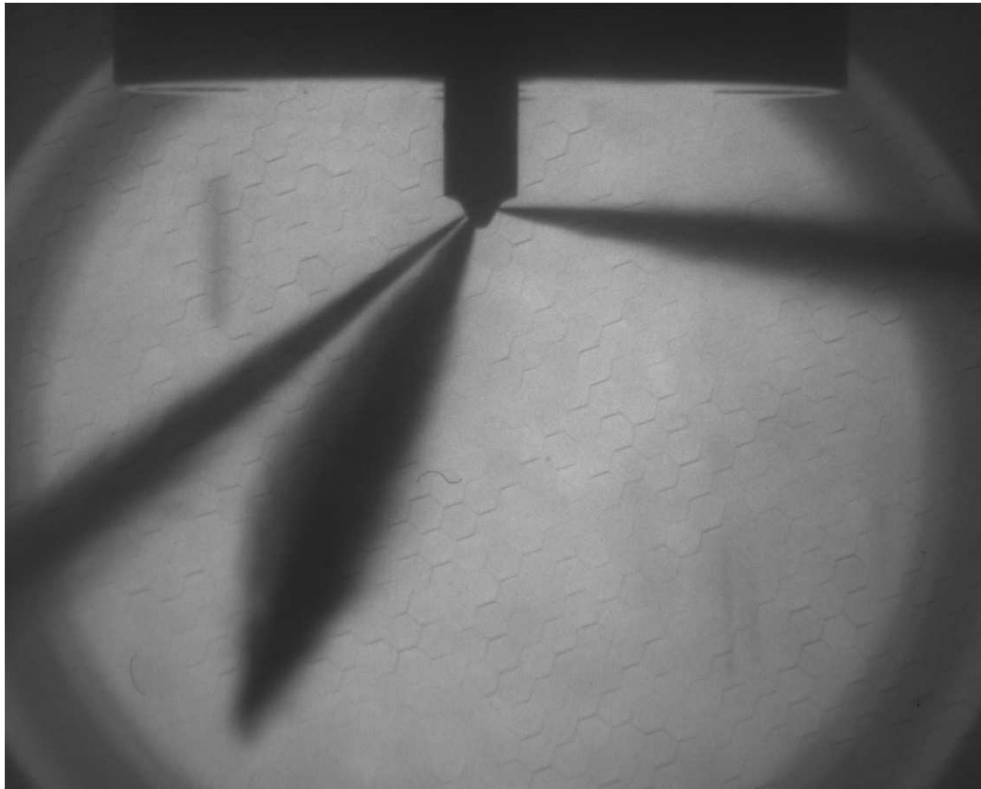
Figure 4.28 Injector plume 1, bomb pressure: atmospheric, fuel pressure 1500bar, time: 0.8ms
