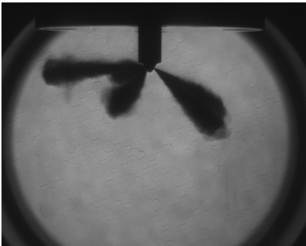
Figure 4.47 Injector plume 3, bomb pressure: 40bar, fuel pressure 1500bar, time: 0.8ms
