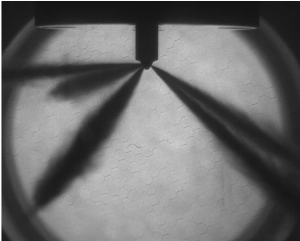
Figure 4.46 Injector plume 3, bomb pressure: atmospheric, fuel pressure 1500bar, time: 0.8ms
