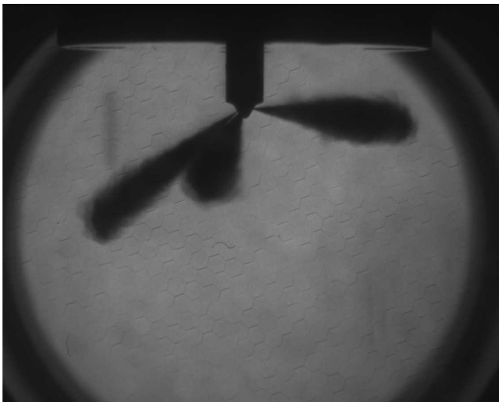
Figure 4.31 Injector plume 1, bomb pressure: 40bar, fuel pressure 1500bar, time: 0.9ms
