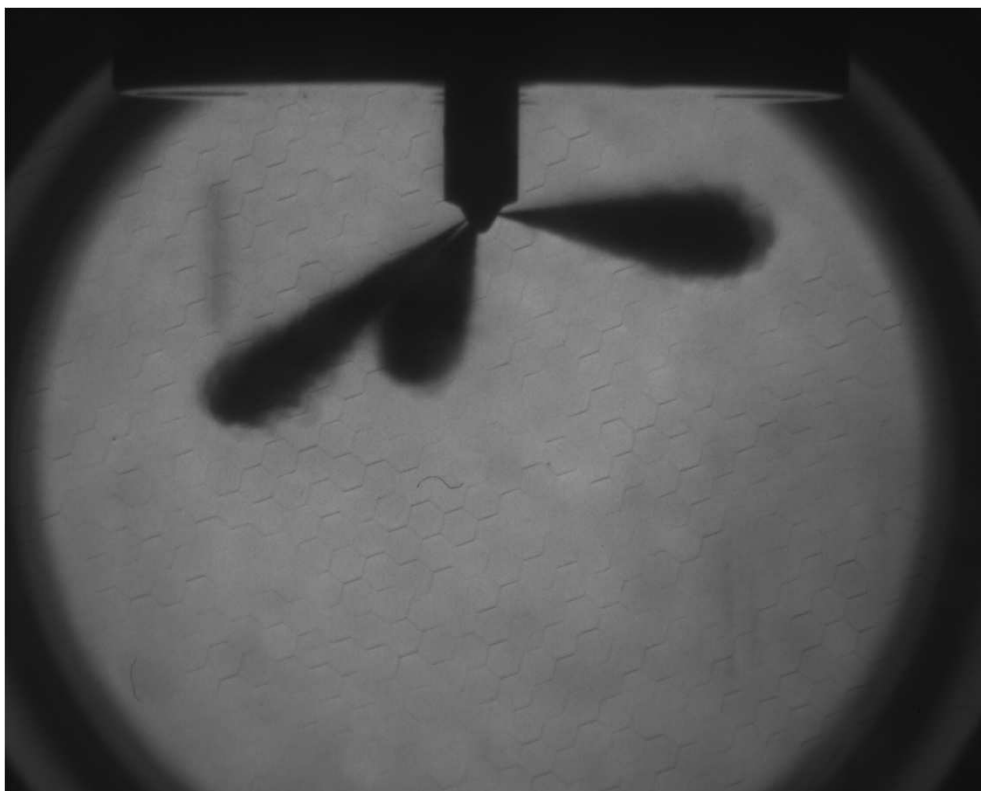
Figure 4.29 Injector plume 1, bomb pressure: 40bar, fuel pressure 1500bar, time: 0.8ms
