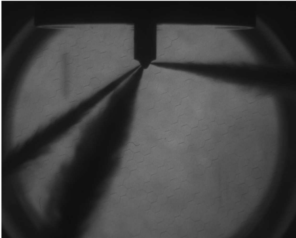
Figure 4.32 Injector plume 1, bomb pressure: atmospheric, fuel pressure 1500bar, time: 1ms
