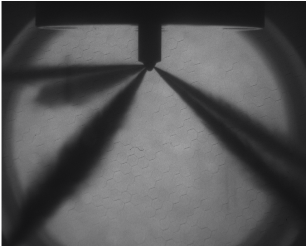
Figure 4.48 Injector plume 3, bomb pressure: atmospheric, fuel pressure 1500bar, time: 0.9ms
