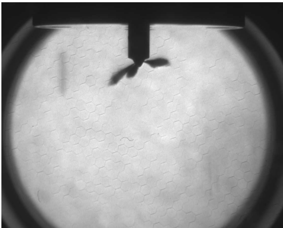
Figure 4.27 Injector plume 1, bomb pressure: 40bar, fuel pressure 1500bar, time: 0.5ms
