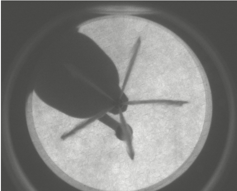
Figure 4.20 Spray image from the below after 2ms from the injection signal. Bomb pressure: atmospheric, fuel pressure 1500bar
