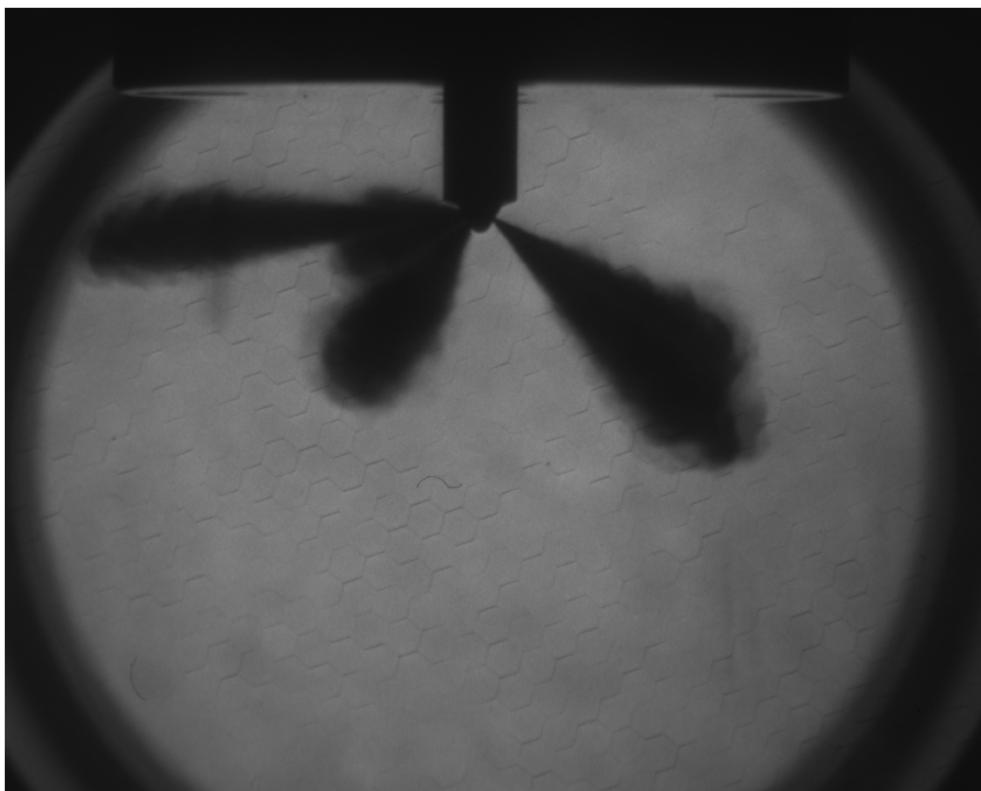
Figure 4.49 Injector plume 3, bomb pressure: 40bar, fuel pressure 1500bar, time: 0.9ms
