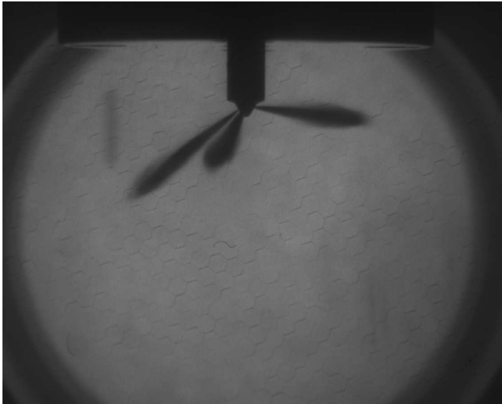
Figure 4.26 Injector plume 1, bomb pressure: atmospheric, fuel pressure 1500bar, time: 0.5ms
