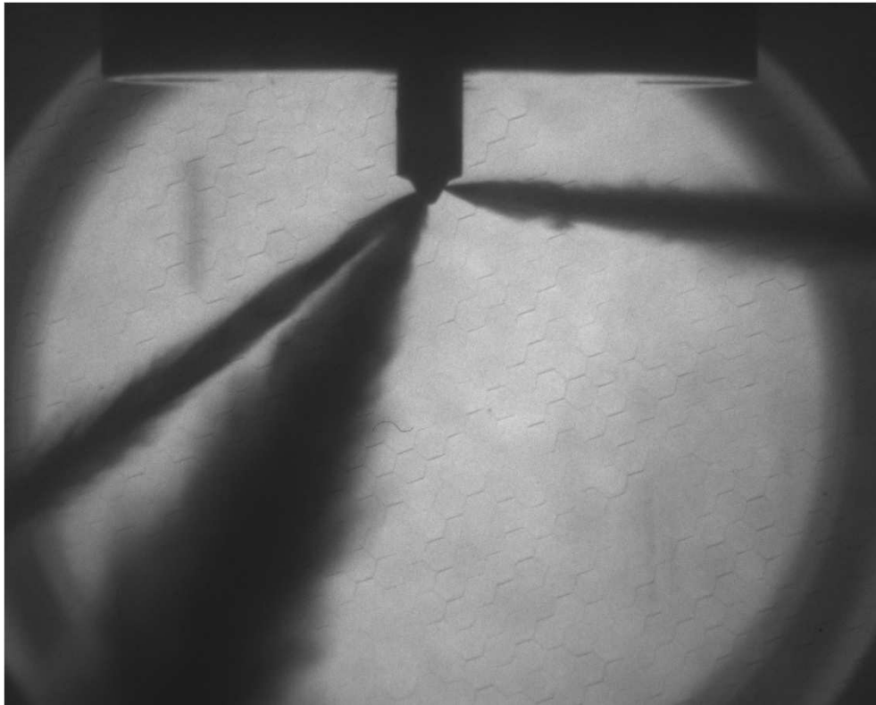
Figure 4.34 Injector plume 1, bomb pressure: atmospheric, fuel pressure 1500bar, time: 1.5ms
