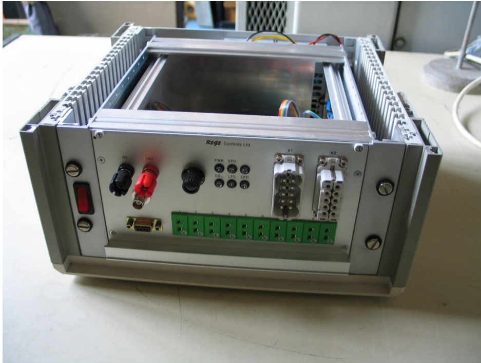
Figure 4.13 R2G2 diesel ECM (electronic control module)
