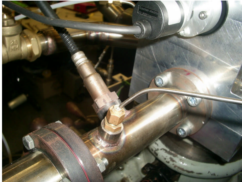
Figure 4.88 Bosch LSU wide band \lambda sensor
