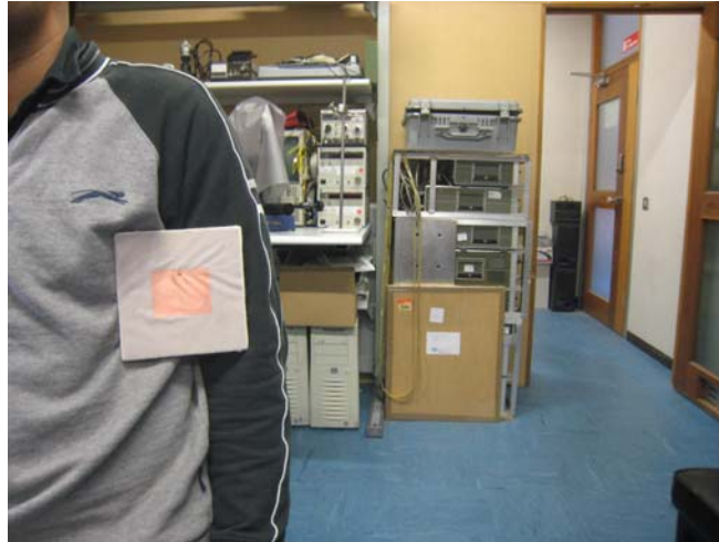
Figure 6-17 Measurement setup for HIS integrated wearable patch antenna.
