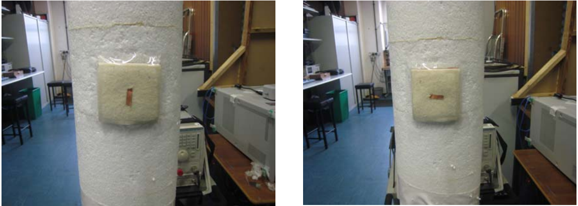
Figure 6-1 Measurement setup for bending condition. (a) H-plane bending, (b) E-plane bending
