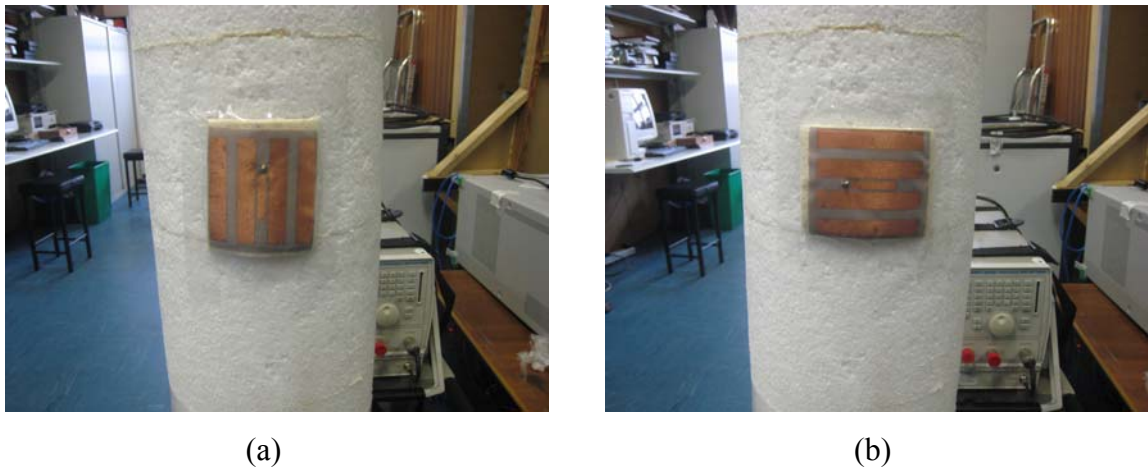
Figure 6-8 Measurement setup for HIS integrated inverted L wearable antenna. (a) E-plane bending, (b) H-plane bending.
