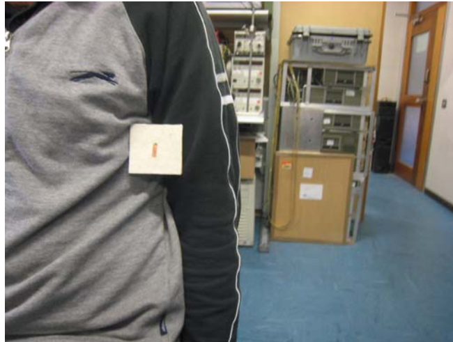
Figure 6-3 Measurement setup for on body effect on input match behaviour of inverted L over HIS wearable antenna.
