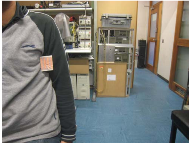
Figure 6-10 Measurement setup for on body test of wearable inverted L antenna integrated with HIS.
