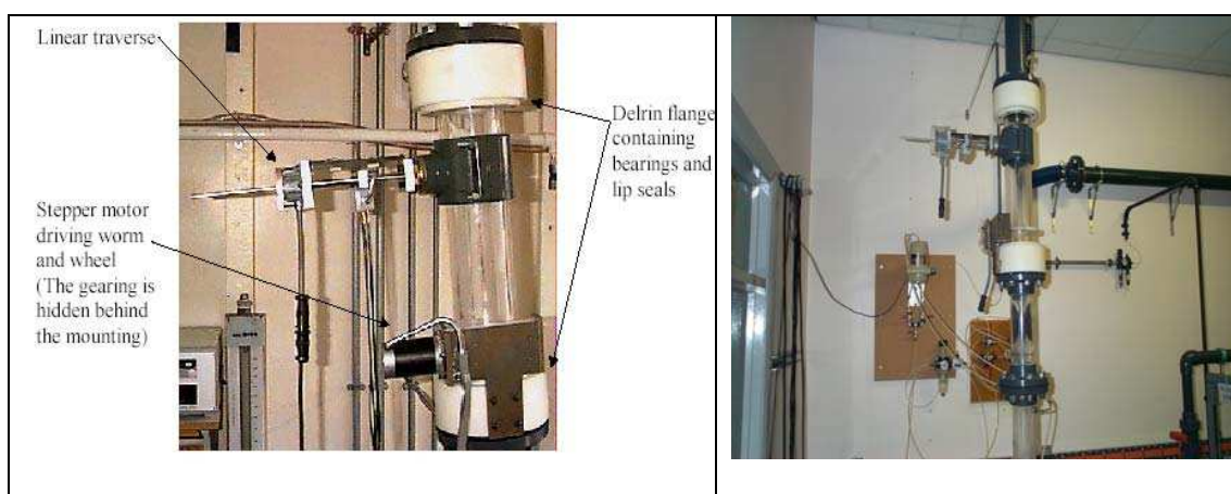
Figure 29. The traverse mechanism in the air water loop[14], and in the oil-water loop with the swirler just upstream of it (right).
