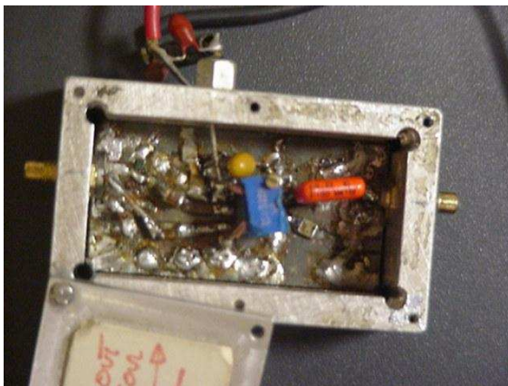
Photos H: Transmitter Filter (up), Receiver Filter (down)
