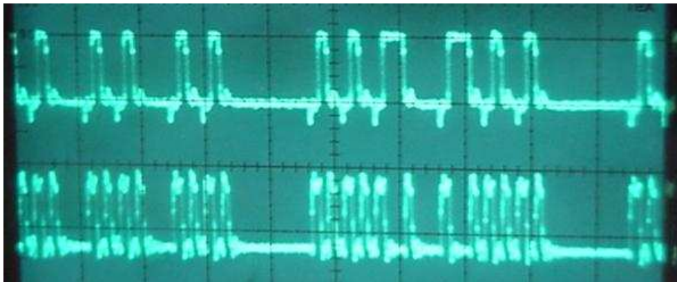
Fig. 8.14: FPGA: PRBS PCM output sequence (top trace), PRBS DiPPM input sequence (bottom trace)
