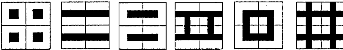
Figure 5.3 Generic urban forms, based on Martin and March (1972) From left to right: pavilions, terraces, slabs, terrace-courts, pavilion-courts and courts (Ratti et al 2003)
