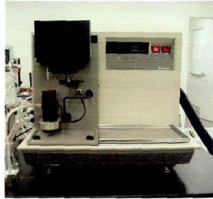
Figure 3-2 – Schematic of a TGA measurement apparatus (left) and picture of TA Instruments 2950 TGA.
