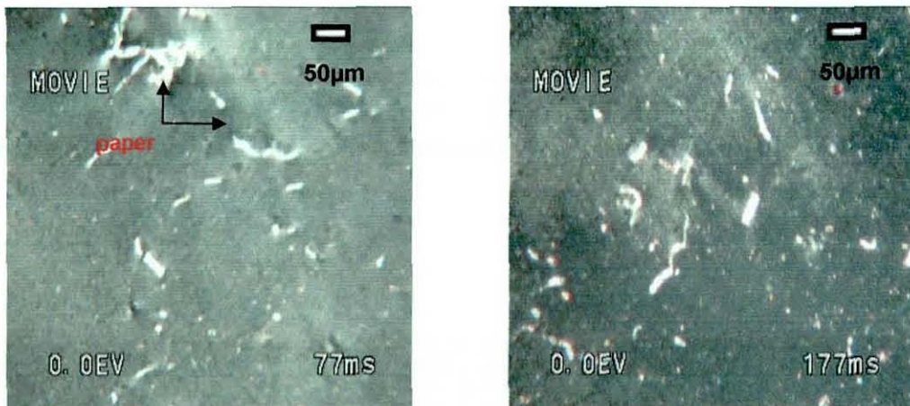
Figure 4-3 – Contaminants in recycled polymer (PR-LD3) under polarized light (x 160)
