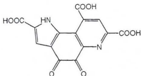
Figure 3.8. Molecular structural unit of the PQQ organic binder unit.
