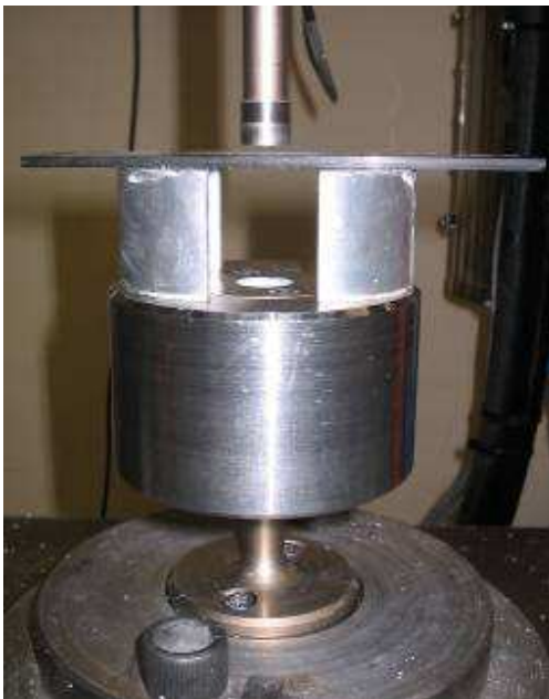
Fig. 4.10 Removal of the die using the top punch and aluminium supports.
