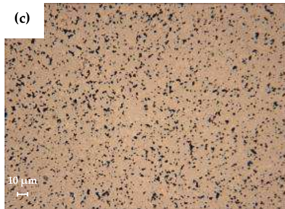
Fig. 5.76 Optical micrographs of WC-10Co-1VC pressureless sintered at 1390°C/60 min after (a) 60 min, (b) 180 min, and (c) 300 min.
