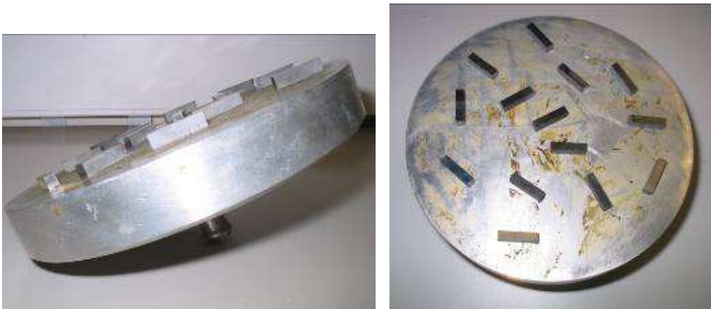
Fig. 4.20 Sintered TRS samples secured onto a grinding/polishing disc.
