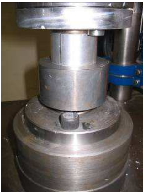
Fig. 4.13 Spacers used to push the die off the bottom punch.
