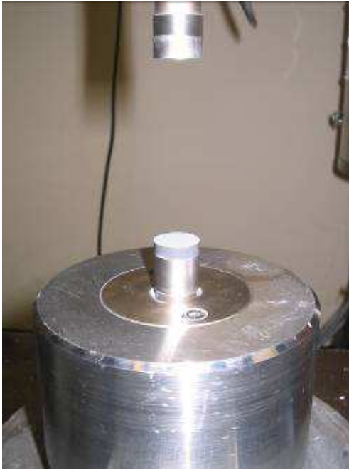
Fig. 4.11 Compacted sample after retraction of the top punch and die.
