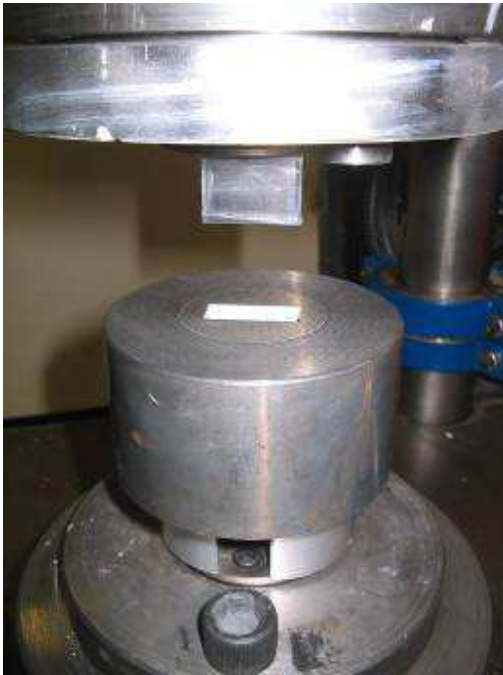
Fig. 4.12 Assembly arrangement of the punches and die showing the starting position of the top punch for rectangular compacts.
