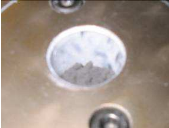
Fig. 4.8 Powder mass poured into the lubricated cylindrical die.
