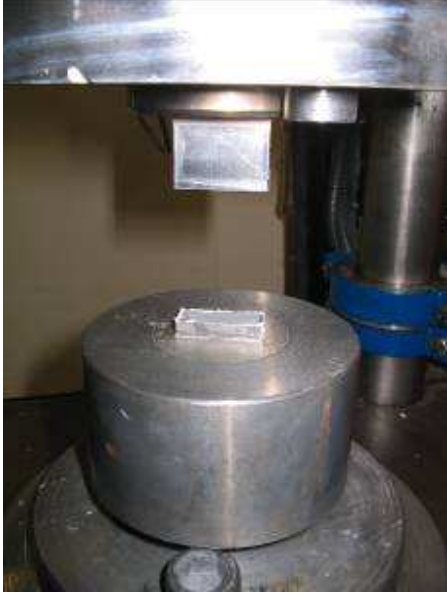
Fig. 4.14 Top punch fully retracted leaving easy access to the compacted sample.
