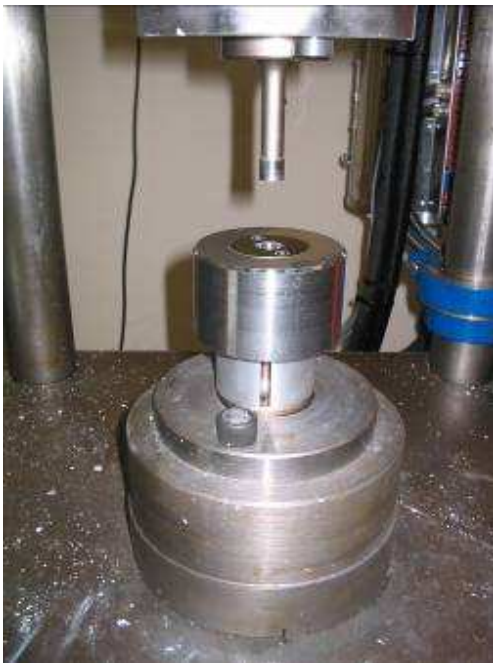
Fig. 4.9 Assembly arrangement of the punches and die showing the starting position of the top punch.
