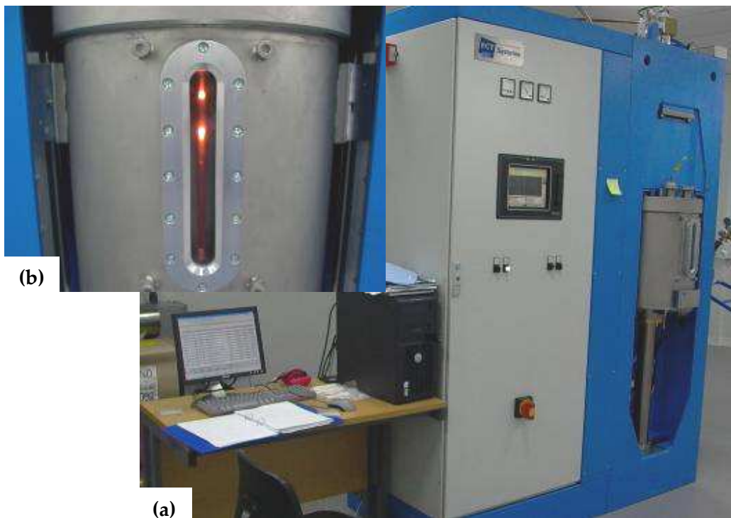
Fig. 4.16 SPS facility (a) used to consolidate the hardmetal powders, with (b) a spark plasma reaction shown in the furnace. (Pictures courtesy of the School of Engineering and Materials Science, Queen Mary, University of London).
