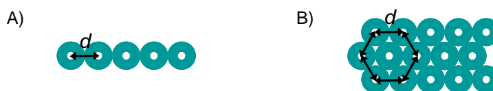
Figure 5.3. Schematic representation of cylinders in A) a lamellar packing (1D growth) and B) a hexagonal packing (2D growth).
