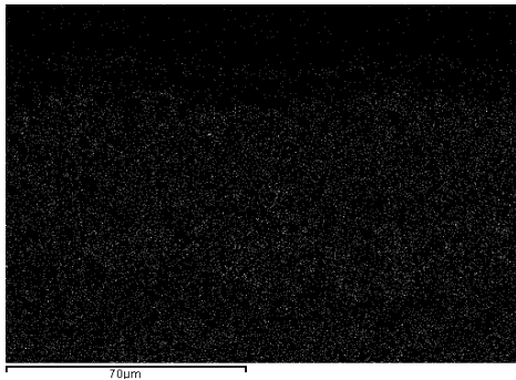
Figure 10.70: IN738LC sample IN2/3; after 500 hours corrosion testing at 900°C – element maps
