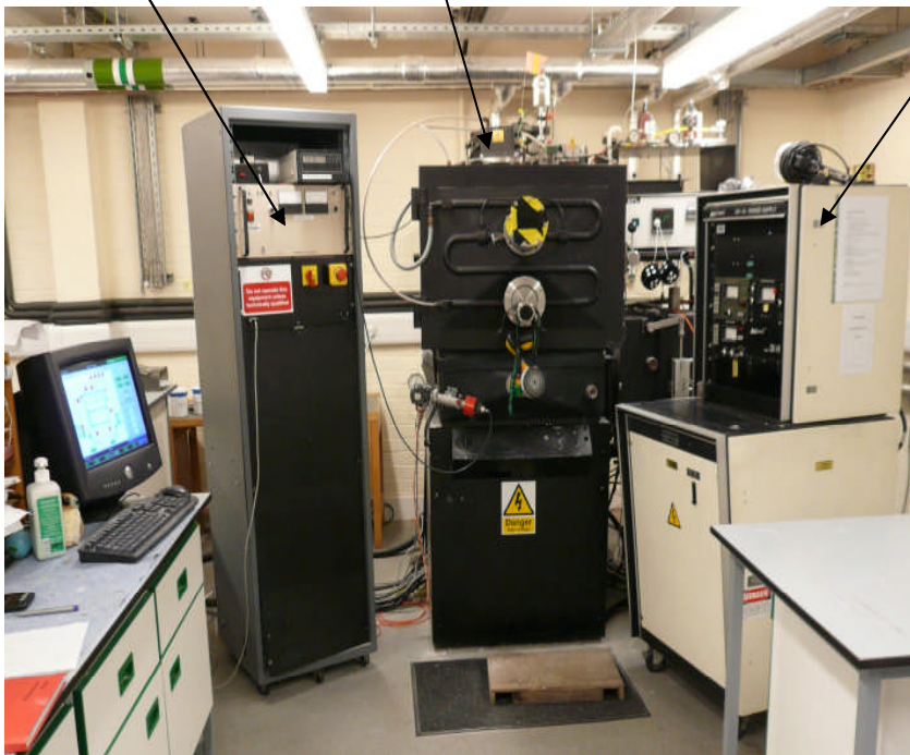
Figure 4.10: Electrotech 680 EB-PVD equipment for TBC deposition
