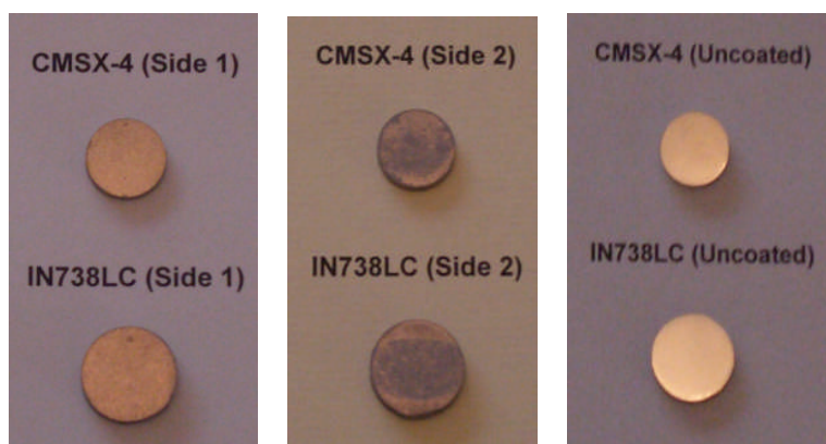
Figure 8.24: IN738LC and CMSX-4 samples after silicon-aluminising CVD for 1h at 800°C
