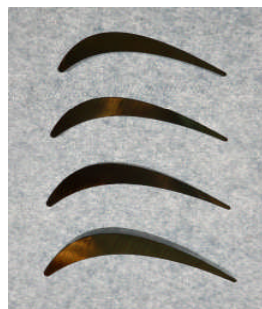
(a) Post EB-PVD Sections ready for mounting
