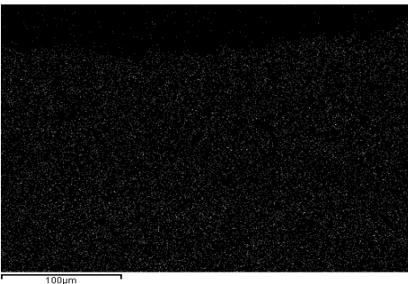
Figure 10.67: IN738LC sample IN1/9; after 500 hours corrosion testing at 900°C – element maps
