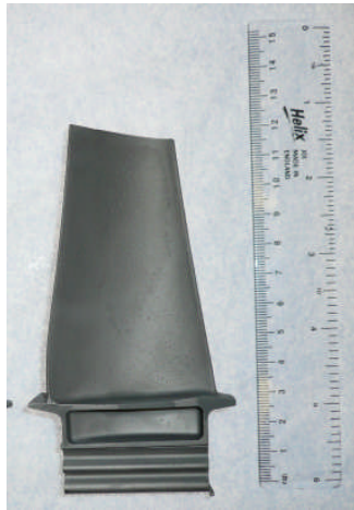
(a) Blade after SiAl CVD; before heat treatment
