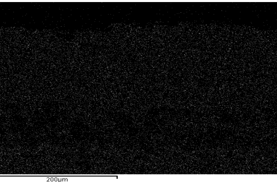
Figure 9.36: Oxidation test: 3000 hours at 1050°C, bottom side of IN738LC sample with 60mins CVD silicon-aluminide coating – element maps
