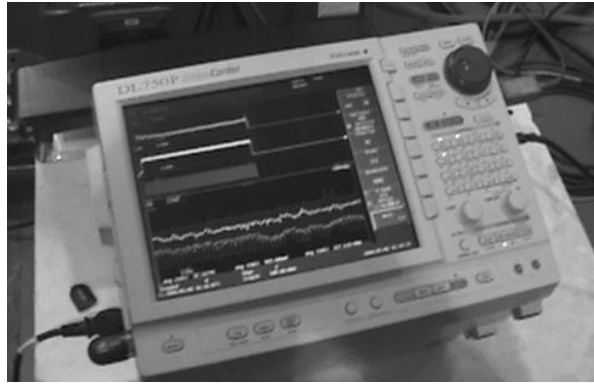
Figure 2.14 – Oscilloscope used for the current and voltage waveform and WFS signal recordings.
