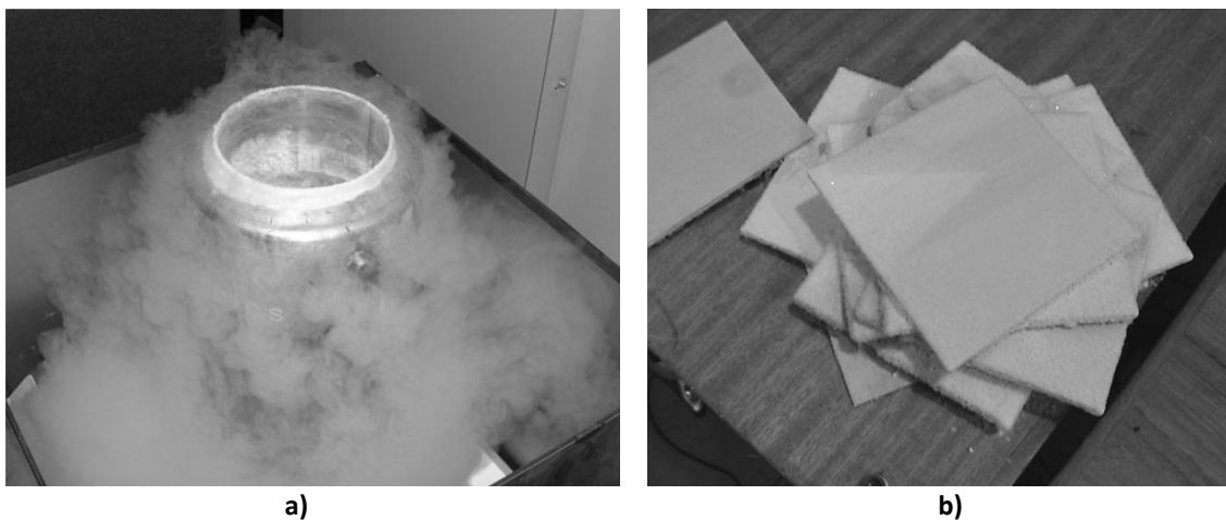
Figure 3.5 – Liquid nitrogen calorimetric tests: a) container during calorimetric test; b) specimens after calorimetric tests.
