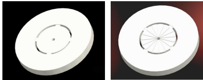
Figure 12-2 A CAD image showing how separation layers could be modified for higher efficiency
