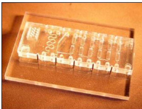
Figure 2-8 Two stacked chips aligned using elastic averaging with V-grooves and dowel pins [170]
