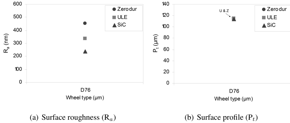
Figure 5.13: Surface responses for rough cuts - a_e = 500 \mu\text{m} , f_r = 15 \text{ mm/rev} , v_w = 25 \text{ mm/s} , Q_w = 187.5 \text{ mm}^3/\text{s}
