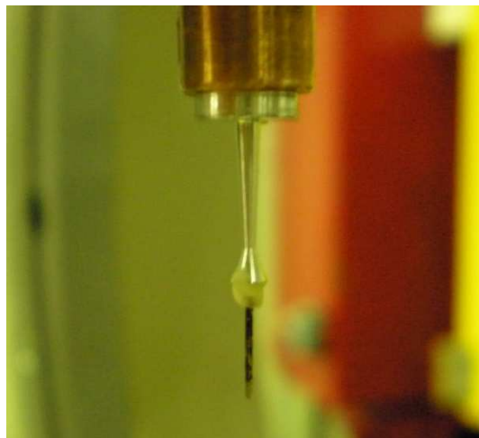
Figure 5.2: HoPtIn single crystal mounted on D9
