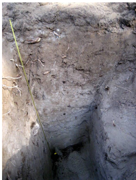
Plate 2.1: Section through mature forest soil; sampling location for CP07/22. Beneath humus-rich A-horizon a mottled carbonate-rich horizon is encountered. This is probably derived from the aeolianite parent material below. Test-pit is 1.2 m deep.
