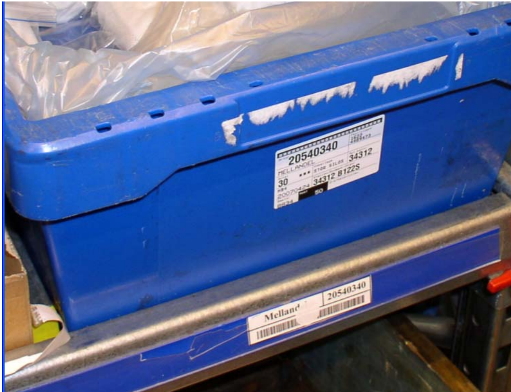
Figure 2.11: Example from a material shelf front. The part number is present on both the box containing the part and on the material shelf front itself.
