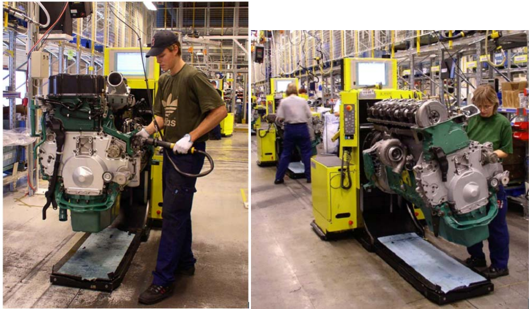
Figure 2.7: Example of one of the products, part of the information system (the computer screen on top of the carrier) and the carrier.
