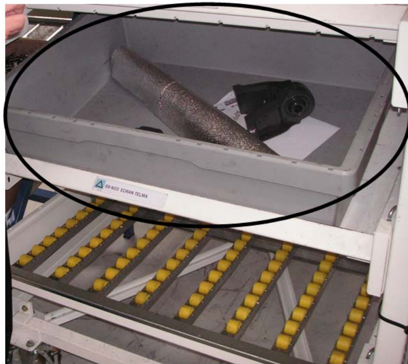
Figure 4.12: Kit presented at the assembly station. When the parts in the box are assembled the box is removed and a new box is presented to the assembler.
