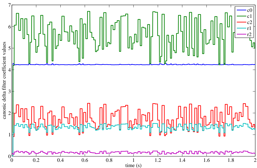
(b) The digital filter coefficient values change depending on the sample rate for the canonic \delta -filter
