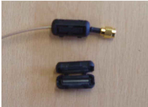
Figure 6-6: Ferrite chokes used on coaxial cables during on-body channel characterisation measurements.
