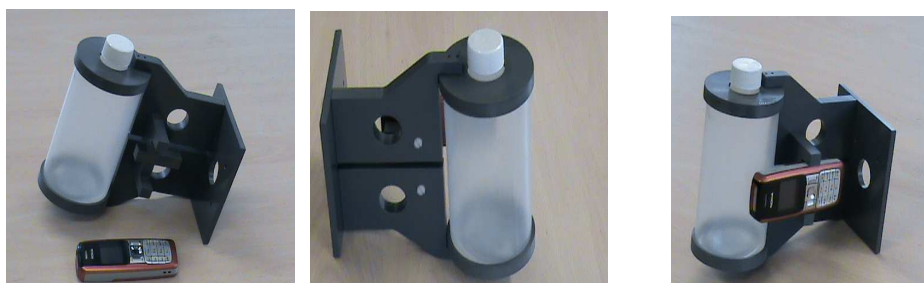
Figure 5-14: DUT and Phantom fixture
