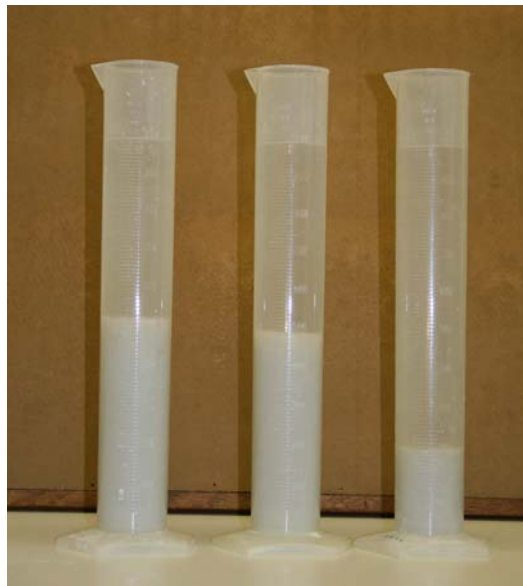
Figure 3.7: Photograph of suspensions settled in their measuring cylinders.
