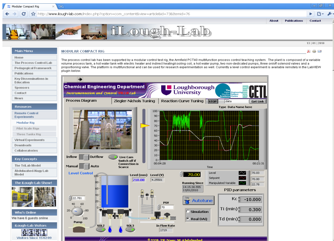
Figure 5.13. The Armfield modular rig operating remotely through an embedded VI inside the Joomla-based portal.
