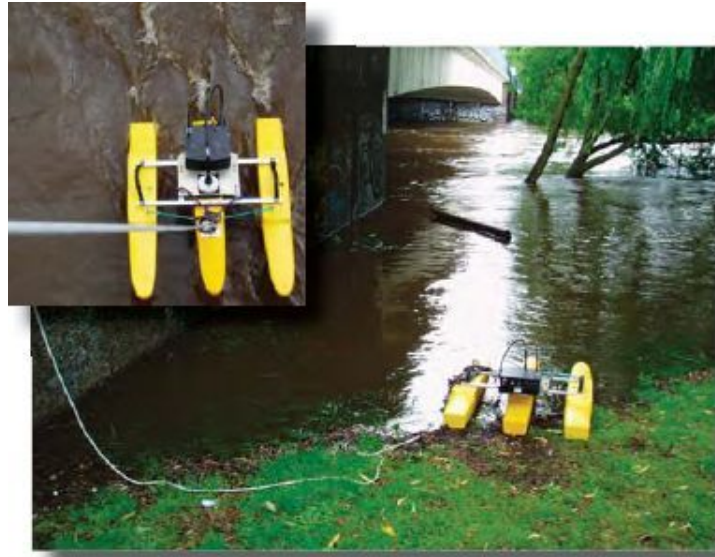
Figure 6.15: ADP used on the River Derwent at Derby Saint Mary's
