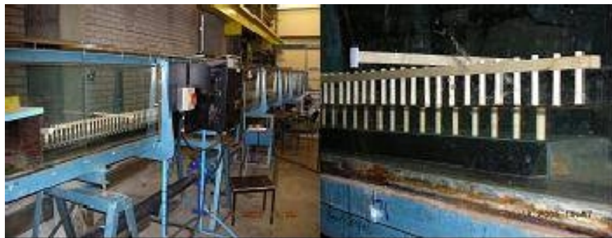
Figure 2.28: Experiments from Sun (2006) with 9 mm rods in the compound channel flume of Loughborough
