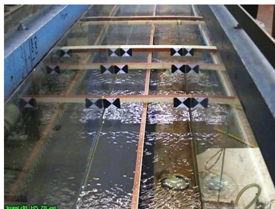
Figure 3.27: Example of LS-PIV set-up at Loughborough University
