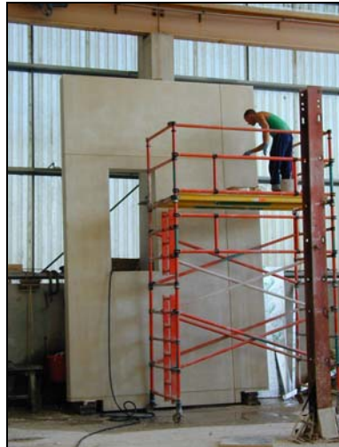
Figure 5.3 Offsite manufactured precast concrete cladding panel
