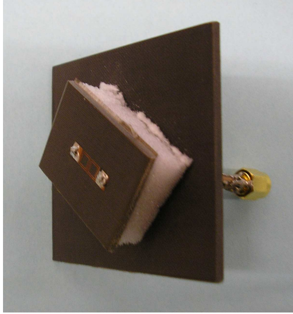
Figure 4.24: Photograph of the proposed \lambda/9 folded monopole built on a \lambda/2 \times \lambda/2 ground plane.
