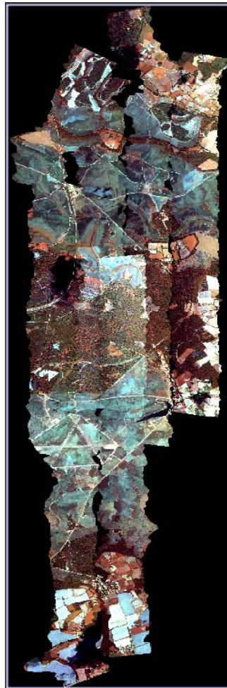
Figure 4.5. CASI-2 RGB mosaic comprised of seven geo-referenced flight scans that have been corrected for the effects of the atmosphere and radiometric variation.
